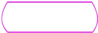
Fig. 1.8.5: Edge defect due to heavy reduction
