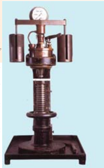
This Brinell hardness testing machine is used to test the hardness of the metal.
