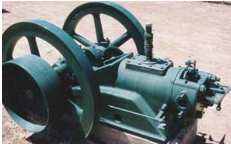
Flywheel of a pump run by a diesel engine.
