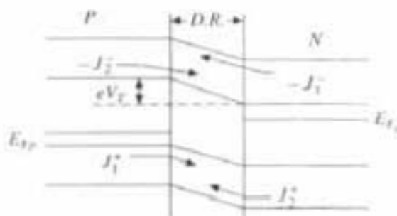
Fig. 6.19(a) Different current flows across forward bias P-N junction
