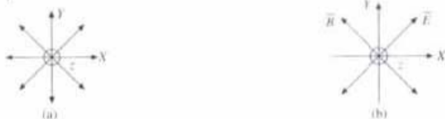
Fig. 1.28 (a) Unpolarised beam moving along Z-axis, when E -vector or M -vector continuously changing its direction in xy plane. (b) Linearly polarised light moving along z -axis, when E - or M -vector which are orthogonal to each other, oscillates only along a particular direction
