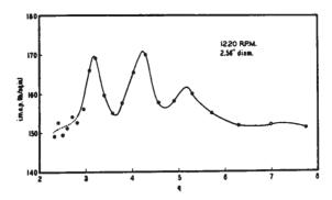
Figure 2.3.3: Experimental verification of the resonance of the n=3,4, and 5 harmonics of the Fourier representation (2.3.14) of the flow of an air-gas mixture with the intake pipe system. The parameter q is defined in the text. (From Morse, P., Boden, R. H., and Schecter, H., 1938: Acoustic vibrations and internal combustion engine performance. J. Appl. Phys., 9, 17 with permission.)
