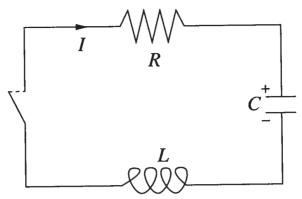
Figure 4.8.2: Schematic of a LCR circuit.
