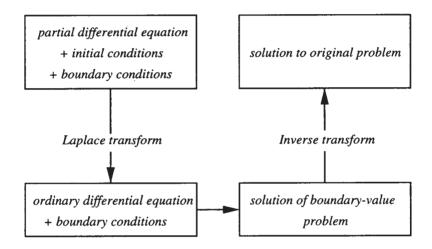
In the following examples, we will illustrate transform methods by solving the classic equation of telegraphy as it applies to a uniform transmission line. The line has a resistance R, an inductance L, a capacitance C, and a leakage conductance G per unit length. We denote the current in the direction of positive x by I; V is the voltage drop across the transmission line at the point x. The dependent variables I and V are functions of both distance x along the line and time t.
