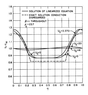
Figure 2.6.1: Temperature distribution along the equator of a spinning spherical satellite. (From Hrycak, P., 1963: Temperature distribution in a spinning spherical space vehicle. AIAA J., 1, 97. ©1963 AIAA, reprinted with permission.)
