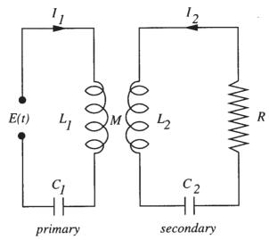
Figure 4.8.4: Schematic of a resonance transformer circuit.
