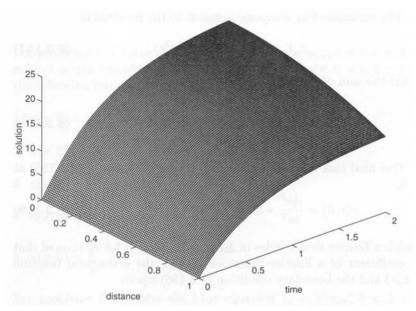
Figure 8.3.8: The temperature field (in degrees Celsius) within an electric copper cable containing 37 wires and a current of 22 amperes at various positions r/b and times  $a^2t/b^2$ . Initially the temperature was zero and then we allow the cable to cool radiatively as it is heated. The parameters are hb=1 and the radius of the cable b=4 cm.
