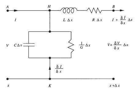
Figure 7.5.1: Schematic of an uniform transmission line.
