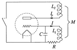
Figure 4.8.3: Schematic of a LCR circuit with the addition of a thermionic amplifier. [From Ballantine, S., 1919: The operational characteristics of thermionic amplifiers. *Proc. IRE*, 7, 155. ©IRE (now IEEE).]
