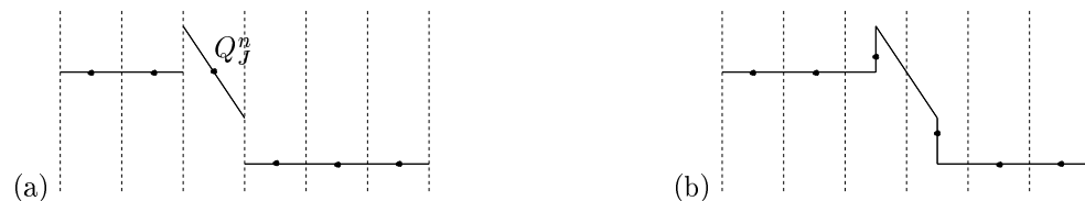
Figure 17.10: (a) Grid values Q^n and reconstructed \tilde{q}^n(\cdot, t_n) using Lax-Wendroff slopes. (b) After advection with ku = h/2 . The dots show the new cell averages Q^{n+1} . Note the overshoot
