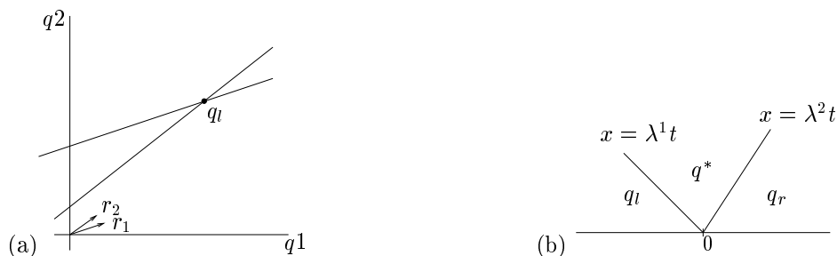
Figure 17.5: (a) The Hugoniot locus of the state q_l consists of all states that differ from q_l by a scalar multiple of r_1 or r_2 . (b) Solution to the Riemann problem in the x-t plane
