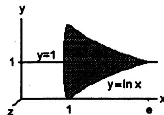
24. (a)  $V = \pi \int_0^1 [(e^y)^2 - 1] dy = \pi \int_0^1 (e^{2y} - 1) dy = \pi \left[ \frac{e^{2y}}{2} - y \right]_0^1 = \pi \left[ \frac{e^2}{2} - 1 - \left( \frac{1}{2} \right) \right] = \frac{\pi(e^2 - 3)}{2}$
