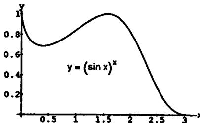
$$(b) \ln f(x) = x \ln(\sin x) = \frac{\ln(\sin x)}{\left(\frac{1}{x}\right)} \Rightarrow \lim_{x \rightarrow 0^+} \ln f(x) = \lim_{x \rightarrow 0^+} \frac{\ln(\sin x)}{\left(\frac{1}{x}\right)} = \lim_{x \rightarrow 0^+} \frac{\left(\frac{1}{\sin x}\right)(\cos x)}{\left(-\frac{1}{x^2}\right)}$$
