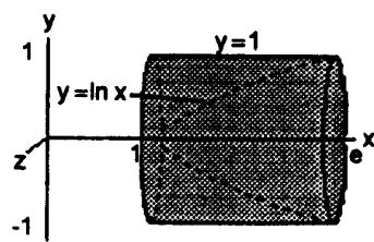
(b)  $V = \int_1^e \pi(1 - \ln x)^2 dx = \pi \int_1^e [1 - 2 \ln x + (\ln x)^2] dx$
