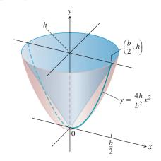
76. Suspension bridge cables hang in parabolas The suspension bridge cable shown here supports a uniform load of w pounds per horizontal foot. It can be shown that if H is the horizontal tension of the cable at the origin, then the curve of the cable satisfies the equation
