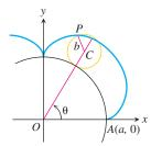
Let the radius of the rolling circle be b and let the initial position of the tracing point P be A(a, 0). Find parametric equations for the epicycloid, using as the parameter the angle  $\theta$  from the positive x-axis to the line through the circles' centers.
