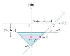
**2. Triangular plate** Calculate the fluid force on one side of the plate in Example 1 using the coordinate system shown here.
