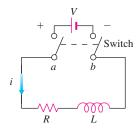
Use a phase line analysis to sketch the solution curve assuming that the switch in the *RL*-circuit is closed at time t=0. What happens to the current as  $t \to \infty$ ? This value is called the *steady-state solution*.
