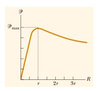
**Figure 28.3** Graph of the power  $\mathcal{P}$  delivered by a battery to a load resistor of resistance R as a function of R. The power delivered to the resistor is a maximum when the load resistance equals the internal resistance of the battery.
