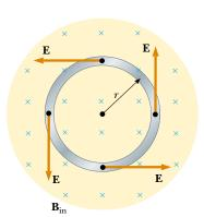
**Figure 31.17** A conducting loop of radius *r* in a uniform magnetic field perpendicular to the plane of the loop. If **B** changes in time, an electric field is induced in a direction tangent to the circumference of the loop.
