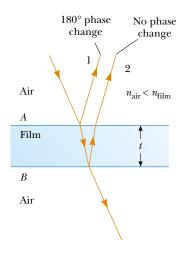
*Figure 37.16* Interference in light reflected from a thin film is due to a combination of rays reflected from the upper and lower surfaces of the film.
