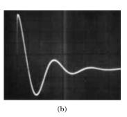
**Figure 32.21** (a) Charge versus time for a damped *RLC* circuit. The charge decays in this way when  $R \ll \sqrt{4L/C}$ . The *Q*-versus-t curve represents a plot of Equation 32.31. (b) Oscilloscope pattern showing the decay in the oscillations of an *RLC* circuit. The parameters used were  $R=75~\Omega, L=10~\text{mH}$ , and  $C=0.19~\mu\text{F}$ .
