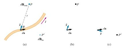
**Figure 30.1** (a) The magnetic field  $d\mathbf{B}$  at point P due to the current I through a length element  $d\mathbf{s}$  is given by the Biot–Savart law. The direction of the field is out of the page at P and into the page at P'. (b) The cross product  $d\mathbf{s} \times \hat{\mathbf{r}}$  points out of the page when  $\hat{\mathbf{r}}$  points toward P. (c) The cross product  $d\mathbf{s} \times \hat{\mathbf{r}}$  points into the page when  $\hat{\mathbf{r}}$  points toward P'.
