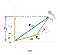
**Figure 37.7** (a) Phasor diagram for the wave disturbance  $E_1 = E_0 \sin \omega t$ . The phasor is a vector of length  $E_0$  rotating counterclockwise. (b) Phasor diagram for the wave  $E_2 = E_0 \sin(\omega t + \phi)$ . (c) The disturbance  $\mathbf{E}_R$  is the resultant phasor formed from the phasors of parts (a) and (b).
