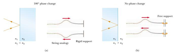
**Figure 37.15** (a) For  $n_1 < n_2$ , a light ray traveling in medium 1 when reflected from the surface of medium 2 undergoes a 180° phase change. The same thing happens with a reflected pulse traveling along a string fixed at one end. (b) For  $n_1 > n_2$ , a light ray traveling in medium 1 undergoes no phase change when reflected from the surface of medium 2. The same is true of a reflected wave pulse on a string whose supported end is free to move.
