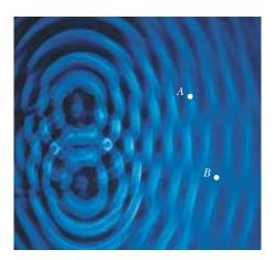
**Figure 37.2** An interference pattern involving water waves is produced by two vibrating sources at the water's surface. The pattern is analogous to that observed in Young's double-slit experiment. Note the regions of constructive (*A*) and destructive (*B*) interference.
