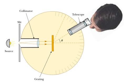
**Figure 38.21** Diagram of a diffraction grating spectrometer. The collimated beam incident on the grating is diffracted into the various orders at the angles  $\theta$  that satisfy the equation  $d \sin \theta = m\lambda$ , where  $m = 0, 1, 2, \ldots$ .
