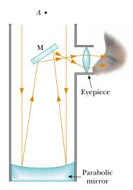
**Figure 36.43** A Newtonian-focus reflecting telescope.
