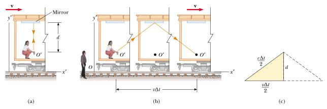
**Figure 39.8** (a) A mirror is fixed to a moving vehicle, and a light pulse is sent out by observer O' at rest in the vehicle. (b) Relative to a stationary observer O standing alongside the vehicle, the mirror and O' move with a speed v. Note that what observer O measures for the distance the pulse travels is greater than 2d. (c) The right triangle for calculating the relationship between  $\Delta t$  and  $\Delta t_p$ .
