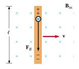
**Figure 31.8** A straight electrical conductor of length  $\ell$  moving with a velocity  $\mathbf{v}$  through a uniform magnetic field  $\mathbf{B}$  directed perpendicular to  $\mathbf{v}$ . A potential difference  $\Delta V = B\ell v$  is maintained between the ends of the conductor.
