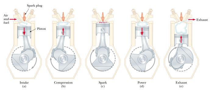
**Figure 22.11** The four-stroke cycle of a conventional gasoline engine. (a) In the intake stroke, air is mixed with fuel. (b) The intake valve is then closed, and the air-fuel mixture is compressed by the piston. (c) The mixture is ignited by the spark plug, with the result that the temperature of the mixture increases. (d) In the power stroke, the gas expands against the piston. (e) Finally, the residual gases are expelled, and the cycle repeats.
