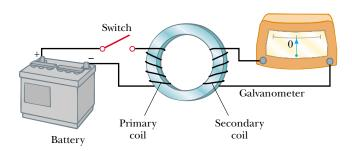
**Figure 31.2** Faraday's experiment. When the switch in the primary circuit is closed, the galvanometer in the secondary circuit deflects momentarily. The emf induced in the secondary circuit is caused by the changing magnetic field through the secondary coil.
