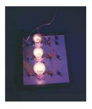
Three lightbulbs having power ratings of 25 W, 75 W, and 150 W, connected in parallel to a voltage source of about 100 V. All bulbs are rated at the same voltage. Why do the intensities differ? Which bulb draws the most current? Which has the least resistance?
