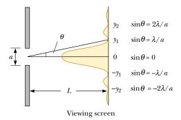
**Figure 38.6** Intensity distribution for a Fraunhofer diffraction pattern from a single slit of width *a*. The positions of two minima on each side of the central maximum are labeled (drawing not to scale).
