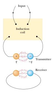
**Figure 34.1** Schematic diagram of Hertz's apparatus for generating and detecting electromagnetic waves. The transmitter consists of two spherical electrodes connected to an induction coil, which provides short voltage surges to the spheres, setting up oscillations in the discharge between the electrodes (suggested by the red dots). The receiver is a nearby loop of wire containing a second spark gap.
