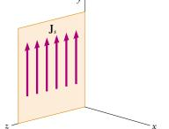
**Figure 34.10** A portion of an infinite current sheet lying in the yz plane. The current density is sinusoidal and is given by the expression  $J_s = J_{\text{max}} \cos \omega t$ . The magnetic field is everywhere parallel to the sheet and lies along z.
