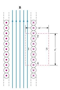
**Figure 30.18** Cross-sectional view of an ideal solenoid, where the interior magnetic field is uniform and the exterior field is zero. Ampère's law applied to the red dashed path can be used to calculate the magnitude of the interior field.
