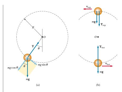
**Figure 6.11** (a) Forces acting on a sphere of mass *m* connected to a cord of length *R* and rotating in a vertical circle centered at *O*. (b) Forces acting on the sphere at the top and bottom of the circle. The tension is a maximum at the bottom and a minimum at the top.
