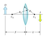
**Figure 36.23** Simplified geometry for a thin lens.
