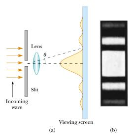
**Figure 38.4** (a) Fraunhofer diffraction pattern of a single slit. The pattern consists of a central bright fringe flanked by much weaker maxima alternating with dark fringes (drawing not to scale). (b) Photograph of a single-slit Fraunhofer diffraction pattern.
