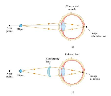
**Figure 36.36** (a) When a farsighted eye looks at an object located between the near point and the eye, the image point is behind the retina, resulting in blurred vision. The eye muscle contracts to try to bring the object into focus. (b) Farsightedness is corrected with a converging lens.
