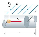
**Figure 29.7** A segment of a current-carrying wire located in a magnetic field **B**. The magnetic force exerted on each charge making up the current is  $q\mathbf{v}_d \times \mathbf{B}$ , and the net force on the segment of length L is  $I\mathbf{L} \times \mathbf{B}$ .
