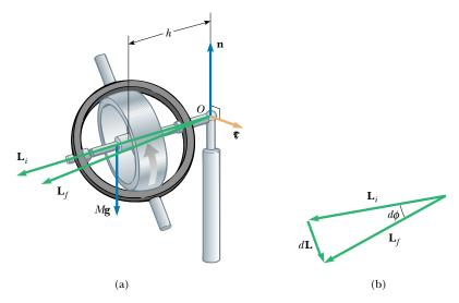
**Figure 11.20** (a) The motion of a simple gyroscope pivoted a distance h from its center of mass. The force of gravity  $M\mathbf{g}$  produces a torque about the pivot, and this torque is perpendicular to the axle. (b) This torque results in a change in angular momentum  $d\mathbf{L}$  in a direction perpendicular to the axle. The axle sweeps out an angle  $d\phi$  in a time dt.
