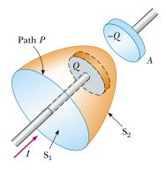
Figure 30.24 Two surfaces S<sub>1</sub> and S<sub>2</sub> near the plate of a capacitor are bounded by the same path P. The conduction current in the wire passes only through  $S_1$ . This leads to a contradiction in Ampère's law that is resolved only if one postulates a displacement current through  $S_2$ .
