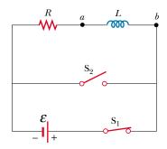
**Figure 32.6** An RL circuit containing two switches. When  $S_1$  is closed and  $S_2$  open as shown, the battery is in the circuit. At the instant  $S_2$  is closed,  $S_1$  is opened, and the battery is no longer part of the circuit.
