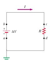
**Figure 27.14** A circuit consisting of a resistor of resistance R and a battery having a potential difference  $\Delta V$  across its terminals. Positive charge flows in the clockwise direction. Points a and d are grounded.
