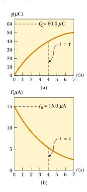
**Figure 28.20** Plots of (a) charge versus time and (b) current versus time for the *RC* circuit shown in Figure 28.19, with  $\mathcal{E} = 12.0 \text{ V}$ ,  $R = 8.00 \times 10^5 \Omega$ , and  $C = 5.00 \mu\text{F}$ .
