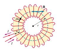
**Figure 30.13** A toroid consisting of many turns of wire. If the turns are closely spaced, the magnetic field in the interior of the torus (the gold-shaded region) is tangent to the dashed circle and varies as 1/r. The field outside the toroid is zero. The dimension a is the cross-sectional radius of the torus.
