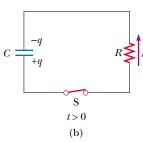
**Figure 28.18** (a) A charged capacitor connected to a resistor and a switch, which is open at t < 0. (b) After the switch is closed, a current that decreases in magnitude with time is set up in the direction shown, and the charge on the capacitor decreases exponentially with time.
