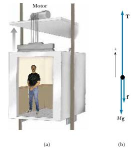
**Figure 7.18** (a) The motor exerts an upward force  $\mathbf{T}$  on the elevator car. The magnitude of this force is the tension T in the cable connecting the car and motor. The downward forces acting on the car are a frictional force  $\mathbf{f}$  and the force of gravity  $\mathbf{F}_g = M\mathbf{g}$ . (b) The free-body diagram for the elevator car.
