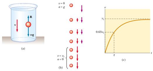
**Figure 6.15** (a) A small sphere falling through a liquid. (b) Motion diagram of the sphere as it falls. (c) Speed–time graph for the sphere. The sphere reaches a maximum, or terminal, speed  $v_t$ , and the time constant  $\tau$  is the time it takes to reach  $0.63v_t$ .
