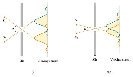
**Figure 38.12** Two point sources far from a narrow slit each produce a diffraction pattern. (a) The angle subtended by the sources at the slit is large enough for the diffraction patterns to be distinguishable. (b) The angle subtended by the sources is so small that their diffraction patterns overlap, and the images are not well resolved. (Note that the angles are greatly exaggerated. The drawing is not to scale.)
