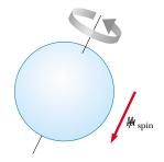
**Figure 30.27** Classical model of a spinning electron. This model gives an incorrect magnitude for the magnetic moment, incorrect quantum numbers, and too many degrees of freedom.
