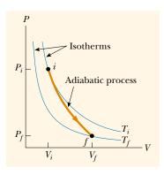
**Figure 21.5** The *PV* diagram for an adiabatic expansion. Note that  $T_f < T_i$  in this process.
