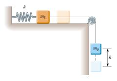
**Figure 8.13** As the hanging block moves from its highest elevation to its lowest, the system loses gravitational potential energy but gains elastic potential energy in the spring. Some mechanical energy is lost because of friction between the sliding block and the surface.
