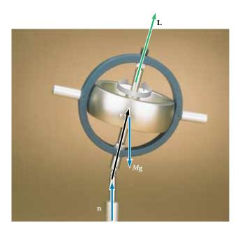
This toy gyroscope undergoes precessional motion about the vertical axis as it spins about its axis of symmetry. The only forces acting on it are the force of gravity  $M\mathbf{g}$  and the upward force of the pivot  $\mathbf{n}$ . The direction of its angular momentum  $\mathbf{L}$  is along the axis of symmetry. The torque and  $\Delta \mathbf{L}$  are directed into the page. (Courtesy of Central Scientific Company)
