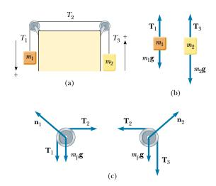
**Figure 10.21** (a) Another look at Atwood's machine. (b) Free-body diagrams for the blocks. (c) Free-body diagrams for the pulleys, where  $m_{\rm p}{\bf g}$  represents the force of gravity acting on each pulley.
