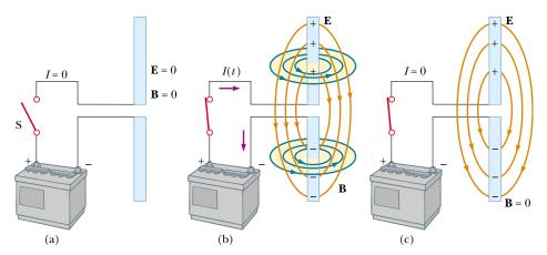
**Figure 34.13** A pair of metal rods connected to a battery. (a) When the switch is open and no current exists, the electric and magnetic fields are both zero. (b) Immediately after the switch is closed, the rods are being charged (so a current exists). Because the current is changing, the rods generate changing electric and magnetic fields. (c) When the rods are fully charged, the current is zero, the electric field is a maximum, and the magnetic field is zero.
