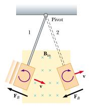
**Figure 31.23** As the conducting plate enters the field (position 1), the eddy currents are counterclockwise. As the plate leaves the field (position 2), the currents are clockwise. In either case, the force on the plate is opposite the velocity, and eventually the plate comes to rest.
