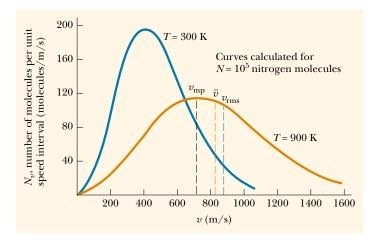
**Figure 21.12** The speed distribution function for  $10^5$  nitrogen molecules at 300 K and 900 K. The total area under either curve is equal to the total number of molecules, which in this case equals  $10^5$ . Note that  $v_{\rm rms} > \overline{v} > v_{\rm mp}$ .
