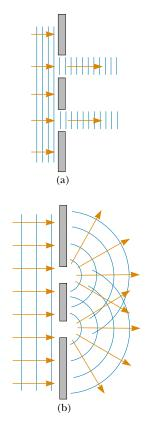
Figure 38.1 (a) If light waves did not spread out after passing through the slits, no interference would occur. (b) The light waves from the two slits overlap as they spread out, filling what we expect to be shadowed regions with light and producing interference fringes.
