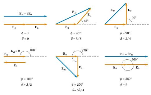
**Figure 37.10** Phasor diagrams for a double-slit interference pattern. The resultant phasor  $\mathbf{E}_R$  is a maximum when  $\phi = 0, 2\pi, 4\pi, \ldots$  and is zero when  $\phi = \pi, 3\pi, 5\pi, \ldots$
