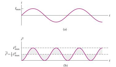
**Figure 33.3** (a) Graph of the current in a resistor as a function of time. (b) Graph of the current squared in a resistor as a function of time. Notice that the gray shaded regions *under* the curve and *above* the dashed line for  $I_{\rm max}^2/2$  have the same area as the gray shaded regions *above* the curve and *below* the dashed line for  $I_{\rm max}^2/2$ . Thus, the average value of  $i^2$  is  $I_{\rm max}^2/2$ .
