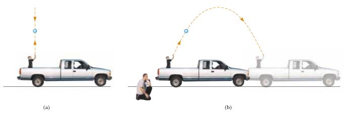
*Figure 39.1* (a) The observer in the truck sees the ball move in a vertical path when thrown upward. (b) The Earth observer sees the path of the ball as a parabola.
