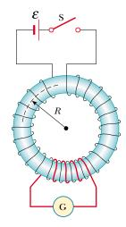
**Figure 30.29** A toroidal winding arrangement used to measure the magnetic properties of a material. The torus is made of the material under study, and the circuit containing the galvanometer measures the magnetic flux.
