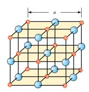
**Figure 38.24** Crystalline structure of sodium chloride (NaCl). The blue spheres represent Cl<sup>-</sup>ions, and the red spheres represent Na<sup>+</sup>ions. The length of the cube edge is a = 0.562737 nm.
