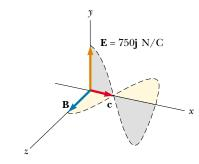
**Figure 34.4** At some instant, a plane electromagnetic wave moving in the x direction has a maximum electric field of 750 N/C in the positive y direction. The corresponding magnetic field at that point has a magnitude E/c and is in the z direction.
