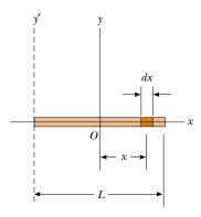
**Figure 10.10** A uniform rigid rod of length L. The moment of inertia about the y axis is less than that about the y' axis. The latter axis is examined in Example 10.8.
