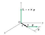
**Figure 11.10** The angular momentum  $\mathbf{L}$  of a particle of mass m and linear momentum  $\mathbf{p}$  located at the vector position  $\mathbf{r}$  is a vector given by  $\mathbf{L} = \mathbf{r} \times \mathbf{p}$ . The value of  $\mathbf{L}$  depends on the origin about which it is measured and is a vector perpendicular to both  $\mathbf{r}$  and  $\mathbf{p}$ .
