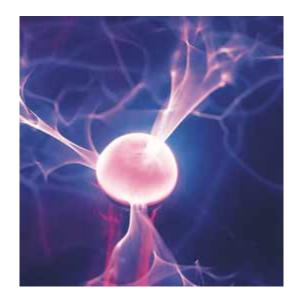
This metallic sphere is charged by a generator so that it carries a net electric charge. The high concentration of charge on the sphere creates a strong electric field around the sphere. The charges then leak through the gas surrounding the sphere, producing a pink glow.
