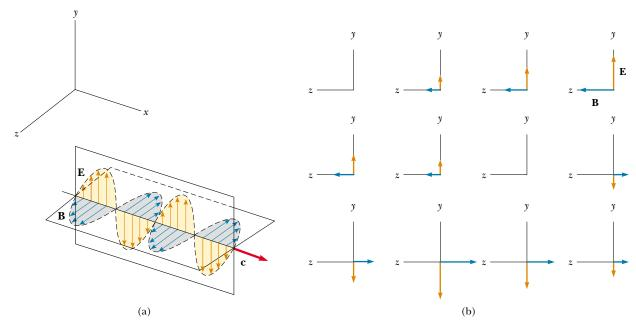
**Figure 34.3** Representation of a sinusoidal, linearly polarized plane electromagnetic wave moving in the positive x direction with velocity  $\mathbf{c}$ . (a) The wave at some instant. Note the sinusoidal variations of E and B with x. (b) A time sequence illustrating the electric and magnetic field vectors present in the yz plane, as seen by an observer looking in the negative x direction. Note the sinusoidal variations of E and B with t.
