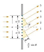
**Figure 38.5** Diffraction of light by a narrow slit of width a. Each portion of the slit acts as a point source of light waves. The path difference between rays 1 and 3 or between rays 2 and 4 is  $(a/2)\sin\theta$  (drawing not to scale).
