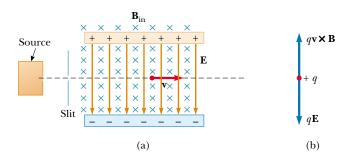
**Figure 29.22** (a) A velocity selector. When a positively charged particle is in the presence of a magnetic field directed into the page and an electric field directed downward, it experiences a downward electric force  $q\mathbf{E}$  and an upward magnetic force  $q\mathbf{v} \times \mathbf{B}$ . (b) When these forces balance, the particle moves in a horizontal line through the fields.
