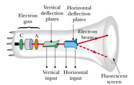
**Figure 23.26** Schematic diagram of a cathode ray tube. Electrons leaving the hot cathode C are accelerated to the anode A. In addition to accelerating electrons, the electron gun is also used to focus the beam of electrons, and the plates deflect the beam.
