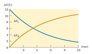
**Figure 32.10** The sum of the potential differences across the resistor and inductor in Figure 32.9a is 12.0 V (the battery emf) at all times.
