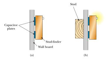
**Figure 26.16** A stud-finder. (a) The materials between the plates of the capacitor are the wall-board and air. (b) When the capacitor moves across a stud in the wall, the materials between the plates are the wallboard and the wood. The change in the dielectric constant causes a signal light to illuminate.
