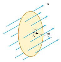
**Figure 31.3** A conducting loop that encloses an area A in the presence of a uniform magnetic field **B**. The angle between **B** and the normal to the loop is  $\theta$ .
