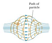
Figure 29.20 A charged particle moving in a nonuniform magnetic field (a magnetic bottle) spirals about the field (red path) and oscillates between the end points. The magnetic force exerted on the particle near either end of the bottle has a component that causes the particle to spiral back toward the center.
