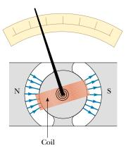
**Figure 29.16** End view of a moving-coil galvanometer.
