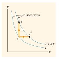
**Figure 21.4** Energy is transferred by heat to an ideal gas in two ways. For the constant-volume path  $i \rightarrow f$ , all the energy goes into increasing the internal energy of the gas because no work is done. Along the constant-pressure path  $i \rightarrow f'$ , part of the energy transferred in by heat is transferred out by work done by the gas.
