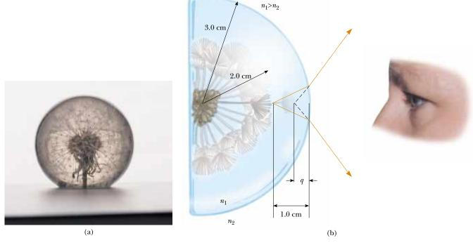
**Figure 36.20** (a) An object embedded in a plastic sphere forms a virtual image between the surface of the object and the sphere surface. All rays are assumed paraxial. Because the object is inside the sphere, the front of the refracting surface is the *interior* of the sphere. (b) Rays from the surface of the object form an image that is still inside the plastic sphere but closer to the plastic surface.
