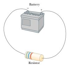
**Figure 28.1** A circuit consisting of a resistor connected to the terminals of a battery.
