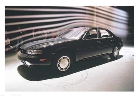
Figure 15.14 Laminar flow around an automobile in a test wind tunnel.
