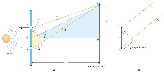
**Figure 37.4** (a) Geometric construction for describing Young's double-slit experiment (not to scale). (b) When we assume that  $r_1$  is parallel to  $r_2$ , the path difference between the two rays is  $r_2 - r_1 = d \sin \theta$ . For this approximation to be valid, it is essential that  $L \gg d$ .
