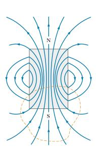
Figure 30.22 The magnetic field lines of a bar magnet form closed loops. Note that the net magnetic flux through the closed surface (dashed red line) surrounding one of the poles (or any other closed surface) is zero.
