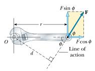
Figure 10.13 The force F has a greater rotating tendency about Oas Fincreases and as the moment arm d increases. It is the component  $F\sin\phi$  that tends to rotate the wrench about O.
