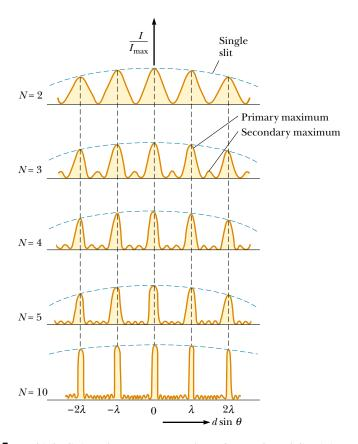
**Figure 37.13** Multiple-slit interference patterns. As *N*, the number of slits, is increased, the primary maxima (the tallest peaks in each graph) become narrower but remain fixed in position, and the number of secondary maxima increases. For any value of *N*, the decrease in intensity in maxima to the left and right of the central maximum, indicated by the blue dashed arcs, is due to diffraction, which is discussed in Chapter 38.
