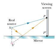
**Figure 37.14** Lloyd's mirror. An interference pattern is produced at point P on the screen as a result of the combination of the direct ray (blue) and the reflected ray (red). The reflected ray undergoes a phase change of  $180^{\circ}$ .
