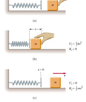
**Figure 8.2** (a) An undeformed spring on a frictionless horizontal surface. (b) A block of mass m is pushed against the spring, compressing it a distance x. (c) When the block is released from rest, the elastic potential energy stored in the spring is transferred to the block in the form of kinetic energy.
