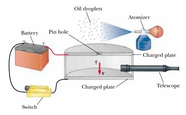
Figure 25.25 Schematic drawing of the Millikan oil-drop apparatus.
