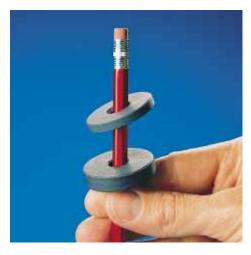
Figure Q30.33 Magnetic levitation using two ceramic magnets.
