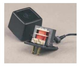
**Figure 33.20** The primary winding in this transformer is directly attached to the prongs of the plug. The secondary winding is connected to the wire on the right, which runs to an electronic device. Many of these power-supply transformers also convert alternating current to direct current. (*George Semble*)
