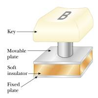
**Figure 26.4** One type of computer keyboard button.
