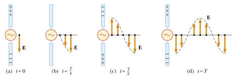
**Figure 34.12** The electric field set up by charges oscillating in an antenna. The field moves away from the antenna with the speed of light.
