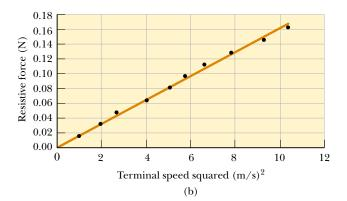
**Figure 6.17** (a) Relationship between the resistive force acting on falling coffee filters and their terminal speed. The curved line is a second-order polynomial fit. (b) Graph relating the resistive force to the square of the terminal speed. The fit of the straight line to the data points indicates that the resistive force is proportional to the terminal speed squared. Can you find the proportionality constant?
