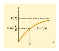
**Figure 32.4** Plot of the current versus time for the RL circuit shown in Figure 32.3. The switch is thrown closed at t=0, and the current increases toward its maximum value  $\mathcal{E}/R$ . The time constant  $\tau$  is the time it takes I to reach 63% of its maximum value.
