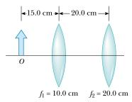
*Figure 36.29* A combination of two converging lenses.
