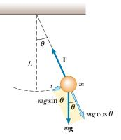
**Figure 13.12** When  $\theta$  is small, a simple pendulum oscillates in simple harmonic motion about the equilibrium position  $\theta = 0$ . The restoring force is  $mg \sin \theta$ , the component of the gravitational force tangent to the arc.
