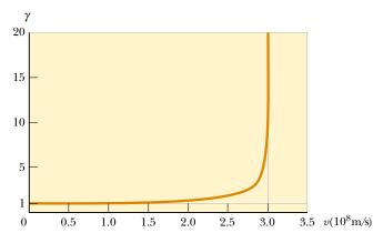
**Figure 39.9** Graph of  $\gamma$  versus v. As the velocity approaches the speed of light,  $\gamma$  increases rapidly.
