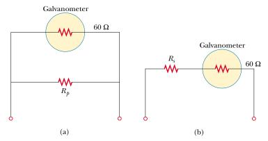
**Figure 28.24** (a) When a galvanometer is to be used as an ammeter, a shunt resistor  $R_p$  is connected in parallel with the galvanometer. (b) When the galvanometer is used as a voltmeter, a resistor  $R_s$  is connected in series with the galvanometer.
