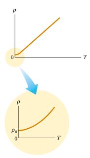
**Figure 27.10** Resistivity versus temperature for a metal such as copper. The curve is linear over a wide range of temperatures, and  $\rho$  increases with increasing temperature. As T approaches absolute zero (inset), the resistivity approaches a finite value  $\rho_0$ .
