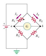
**Figure 28.25** Circuit diagram for a Wheatstone bridge, an instrument used to measure an unknown resistance  $R_x$  in terms of known resistances  $R_1$ ,  $R_2$ , and  $R_3$ . When the bridge is balanced, no current is present in the galvanometer. The arrow superimposed on the circuit symbol for resistor  $R_1$  indicates that the value of this resistor can be varied by the person operating the bridge.
