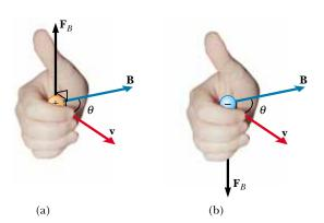
**Figure 29.4** The right-hand rule for determining the direction of the magnetic force  $\mathbf{F}_B = q\mathbf{v} \times \mathbf{B}$  acting on a particle with charge q moving with a velocity  $\mathbf{v}$  in a magnetic field  $\mathbf{B}$ . The direction of  $\mathbf{v} \times \mathbf{B}$  is the direction in which the thumb points. (a) If q is positive,  $\mathbf{F}_B$  is upward. (b) If q is negative,  $\mathbf{F}_B$  is downward, antiparallel to the direction in which the thumb points.
