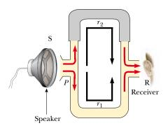
**Figure 18.2** An acoustical system for demonstrating interference of sound waves. A sound wave from the speaker (S) propagates into the tube and splits into two parts at point P. The two waves, which superimpose at the opposite side, are detected at the receiver (R). The upper path length  $r_2$  can be varied by sliding the upper section.
