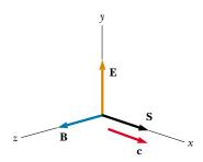
**Figure 34.7** The Poynting vector **S** for a plane electromagnetic wave is along the direction of wave propagation.
