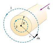
**Figure 30.11** A long, straight wire of radius R carrying a steady current  $I_0$  uniformly distributed across the cross-section of the wire. The magnetic field at any point can be calculated from Ampère's law using a circular path of radius r, concentric with the wire.
