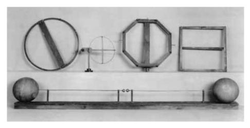
A large oscillator (bottom) and circular, octagonal, and square receivers used by Heinrich Hertz.
