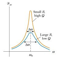
**Figure 33.16** Average power versus frequency for a series RLC circuit. The width  $\Delta \omega$  of each curve is measured between the two points where the power is half its maximum value. The power is a maximum at the resonance frequency  $\omega_0$ .
