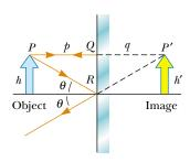
**Figure 36.2** A geometric construction that is used to locate the image of an object placed in front of a flat mirror. Because the triangles PQR and P'QR are congruent, |p| = |q| and h = h'.
