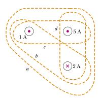
**Figure 30.9** Four closed paths around three current-carrying wires.
