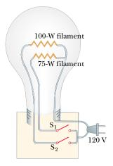
Figure 28.9 A three-way lightbulb.
