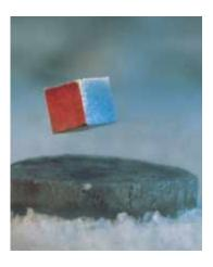
A small permanent magnet levitated above a disk of the superconductor  $YBa_2Cu_3O_7$ , which is at 77 K.
