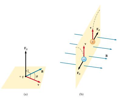
**Figure 29.3** The direction of the magnetic force  $\mathbf{F}_B$  acting on a charged particle moving with a velocity  $\mathbf{v}$  in the presence of a magnetic field  $\mathbf{B}$ . (a) The magnetic force is perpendicular to both  $\mathbf{v}$  and  $\mathbf{B}$ . (b) Oppositely directed magnetic forces  $\mathbf{F}_B$  are exerted on two oppositely charged particles moving at the same velocity in a magnetic field.
