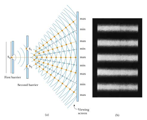
**Figure 37.1** (a) Schematic diagram of Young's double-slit experiment. Slits  $S_1$  and  $S_2$  behave as coherent sources of light waves that produce an interference pattern on the viewing screen (drawing not to scale). (b) An enlargement of the center of a fringe pattern formed on the viewing screen with many slits could look like this.
