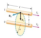
**Figure 30.7** Two parallel wires that each carry a steady current exert a force on each other. The field  $\mathbf{B}_2$  due to the current in wire 2 exerts a force of magnitude  $F_1 = I_1 \ell B_2$  on wire 1. The force is attractive if the currents are parallel (as shown) and repulsive if the currents are antiparallel.
