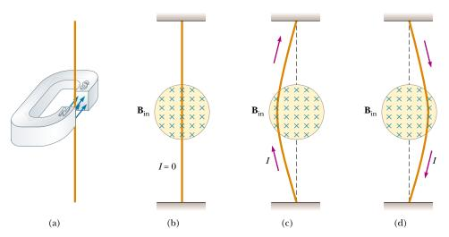
**Figure 29.6** (a) A wire suspended vertically between the poles of a magnet. (b) The setup shown in part (a) as seen looking at the south pole of the magnet, so that the magnetic field (blue crosses) is directed into the page. When there is no current in the wire, it remains vertical. (c) When the current is upward, the wire deflects to the left. (d) When the current is downward, the wire deflects to the right.
