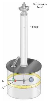
**Figure 23.5** Coulomb's torsion balance, used to establish the inverse-square law for the electric force between two charges.
