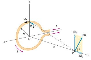
**Figure 30.5** Geometry for calculating the magnetic field at a point *P* lying on the axis of a current loop. By symmetry, the total field **B** is along this axis.
