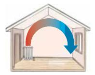
**Figure 20.13** Convection currents are set up in a room heated by a radiator.
