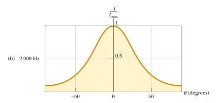
**Figure 38.17** Angular dispersion of sound intensity I for a midrange speaker at (a) 500 Hz and (b) 2 000 Hz.
