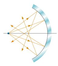
**Figure 36.10** Rays diverging from the object at large angles from the principal axis reflect from a spherical concave mirror to intersect the principal axis at different points, resulting in a blurred image. This condition is called *spherical aberration*.
