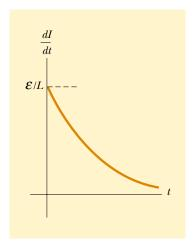
**Figure 32.5** Plot of dI/dt versus time for the RL circuit shown in Figure 32.3. The time rate of change of current is a maximum at t=0, which is the instant at which the switch is thrown closed. The rate decreases exponentially with time as I increases toward its maximum value.
