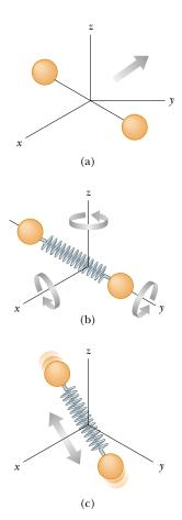
**Figure 21.6** Possible motions of a diatomic molecule: (a) translational motion of the center of mass, (b) rotational motion about the various axes, and (c) vibrational motion along the molecular axis.
