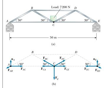
**Figure 12.12** (a) Truss structure for a bridge. (b) The forces acting on the pins at points A, C, and E. As an exercise, you should diagram the forces acting on the pin at point B.
