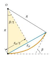
**Figure 38.9** Phasor diagram for a large number of coherent sources. All the ends of the phasors lie on the circular red arc of radius R. The resultant electric field magnitude  $E_R$  equals the length of the chord.
