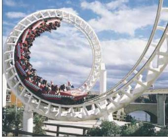
Some examples of forces acting during circular motion. (*Left*) As these speed skaters round a curve, the force exerted by the ice on their skates provides the centripetal acceleration. (*Right*) Passengers on a "corkscrew" roller coaster. What are the origins of the forces in this example?
