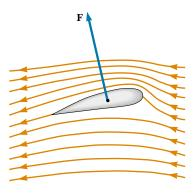
**Figure 15.24** Streamline flow around an airplane wing. The pressure above the wing is less than the pressure below, and a dynamic lift upward results.
