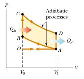
Figure 22.12 PV diagram for the Otto cycle, which approximately represents the processes occurring
