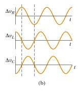
**Figure 33.9** (a) A series circuit consisting of a resistor, an inductor, and a capacitor connected to an ac generator. (b) Phase relationships for instantaneous voltages in the series *RLC* circuit.
