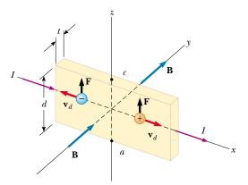
**Figure 29.27** To observe the Hall effect, a magnetic field is applied to a current-carrying conductor. When I is in the x direction and  $\mathbf{B}$  in the y direction, both positive and negative charge carriers are deflected upward in the magnetic field. The Hall voltage is measured between points a and c.
