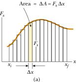
**Figure 7.7** (a) The work done by the force component  $F_x$  for the small displacement  $\Delta x$  is  $F_x \Delta x$ , which equals the area of the shaded rectangle. The total work done for the displacement from  $x_i$  to  $x_f$  is approximately equal to the sum of the areas of all the rectangles. (b) The work done by the component  $F_x$  of the varying force as the particle moves from  $x_i$  to  $x_f$  is exactly equal to the area under this curve.
