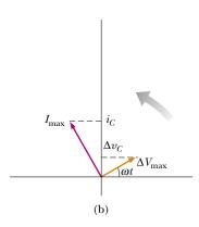
**Figure 33.8** (a) Plots of the instantaneous current  $i_C$  and instantaneous voltage  $\Delta v_C$  across a capacitor as functions of time. The voltage lags behind the current by 90°. (b) Phasor diagram for the capacitive circuit, showing that the current leads the voltage by 90°.
