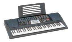
This synthesizer can produce the characteristic sounds of different instruments by properly combining frequencies from electronic oscillators.
