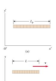
**Figure 39.13** (a) A stick measured by an observer in a frame attached to the stick (that is, both have the same velocity) has its proper length  $L_p$ . (b) The stick measured by an observer in a frame in which the stick has a velocity  ${\bf v}$  relative to the frame is shorter than its proper length  $L_p$  by a factor  $(1-v^2/c^2)^{1/2}$ .
