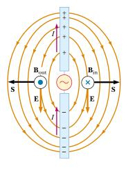
**Figure 34.14** A half-wave antenna consists of two metal rods connected to an alternating voltage source. This diagram shows **E** and **B** at an instant when the current is upward. Note that the electric field lines resemble those of a dipole (shown in Fig. 23.21).
