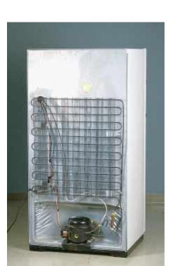
Figure 22.14 The coils on the back of a refrigerator transfer energy by heat to the air. The second law of thermodynamics states that this amount of energy must be greater than the amount of energy removed from the contents of the refrigerator (or from the air in the kitchen, if the refrigerator door is left open).
