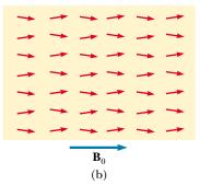
Figure 30.28 (a) Random orientation of atomic magnetic moments in an unmagnetized substance. (b) When an external field **B**<sub>0</sub> is applied, the atomic magnetic moments tend to align with the field, giving the sample a net magnetization vector **M**.
