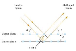
**Figure 38.25** A two-dimensional description of the reflection of an x-ray beam from two parallel crystalline planes separated by a distance d. The beam reflected from the lower plane travels farther than the one reflected from the upper plane by a distance  $2d \sin \theta$ .
