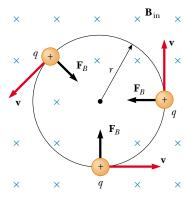
**Figure 29.17** When the velocity of a charged particle is perpendicular to a uniform magnetic field, the particle moves in a circular path in a plane perpendicular to  $\bf B$ . The magnetic force  $\bf F_B$  acting on the charge is always directed toward the center of the circle.
