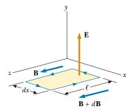
**Figure 34.6** As a plane wave passes through a rectangular path of width dx lying in the xz plane, the magnetic field in the z direction varies from  $\bf B$  to  $\bf B + d\bf B$ . This spatial variation in  $\bf B$  gives rise to a time-varying electric field along the  $\bf y$  direction, according to Equation 34.7.
