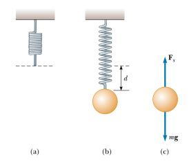
**Figure 7.12** Determining the force constant k of a spring. The elongation d is caused by the attached object, which has a weight mg. Because the spring force balances the force of gravity, it follows that k = mg/d.
