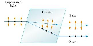
Figure 38.31 Unpolarized light incident on a calcite crystal splits into an ordinary (O) ray and an extraordinary (E) ray. These two rays are polarized in mutually perpendicular directions (drawing not to scale).
