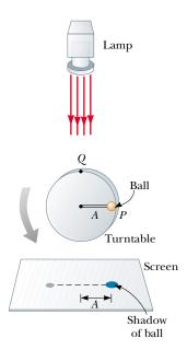
Figure 13.17 An experimental setup for demonstrating the connection between simple harmonic motion and uniform circular motion. As the ball rotates on the turntable with constant angular speed, its shadow on the screen moves back and forth in simple harmonic motion.
