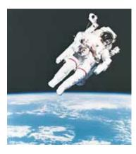
The force from a nitrogen-propelled, hand-controlled device allows an astronaut to move about freely in space without restrictive tethers.
