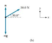
**Figure 7.4** (a) A vacuum cleaner being pulled at an angle of  $30.0^{\circ}$  with the horizontal. (b) Free-body diagram of the forces acting on the vacuum cleaner.
