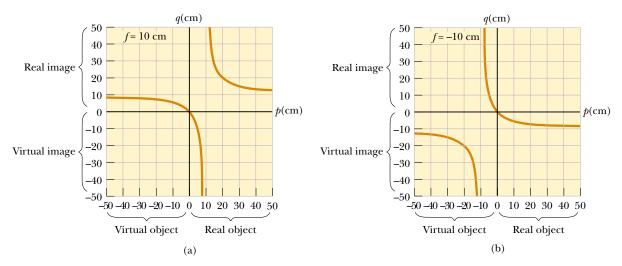
**Figure 36.30** (a) Image position as a function of object position for a lens having a focal length of +10 cm. (b) Image position as a function of object position for a lens having a focal length of -10 cm.
