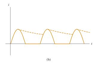
**Figure 33.21** (a) A half-wave rectifier with an optional filter capacitor. (b) Current versus time in the resistor. The solid curve represents the current with no filter capacitor, and the dashed curve is the current when the circuit includes the capacitor.
