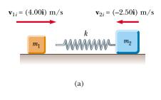
**Solution** To determine the distance that the spring is compressed, shown as x in Figure 9.12b, we can use the concept of conservation of mechanical energy because no friction or other nonconservative forces are acting on the system. Thus, we have
