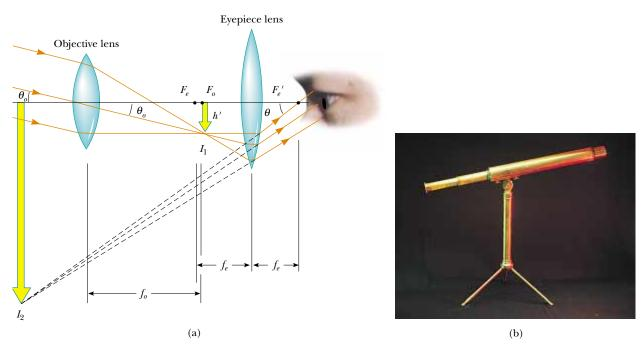
**Figure 36.42** (a) Lens arrangement in a refracting telescope, with the object at infinity. (b) A refracting telescope.
