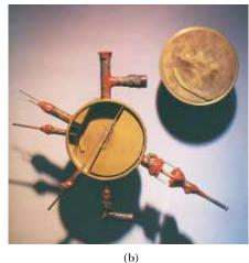
**Figure 29.26** (a) A cyclotron consists of an ion source at P, two dees  $D_1$  and  $D_2$  across which an alternating potential difference is applied, and a uniform magnetic field. (The south pole of the magnet is not shown.) The red dashed curved lines represent the path of the particles. (b) The first cyclotron, invented by E.O. Lawrence and M.S. Livingston in 1934.
