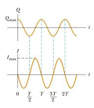
**Figure 32.16** Graphs of charge versus time and current versus time for a resistanceless, nonradiating *LC* circuit. Note that *Q* and *I* are 90° out of phase with each other.
