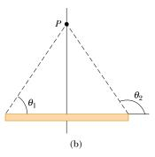
**Figure 30.2** (a) A thin, straight wire carrying a current *I*. The magnetic field at point *P* due to the current in each element  $d\mathbf{s}$  of the wire is out of the page, so the net field at point *P* is also out of the page. (b) The angles  $\theta_1$  and  $\theta_2$ , used for determining the net field. When the wire is infinitely long,  $\theta_1 = 0$  and  $\theta_2 = 180^\circ$ .
