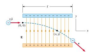
**Figure 23.25** An electron is projected horizontally into a uniform electric field produced by two charged plates. The electron undergoes a downward acceleration (opposite **E**), and its motion is parabolic while it is between the plates.
