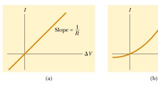
**Figure 27.7** (a) The current–potential difference curve for an ohmic material. The curve is linear, and the slope is equal to the inverse of the resistance of the conductor. (b) A nonlinear current–potential difference curve for a semiconducting diode. This device does not obey Ohm's law.
