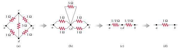
**Figure 28.8** Because of the symmetry in this circuit, the  $5\Omega$  resistor does not contribute to the resistance between points a and b and therefore can be disregarded when we calculate the equivalent resistance.
