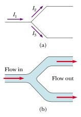
**Figure 28.11** (a) Kirchhoff's junction rule. Conservation of charge requires that all current entering a junction must leave that junction. Therefore,  $I_1 = I_2 + I_3$ . (b) A mechanical analog of the junction rule: the amount of water flowing out of the branches on the right must equal the amount flowing into the single branch on the left.
