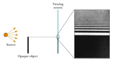
**Figure 38.2** Light from a small source passes by the edge of an opaque object. We might expect no light to appear on the screen below the position of the edge of the object. In reality, light bends around the top edge of the object and enters this region. Because of these effects, a diffraction pattern consisting of bright and dark fringes appears in the region above the edge of the object.
