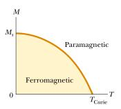
Figure 30.33 Magnetization versus absolute temperature for a ferromagnetic substance. The magnetic moments are aligned below the Curie temperature  $T_{\rm Curie}$ , where the substance is ferromagnetic. The substance becomes paramagnetic (magnetic moments unaligned) above  $T_{\rm Curie}$ .
