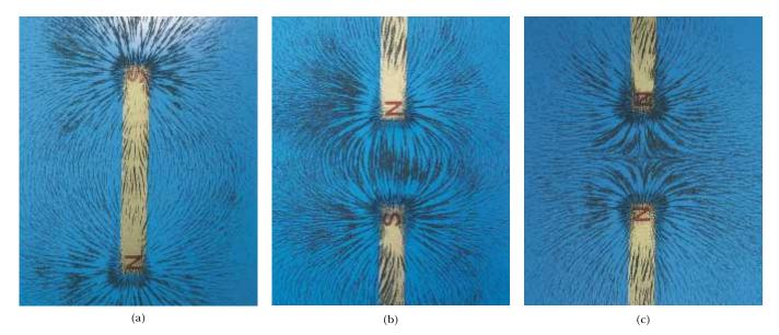
**Figure 29.2** (a) Magnetic field pattern surrounding a bar magnet as displayed with iron filings. (b) Magnetic field pattern between *unlike* poles of two bar magnets. (c) Magnetic field pattern between *like* poles of two bar magnets.
