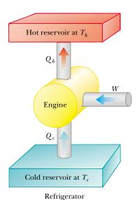
**Figure 22.5** Schematic diagram of a refrigerator, which absorbs energy  $Q_e$  from a cold reservoir and expels energy  $Q_h$  to a hot reservoir. Work W is done on the refrigerator. A heat pump, which can be used to heat or cool a building, works the same way.
