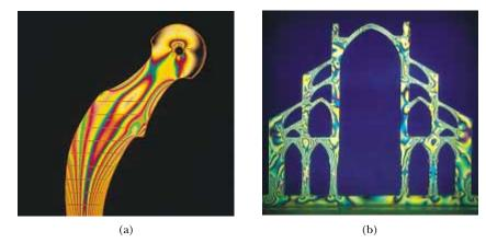
**Figure 38.35** (a) Strain distribution in a plastic model of a hip replacement used in a medical research laboratory. The pattern is produced when the plastic model is viewed between a polarizer and analyzer oriented perpendicular to each other. (b) A plastic model of an arch structure under load conditions observed between perpendicular polarizers. Such patterns are useful in the optimum design of architectural components.
