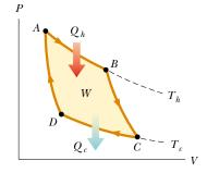
**Figure 22.10** PV diagram for the Carnot cycle. The net work done, W, equals the net energy received in one cycle,  $Q_h - Q_c$ . Note that  $\Delta E_{\rm int} = 0$  for the cycle.
