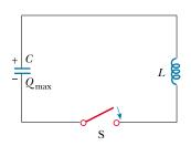
**Figure 32.14** A simple *LC* circuit. The capacitor has an initial charge  $Q_{\text{max}}$ , and the switch is thrown closed at t=0.
