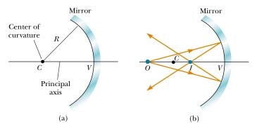
**Figure 36.9** (a) A concave mirror of radius R. The center of curvature C is located on the principal axis. (b) A point object placed at O in front of a concave spherical mirror of radius R, where O is any point on the principal axis farther than R from the mirror surface, forms a real image at I. If the rays diverge from O at small angles, they all reflect through the same image point.
