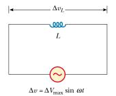
**Figure 33.4** A circuit consisting of an inductor of inductance L connected to an ac generator.
