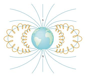
*Figure 29.21* The Van Allen belts are made up of charged particles trapped by the Earth's nonuniform magnetic field. The magnetic field lines are in blue and the particle paths in red.
