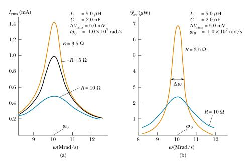
**Figure 33.15** (a) The rms current versus frequency for a series RLC circuit, for three values of R. The current reaches its maximum value at the resonance frequency  $\omega_0$ . (b) Average power versus frequency for the series RLC circuit, for two values of R.
