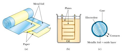
**Figure 26.15** Three commercial capacitor designs. (a) A tubular capacitor, whose plates are separated by paper and then rolled into a cylinder. (b) A high-voltage capacitor consisting of many parallel plates separated by insulating oil. (c) An electrolytic capacitor.
