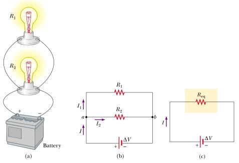
**Figure 28.5** (a) A parallel connection of two resistors  $R_1$  and  $R_2$ . The potential difference across  $R_1$  is the same as that across  $R_2$ . (b) Circuit diagram for the two-resistor circuit. (c) The resistors replaced with a single resistor having an equivalent resistance  $R_{\rm eq} = (R_1^{-1} + R_2^{-1})^{-1}$ .
