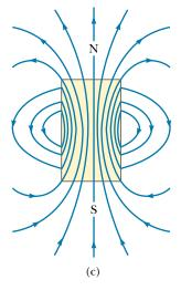
**Figure 30.6** (a) Magnetic field lines surrounding a current loop. (b) Magnetic field lines surrounding a current loop, displayed with iron filings (*Education Development Center, Newton, MA*). (c) Magnetic field lines surrounding a bar magnet. Note the similarity between this line pattern and that of a current loop.
