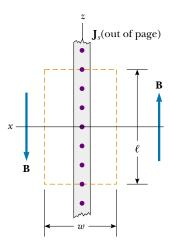
**Figure 30.14** End view of an infinite current sheet lying in the yz plane, where the current is in the yz direction (out of the page). This view shows the direction of  $\mathbf{B}$  on both sides of the sheet.
