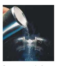
Oxygen, a paramagnetic substance, is attracted to a magnetic field. The liquid oxygen in this photograph is suspended between the poles of the magnet.
