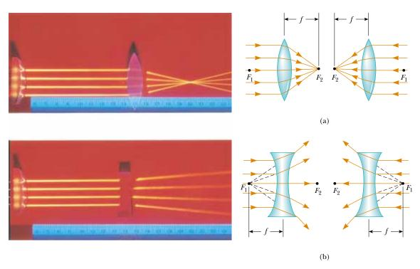
**Figure 36.24** (*Left*) Effects of a converging lens (top) and a diverging lens (bottom) on parallel rays. (*Right*) The object and image focal points of (a) a converging lens and (b) a diverging lens.
