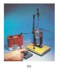
**Figure 28.23** (a) The principal components of a D'Arsonval galvanometer. When the coil situated in a magnetic field carries a current, the magnetic torque causes the coil to twist. The angle through which the coil rotates is proportional to the current in the coil because of the counteracting torque of the spring. (b) A large-scale model of a galvanometer movement. Why does the coil rotate about the vertical axis after the switch is closed?
