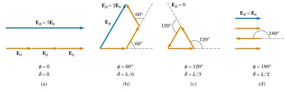
**Figure 37.12** Phasor diagrams for three equally spaced slits at various values of  $\phi$ . Note from (a) that there are primary maxima of amplitude  $3E_0$  and from (d) that there are secondary maxima of amplitude  $E_0$ .
