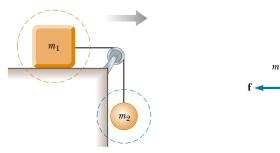
Two masses connected by a light cord. The surface is rough, and the pulley is frictionless.
