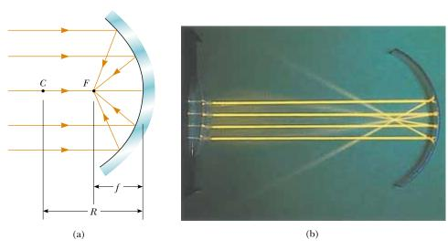
**Figure 36.12** (a) Light rays from a distant object ( $p \approx \infty$ ) reflect from a concave mirror through the focal point *F*. In this case, the image distance  $q \approx R/2 = f$ , where *f* is the focal length of the mirror. (b) Reflection of parallel rays from a concave mirror.
