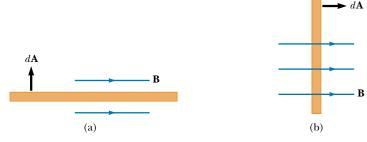
**Figure 30.20** Magnetic flux through a plane lying in a magnetic field. (a) The flux through the plane is zero when the magnetic field is parallel to the plane surface. (b) The flux through the plane is a maximum when the magnetic field is perpendicular to the plane.
