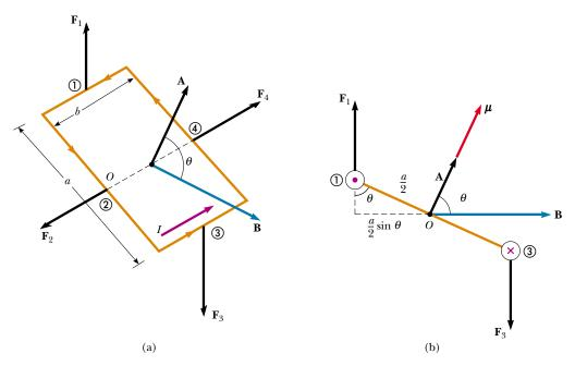
**Figure 29.13** (a) A rectangular current loop in a uniform magnetic field. The area vector **A** perpendicular to the plane of the loop makes an angle  $\theta$  with the field. The magnetic forces exerted on sides ② and ④ cancel, but the forces exerted on sides ① and ③ create a torque on the loop. (b) Edge view of the loop sighting down sides ① and ③.
