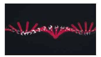
**Figure 9.25** Multiflash photograph showing an overhead view of a wrench moving on a horizontal surface. The center of mass of the wrench moves in a straight line as the wrench rotates about this point, shown by the white dots.
