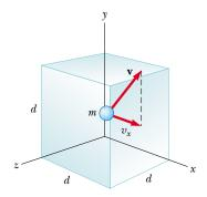
**Figure 21.1** A cubical box with sides of length *d* containing an ideal gas. The molecule shown moves with velocity **v**.
