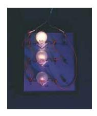
A series connection of three lightbulbs, all rated at 120 V but having power ratings of 60 W, 75 W, and 200 W. Why are the intensities of the bulbs different? Which bulb has the greatest resistance? How would their relative intensities differ if they were connected in parallel?
