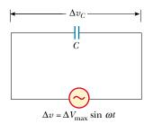
**Figure 33.7** A circuit consisting of a capacitor of capacitance *C* connected to an ac generator.
