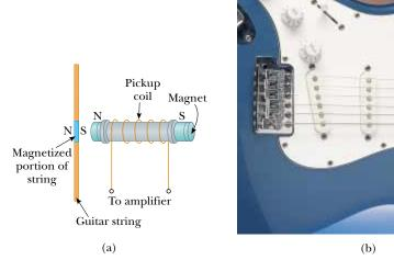
**Figure 31.5** (a) In an electric guitar, a vibrating string induces an emf in a pickup coil. (b) The circles beneath the metallic strings of this electric guitar detect the notes being played and send this information through an amplifier and into speakers. (A switch on the guitar allows the musician to select which set of six is used.) How does a guitar "pickup" sense what music is being played? (b, Charles D. Winters)
