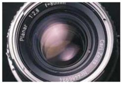
This camera lens has several coatings (of different thicknesses) that minimize reflection of light waves having wavelengths near the center of the visible spectrum. As a result, the little light that is reflected by the lens has a greater proportion of the far ends of the spectrum and appears reddish-violet.
