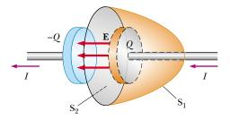
**Figure 30.25** Because it exists only in the wires attached to the capacitor plates, the conduction current I = dQ/dt passes through  $S_1$  but not through  $S_2$ . Only the displacement current  $I_d = \epsilon_0 d\Phi_E/dt$  passes through  $S_2$ . The two currents must be equal for continuity
