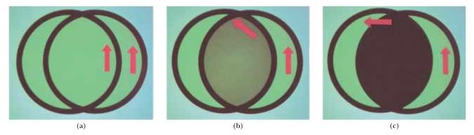
**Figure 38.29** The intensity of light transmitted through two polarizers depends on the relative orientation of their transmission axes. (a) The transmitted light has maximum intensity when the transmission axes are aligned with each other. (b) The transmitted light has lesser intensity when the transmission axes are at an angle of 45° with each other. (c) The transmitted light intensity is a minimum when the transmission axes are at right angles to each other.
