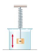
**Figure 32.20** A block–spring system moving in a viscous medium with damped harmonic motion is analogous to an *RLC* circuit.
