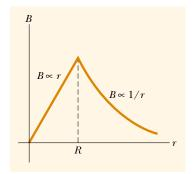
**Figure 30.12** Magnitude of the magnetic field versus r for the wire shown in Figure 30.11. The field is proportional to r inside the wire and varies as 1/r outside the wire.
