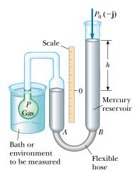
**Figure 19.2** A constant-volume gas thermometer measures the pressure of the gas contained in the flask immersed in the bath. The volume of gas in the flask is kept constant by raising or lowering reservoir *B* to keep the mercury level in column *A* constant.
