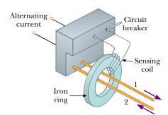
**Figure 31.4** Essential components of a ground fault interrupter.
