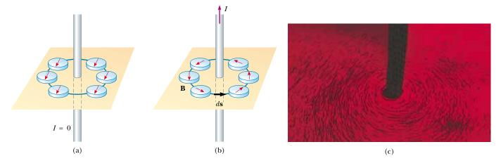
**Figure 30.8** (a) When no current is present in the wire, all compass needles point in the same direction (toward the Earth's north pole). (b) When the wire carries a strong current, the compass needles deflect in a direction tangent to the circle, which is the direction of the magnetic field created by the current. (c) Circular magnetic field lines surrounding a current-carrying conductor, displayed with iron filings.
