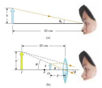
**Figure 36.40** (a) An object placed at the near point of the eye (p = 25 cm) subtends an angle  $\theta_0 \approx h/25$  at the eye. (b) An object placed near the focal point of a converging lens produces a magnified image that subtends an angle  $\theta \approx h'/25$  at the eye.
