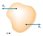
**Figure 12.2** The forces  $\mathbf{F}_1$  and  $\mathbf{F}_2$  are not equivalent because they do not produce the same torque about some axis, even though they are equal in magnitude and opposite in direction.
