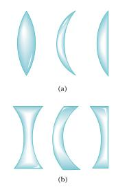
Figure 36.26 Various lens shapes. (a) Biconvex, convex—concave, and plano—convex. These are all converging lenses; they have a positive focal length and are thickest at the middle. (b) Biconcave, convex—concave, and plano—concave. These are all diverging lenses; they have a negative focal length and are thickest at the edges.
