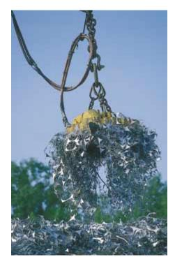
An electromagnet is used to move tons of scrap metal.
