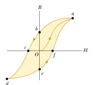
**Figure 30.30** Magnetization curve for a ferromagnetic material.
