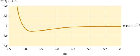
**Figure 8.17** (a) Potential energy curve associated with a molecule. The distance x is the separation between the two atoms making up the molecule. (b) Force exerted on one atom by the other.
