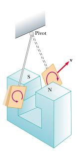
**Figure 31.22** Formation of eddy currents in a conducting plate moving through a magnetic field. As the plate enters or leaves the field, the changing magnetic flux induces an emf, which causes eddy currents in the plate.
