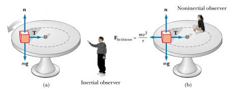
**Figure 6.14** A block of mass m connected to a string tied to the center of a rotating turntable. (a) The inertial observer claims that the force causing the circular motion is provided by the force  $\mathbf{T}$  exerted by the string on the block. (b) The noninertial observer claims that the block is not accelerating, and therefore she introduces a fictitious force of magnitude  $mv^2/r$  that acts outward and balances the force  $\mathbf{T}$ .
