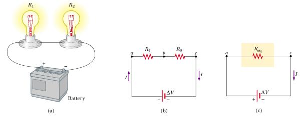
**Figure 28.4** (a) A series connection of two resistors  $R_1$  and  $R_2$ . The current in  $R_1$  is the same as that in  $R_2$ . (b) Circuit diagram for the two-resistor circuit. (c) The resistors replaced with a single resistor having an equivalent resistance  $R_{\rm eq} = R_1 + R_2$ .
