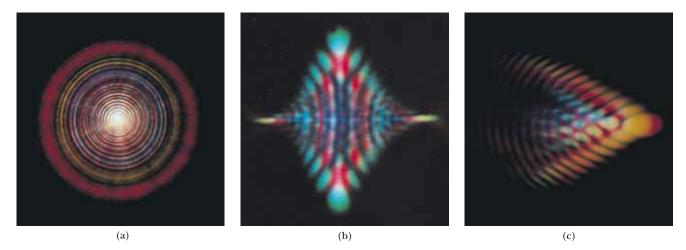
Lens aberrations. (a) *Spherical aberration* occurs when light passing through the lens at different distances from the principal axis is focused at different points. (b) *Astignatism* occurs for objects not located on the principal axis of the lens. (c) *Coma* occurs as light passing through the lens far from the principal axis and light passing near the center of the lens focus at different parts of the focal plane.
