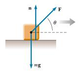
Figure 7.3 When an object is displaced on a frictionless, horizontal, surface, the normal force n and the force of gravity  $m\mathbf{g}$  do no work on the object. In the situation shown here,  $\mathbf{F}$  is the only force doing work on the object.
