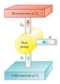
**Figure 22.15** Schematic diagram of a heat pump, which absorbs energy  $Q_e$  from a cold reservoir and expels energy  $Q_h$  to a hot reservoir. Note that this diagram is the same as that for the refrigerator shown in Figure 22.5.
