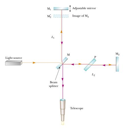
**Figure 37.22** Diagram of the Michelson interferometer. A single ray of light is split into two rays by mirror M, which is called a beam splitter. The path difference between the two rays is varied with the adjustable mirror  $M_1$ . As  $M_1$  is moved toward M, an interference pattern moves across the field of view.
