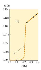
**Figure 27.12** Resistance versus temperature for a sample of mercury (Hg). The graph follows that of a normal metal above the critical temperature  $T_c$ . The resistance drops to zero at  $T_c$ , which is 4.2 K for mercury.
