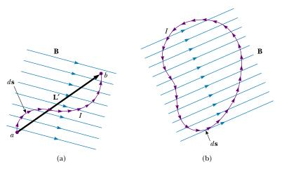
**Figure 29.9** (a) A curved wire carrying a current *I* in a uniform magnetic field. The total magnetic force acting on the wire is equivalent to the force on a straight wire of length *L'* running between the ends of the curved wire. (b) A current-carrying loop of arbitrary shape in a uniform magnetic field. The net magnetic force on the loop is zero.
