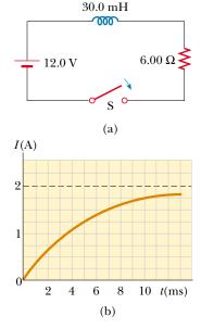
**Figure 32.9** (a) The switch in this RL circuit is thrown closed at t = 0. (b) A graph of the current versus time for the circuit in part (a).
