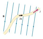
**Figure 29.8** A wire segment of arbitrary shape carrying a current I in a magnetic field  $\mathbf{B}$  experiences a magnetic force. The force on any segment  $d\mathbf{s}$  is  $I d\mathbf{s} \times \mathbf{B}$  and is directed out of the page. You should use the right-hand rule to confirm this force direction.
