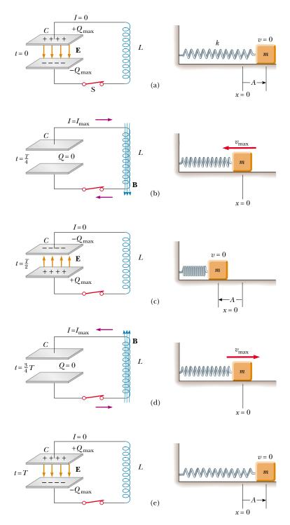
**Figure 32.15** Energy transfer in a resistanceless, non-radiating LC circuit. The capacitor has a charge  $Q_{\max}$  at t=0, the instant at which the switch is thrown closed. The mechanical analog of this circuit is a block-spring system.
