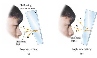
**Figure 36.7** Cross-sectional views of a rearview mirror. (a) With the day setting, the silvered back surface of the mirror reflects a bright ray *B* into the driver's eyes. (b) With the night setting, the glass of the unsilvered front surface of the mirror reflects a dim ray *D* into the driver's eyes.
