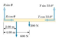
**Figure 12.9** (a) A uniform beam supported by a cable. (b) The free-body diagram for the beam. (c) The free-body diagram for the beam showing the components of **R** and **T**.
