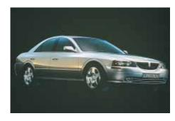
Aerodynamic car. A streamlined body reduces air drag and increases fuel efficiency.
