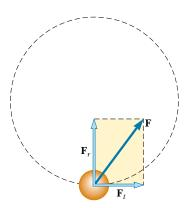
**Figure 6.10** When the force acting on a particle moving in a circular path has a tangential component  $F_t$ , the particle's speed changes. The total force exerted on the particle in this case is the vector sum of the radial force and the tangential force. That is,  $\mathbf{F} = \mathbf{F}_t + \mathbf{F}_t$ .
