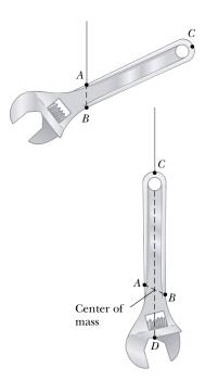
**Figure 9.20** An experimental technique for determining the center of mass of a wrench. The wrench is hung freely first from point *A* and then from point *C*. The intersection of the two lines *AB* and *CD* locates the center of mass.
