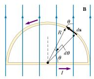
**Figure 29.10** The net force acting on a closed current loop in a uniform magnetic field is zero. In the setup shown here, the force on the straight portion of the loop is 2*IRB* and directed out of the page, and the force on the curved portion is 2*IRB* directed into the page.
