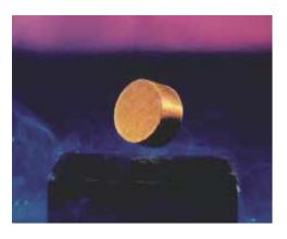
**Figure 30.34** A small permanent magnet levitated above a disk of the superconductor YBa<sub>2</sub>Cu<sub>3</sub>O<sub>7</sub> cooled to liquid nitrogen temperature (77 K).
