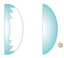
**Figure 36.28** The Fresnel lens on the left has the same focal length as the thick lens on the right but is made of much less glass.
