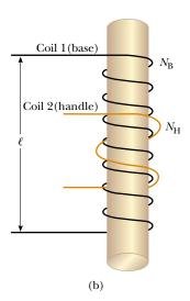
**Figure 32.13** (a) This electric toothbrush uses the mutual induction of solenoids as part of its battery-charging system. (b) A coil of  $N_{\rm H}$  turns wrapped around the center of a solenoid of  $N_{\rm B}$  turns.
