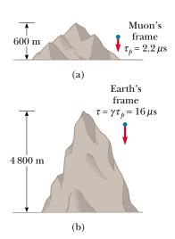
**Figure 39.10** (a) Muons moving with a speed of 0.99c travel approximately 600 m as measured in the reference frame of the muons, where their lifetime is about  $2.2 \mu s$ . (b) The muons travel approximately  $4\,800$  m as measured by an observer on the Earth.
