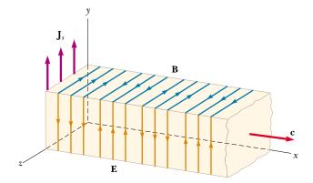
**Figure 34.11** Representation of the plane electromagnetic wave radiated by an infinite current sheet lying in the yz plane. The vector  $\mathbf{B}$  is in the z direction, the vector  $\mathbf{E}$  is in the y direction, and the direction of wave motion is along x. Both vector  $\mathbf{B}$  and vector  $\mathbf{E}$  behave according to the expression  $\cos(kx - \omega t)$ . Compare this drawing with Figure 34.3a.
