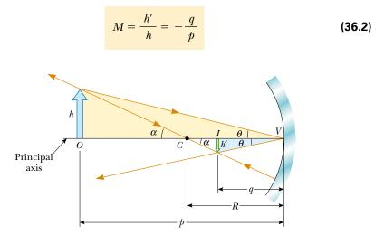
**Figure 36.11** The image formed by a spherical concave mirror when the object O lies outside the center of curvature C.
