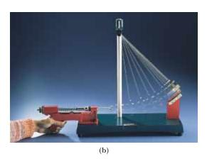
**Figure 9.11** (a) Diagram of a ballistic pendulum. Note that  $\mathbf{v}_{1i}$  is the velocity of the bullet just before the collision and  $\mathbf{v}_f = \mathbf{v}_{1f} = \mathbf{v}_{2f}$  is the velocity of the bullet + block system just after the perfectly inelastic collision. (b) Multiflash photograph of a ballistic pendulum used in the laboratory.
