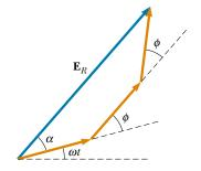
**Figure 37.11** Phasor diagram for three equally spaced slits.
