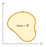
**Figure 22.3** PV diagram for an arbitrary cyclic process. The value of the net work done equals the area enclosed by the curve.
