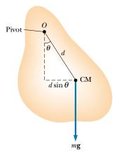
Figure 13.13 A physical pendulum
