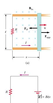
**Figure 31.9** (a) A conducting bar sliding with a velocity  $\mathbf{v}$  along two conducting rails under the action of an applied force  $\mathbf{F}_{app}$ . The magnetic force  $\mathbf{F}_B$  opposes the motion, and a counterclockwise current I is induced in the loop. (b) The equivalent circuit diagram for the setup shown in part (a).
