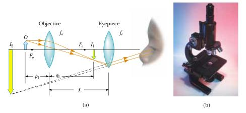
**Figure 36.41** (a) Diagram of a compound microscope, which consists of an objective lens and an eyepiece lens. (b) A compound microscope. The three-objective turret allows the user to choose from several powers of magnification. Combinations of eyepieces with different focal lengths and different objectives can produce a wide range of magnifications.
