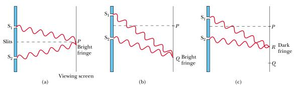
**Figure 37.3** (a) Constructive interference occurs at point P when the waves combine. (b) Constructive interference also occurs at point Q. (c) Destructive interference occurs at R when the two waves combine because the upper wave falls half a wavelength behind the lower wave (all figures not to scale).
