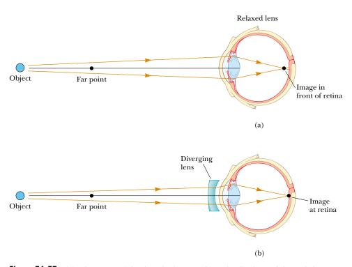
*Figure 36.37* (a) When a nearsighted eye looks at an object that lies beyond the eye's far point, the image is formed in front of the retina, resulting in blurred vision. (b) Nearsightedness is corrected with a diverging lens.
