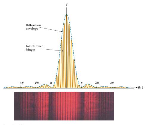
**Figure 38.11** The combined effects of diffraction and interference. This is the pattern produced when 650-nm light waves pass through two 3.0- $\mu$ m slits that are 18  $\mu$ m apart. Notice how the diffraction pattern acts as an "envelope" and controls the intensity of the regularly spaced interference maxima.
