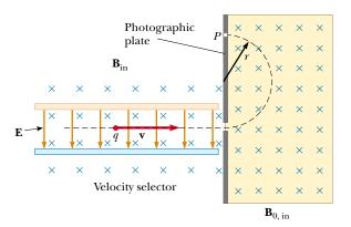
**Figure 29.23** A mass spectrometer. Positively charged particles are sent first through a velocity selector and then into a region where the magnetic field  $\mathbf{B}_0$  causes the particles to move in a semicircular path and strike a photographic film at P.
