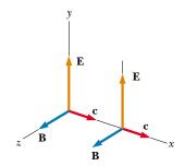
**Figure 34.2** An electromagnetic wave traveling at velocity  $\mathbf{c}$  in the positive x direction. The electric field is along the y direction, and the magnetic field is along the z direction. These fields depend only on x and t.
