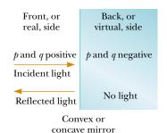
**Figure 36.14** Signs of p and q for convex and concave mirrors.
