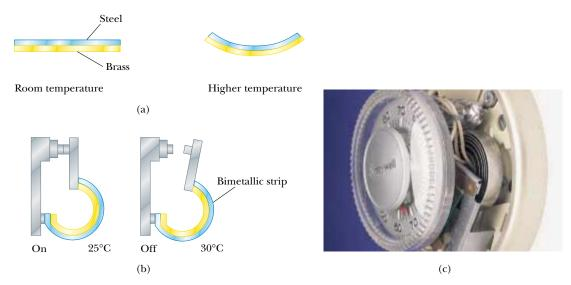
**Figure 19.9** (a) A bimetallic strip bends as the temperature changes because the two metals have different expansion coefficients. (b) A bimetallic strip used in a thermostat to break or make electrical contact. (c) The interior of a thermostat, showing the coiled bimetallic strip. Why do you suppose the strip is coiled?
