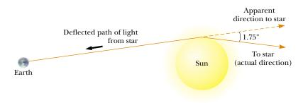
**Figure 39.23** Deflection of starlight passing near the Sun. Because of this effect, the Sun or some other remote object can act as a *gravitational lens*. In his general theory of relativity, Einstein calculated that starlight just grazing the Sun's surface should be deflected by an angle of 1.75".
