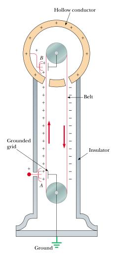
**Figure 25.27** Schematic diagram of a Van de Graaff generator. Charge is transferred to the hollow conductor at the top by means of a moving belt. The charge is deposited on the belt at point *A* and transferred to the hollow conductor at point *B*.
