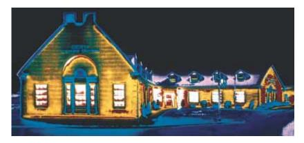
This thermogram of a home, made during cold weather, shows colors ranging from white and orange (areas of greatest energy loss) to blue and purple (areas of least energy loss).
