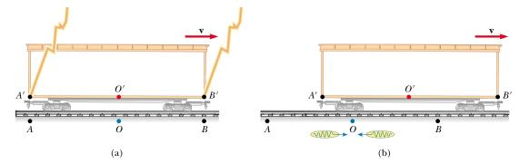
**Figure 39.7** (a) Two lightning bolts strike the ends of a moving boxcar. (b) The events appear to be simultaneous to the stationary observer O, standing midway between A and B. The events do not appear to be simultaneous to observer O', who claims that the front of the car is struck before the rear. Note that in (b) the leftward-traveling light signal has already passed O' but the rightward-traveling signal has not yet reached O'.
