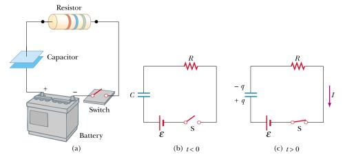
**Figure 28.16** (a) A capacitor in series with a resistor, switch, and battery. (b) Circuit diagram representing this system at time t < 0, before the switch is closed. (c) Circuit diagram at time t > 0, after the switch has been closed.
