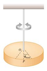
Figure 13.15 A torsional pendulum consists of a rigid body suspended by a wire attached to a rigid support. The body oscillates about the line OP with an amplitude  $\theta_{\max}$ .
