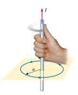
**Figure 30.3** The right-hand rule for determining the direction of the magnetic field surrounding a long, straight wire carrying a current. Note that the magnetic field lines form circles around the wire.
