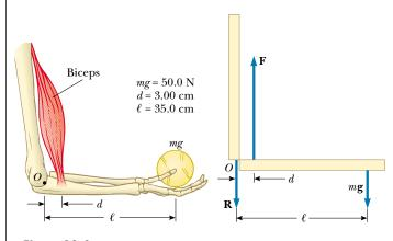
**Figure 12.8** (a) The biceps muscle pulls upward with a force **F** that is essentially at right angles to the forearm. (b) The mechanical model for the system described in part (a).
