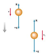
**Figure 6.16** An object falling through air experiences a resistive force  $\mathbf{R}$  and a gravitational force  $\mathbf{F}_g = m\mathbf{g}$ . The object reaches terminal speed (on the right) when the net force acting on it is zero, that is, when  $\mathbf{R} = -\mathbf{F}_g$  or R = mg. Before this occurs, the acceleration varies with speed according to Equation 6.8.
