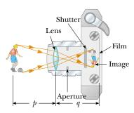
**Figure 36.33** Cross-sectional view of a simple camera. Note that in reality,  $p \gg q$ .
