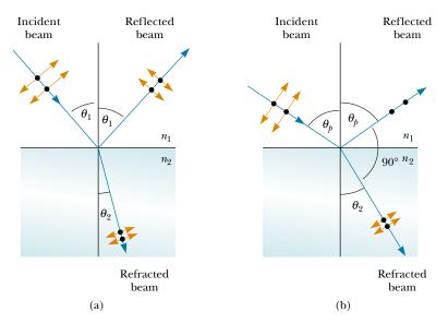
**Figure 38.30** (a) When unpolarized light is incident on a reflecting surface, the reflected and refracted beams are partially polarized. (b) The reflected beam is completely polarized when the angle of incidence equals the polarizing angle  $\theta_p$ , which satisfies the equation  $n = \tan \theta_p$ .
