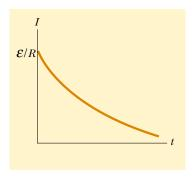
**Figure 32.7** Current versus time for the upper loop of the circuit shown in Figure 32.6. For t < 0,  $S_1$  is closed and  $S_2$  is open. At t = 0,  $S_2$  is closed as  $S_1$  is opened, and the current has its maximum value  $\mathcal{E}/R$ .
