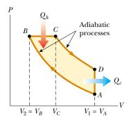
Figure 22.13 PV diagram for an ideal diesel engine.
