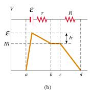
**Figure 28.2** (a) Circuit diagram of a source of emf  $\mathcal{E}$  (in this case, a battery), of internal resistance r, connected to an external resistor of resistance R. (b) Graphical representation showing how the electric potential changes as the circuit in part (a) is traversed clockwise.
