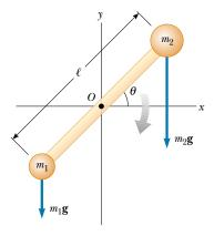
**Figure 11.14** Because gravitational forces act on the rotating rod, there is in general a net nonzero torque about O when  $m_1 \neq m_2$ . This net torque produces an angular acceleration given by  $\alpha = \sum \tau_{\text{ext}} / I$ .
