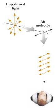
**Figure 38.34** The scattering of unpolarized sunlight by air molecules. The scattered light traveling perpendicular to the incident light is plane-polarized because the vertical vibrations of the charges in the air molecule send no light in this direction.
