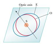
**Figure 38.32** A point source S inside a double-refracting crystal produces a spherical wave front corresponding to the ordinary ray and an elliptical wave front corresponding to the extraordinary ray. The two waves propagate with the same velocity along the optic axis.
