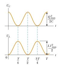
**Figure 32.17** Plots of  $U_C$  versus t and  $U_L$  versus t for a resistanceless, nonradiating LC circuit. The sum of the two curves is a constant and equal to the total energy stored in the circuit.
