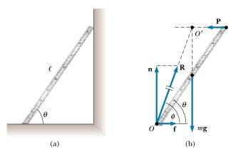
**Figure 12.10** (a) A uniform ladder at rest, leaning against a smooth wall. The ground is rough. (b) The free-body diagram for the ladder. Note that the forces  $\mathbf{R}$ ,  $m\mathbf{g}$ , and  $\mathbf{P}$  pass through a common point O'.
