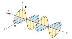
**Figure 38.26** Schematic diagram of an electromagnetic wave propagating at velocity  $\mathbf{c}$  in the x direction. The electric field vibrates in the xy plane, and the magnetic field vibrates in the xz plane.
