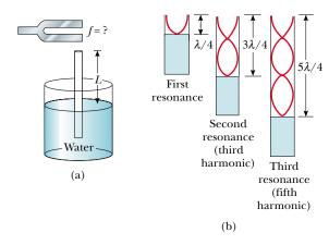
**Figure 18.15** (a) Apparatus for demonstrating the resonance of sound waves in a tube closed at one end. The length L of the air column is varied by moving the tube vertically while it is partially submerged in water. (b) The first three normal modes of the system shown in part (a).
