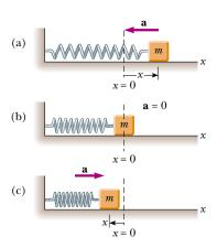
**Figure 13.5** A block of mass m attached to a spring on a frictionless surface undergoes simple harmonic motion. (a) When the block is displaced to the right of equilibrium, the displacement is positive and the acceleration is negative. (b) At the equilibrium position, x = 0, the acceleration is zero and the speed is a maximum. (c) When the block is displaced to the left of equilibrium, the displacement is negative and the acceleration is positive.
