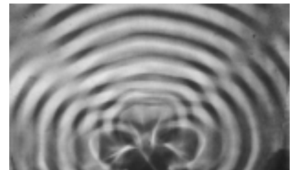
w / A pretty good simulation of the single-slit pattern of figure u, made by using three motors to produce overlapping ripples from three neighboring points in the water.
