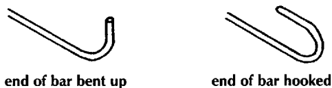
Fig. 91 Ends of reinforcing rods.
