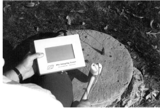
Fig. 7.29 Pile Integrity Tester. (Courtesy of Pile Dynamics, Inc., Cleveland, Ohio.)
