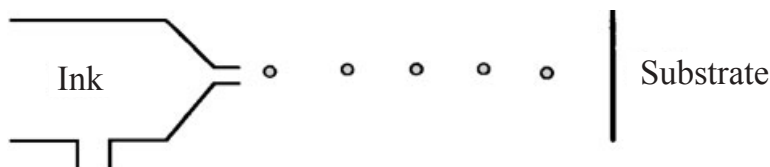
Figure 6.6 Principle of ink-jet printing
