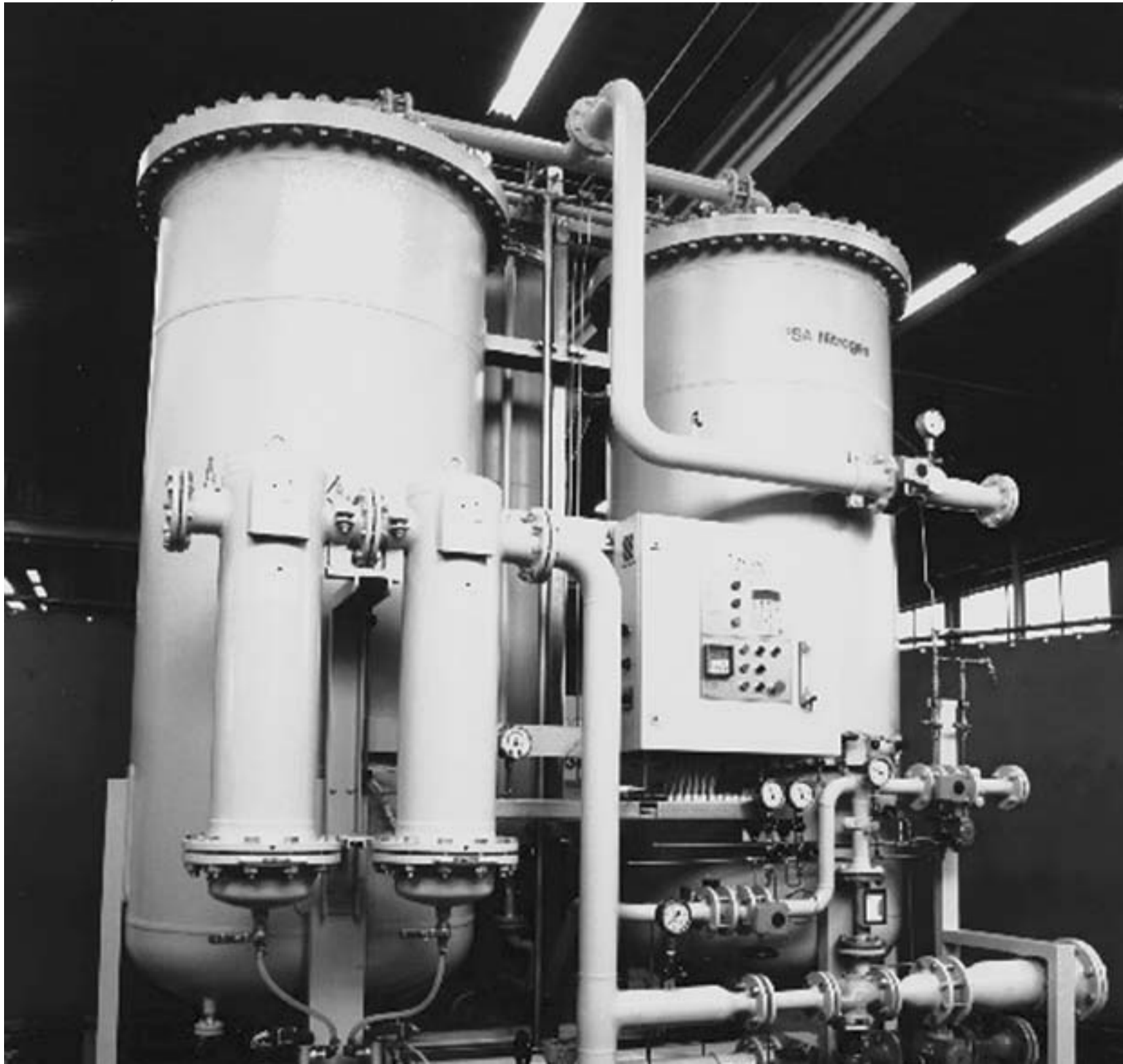
Fig. 13.4 An on-site nitrogen PSA supply system. The large vessels are absorbers and the smaller ones are dryers. (Courtesy Cirmac International, B.V., Netherlands)
