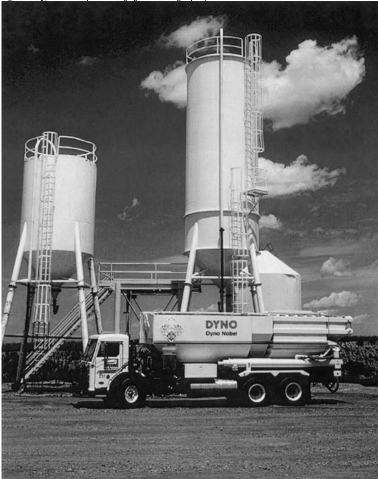
Fig. 31.10 Typical bulk explosives staging area in a large open-pit mine.
