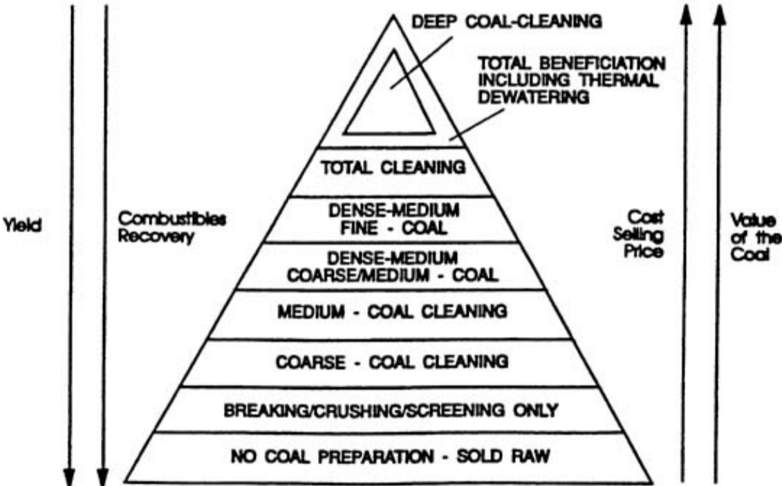
Fig. 17.6 Different levels of coal cleaning and the effect on coal recovery and economics.
