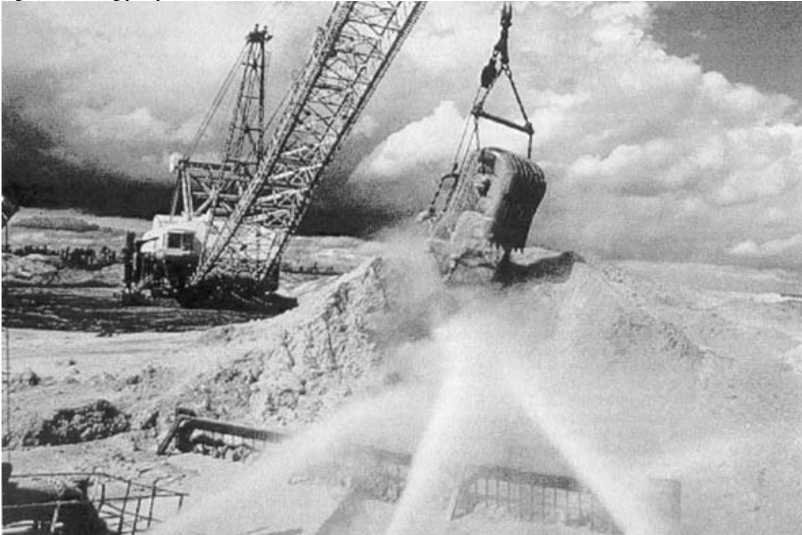
Fig. 10.4 Gunning phosphate rock in a Florida mine.
