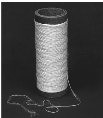
Figure 3.3 Textile fibers of [\text{NP}(\text{OCH}_2\text{CF}_3)_2]_n , a non-burning polymer. Reproduced by permission of Ethyl Corporation.
