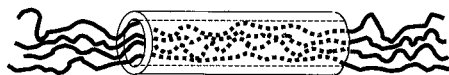
Figure 8.11 Polymer chains being threaded through a porous inorganic material such as a zeolite by polymerizing monomer that had been absorbed into one of the channels or cavities.
