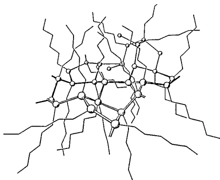
Figure 5.24 The network structure proposed for (n\text{-HexSi})_n . Large spheres represent Si atoms. Reprinted with permission from Bianconi et al., Macromolecules 1989, 22, 1697. Copyright 1989 American Chemical Society.
