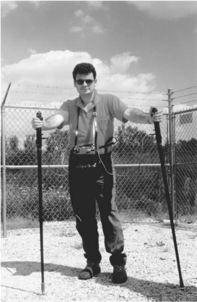
Figure 11.26 DCVG measuring equipment. (Courtesy of CSIR North America Inc.)
