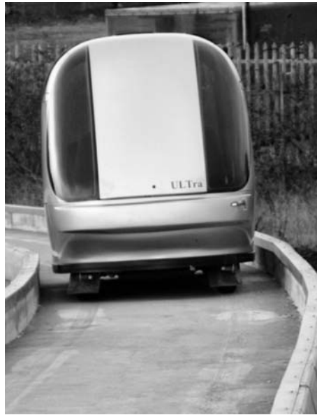
Figure 10.18 Front view of ULTra vehicle on guideway. (Courtesy of Advanced Transport Systems, Ltd.)
