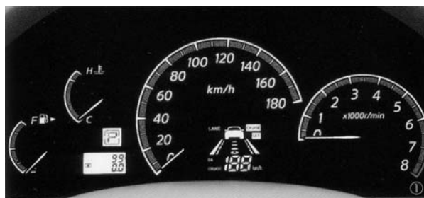
Figure 6.9 Nissan LKS driver interface integrated into instrument panel. (Source: Nissan.)
