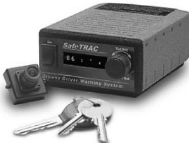
Figure 6.2 SafeTRAC camera (left) and combination processing and driver interface unit (right). (Source: AssistWare Technology.)
