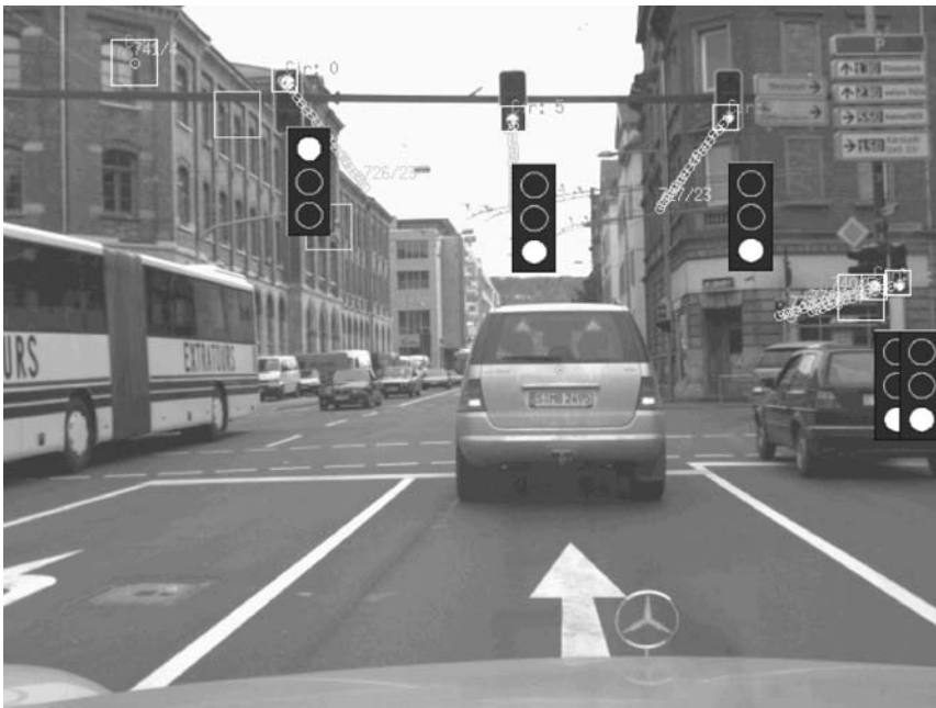
Figure 8.3 Traffic light detection and state detection by DaimlerChrysler's vision system. (Courtesy of Profs. U. Franke and F. Linder, DaimlerChrysler AG.)
