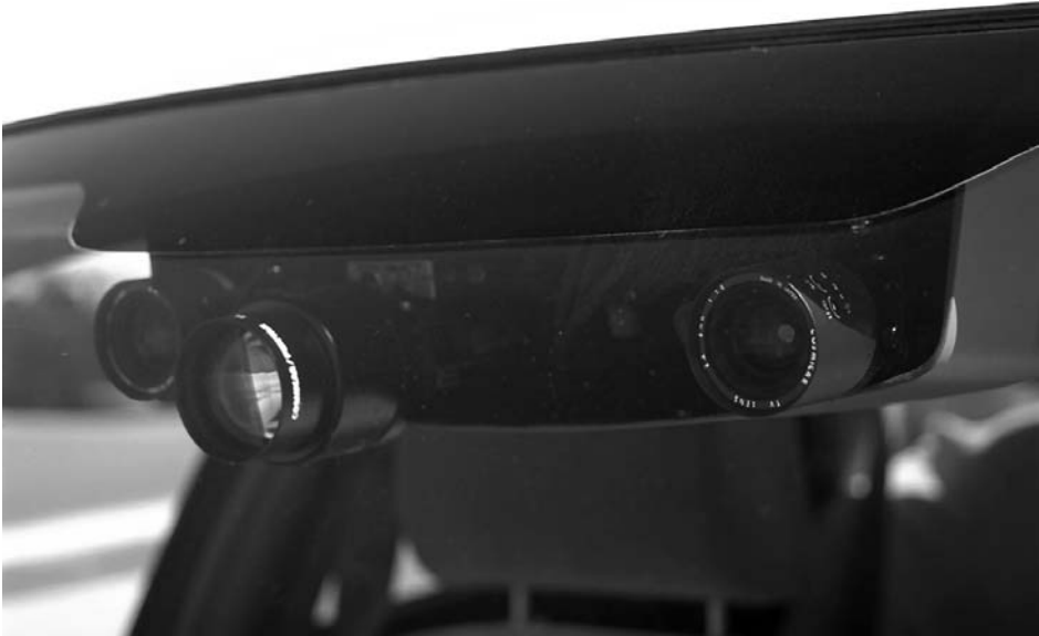
Figure 10.5 Camera system used in Honda vehicles at Demo '97. (Courtesy of California PATH.)
