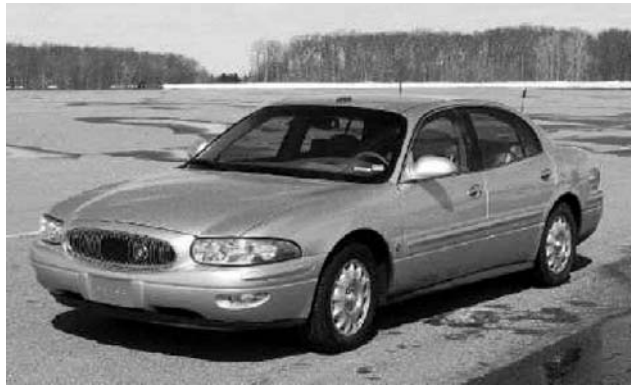
Figure 7.10 One of 10 Buick LeSabre test vehicles used in the ACAS forward collision warning/adaptive cruise control field operational test. (Source: General Motors.)
