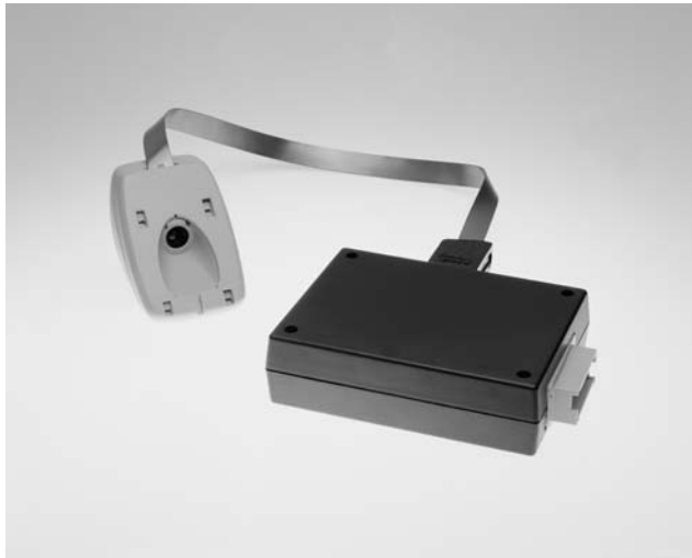
Figure 6.3 Iteris's first generation LDWS. Used in the United States commercial market starting in 2002. (Source: Iteris, Inc.)
