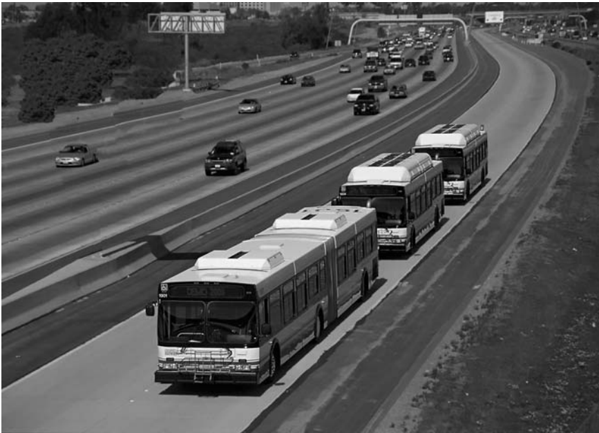
Figure 10.16 Buses in automated platoon mode on I-15 in San Diego, California. (Courtesy of California PATH.)
