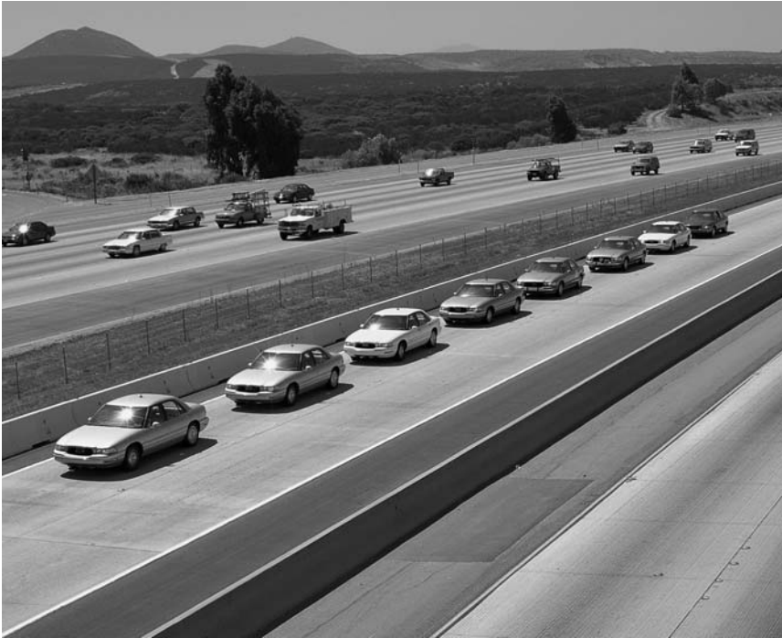
Figure 10.1 PATH vehicles in platoon formation at 60 mph during Demo '97. (Courtesy of California PATH.)
