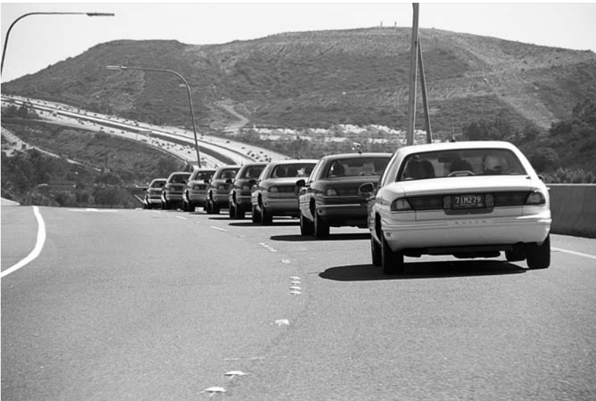
Figure 10.2 A perspective indicating tight intervehicle spacing within platoons at Demo '97. (Courtesy of California PATH.)
