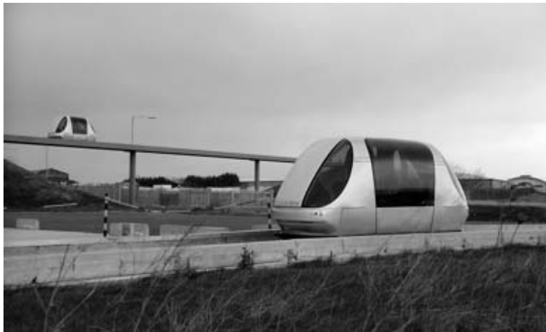
Figure 10.19 Elevated and ground-level ULTra guideways. (Courtesy of Advanced Transport Systems, Ltd.)
