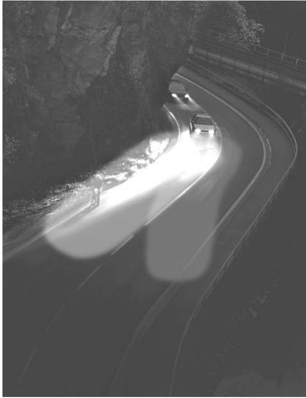
Figure 7.3 AFS improves roadside illumination on curving roads. (Source: Visteon.)
