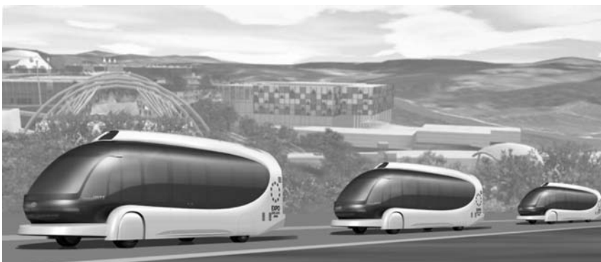
Figure 10.11 An artist's rendering of IMTS in platoon operation at EXPO 2005 Aichi, Japan. (Source: Toyota.)
