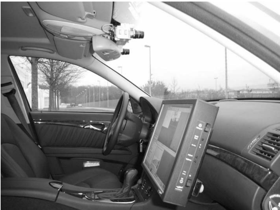
Figure 7.13 Stereo vision camera set up in the DaimlerChrysler PROTECTOR System. (Courtesy of Prof. D. M. Gavrilu, DaimlerChrysler AG.)
