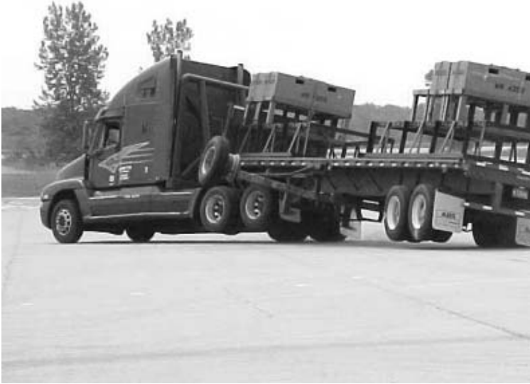
Figure 6.13 Photo of tractor-trailer on a test track invoking roll forces (note that the tractor is relatively stable while the trailer is in serious trouble). ( Photo courtesy of Meritor WABCO. )
