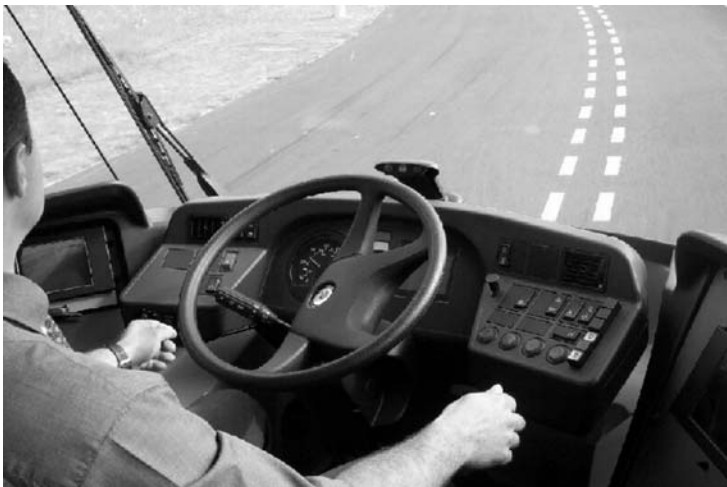
Figure 6.7 Specialized pavement markings used by the CIVIS system for lane-tracking. (Source: Irisbus.)
