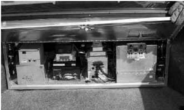
Figure 7.11 ACAS data acquisition systems housed in the trunk of the test vehicles. (Source: General Motors.)
