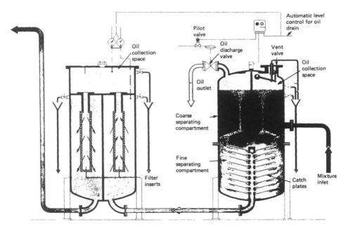
Figure 7.8 Oily water separator
