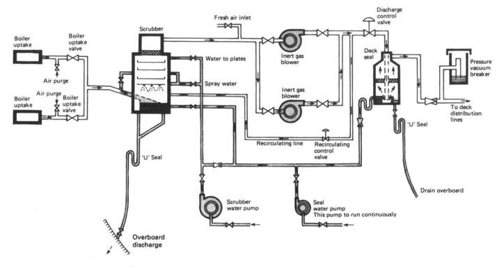
Figure 13.14 Funnel gas inerting system
