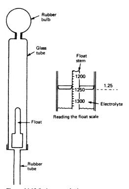
Figure 14.13 Syringe-type hydrometer
