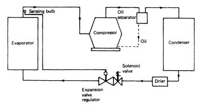
Figure 9.1 Vapour compression cycle
