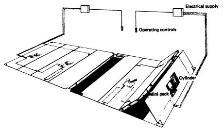
Figure 10.6 Tween-deck hatch cover
