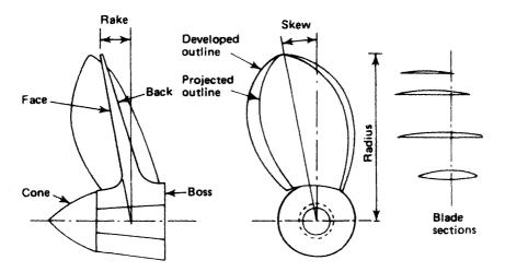
Figure 11.5 Solid propeller
