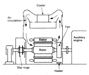
Figure 14.7 Alternator construction
