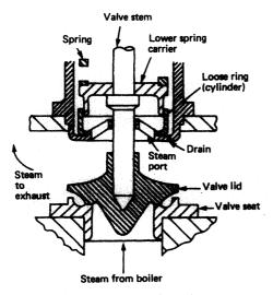
Figure 4.14 Improved high-lift safety valve
