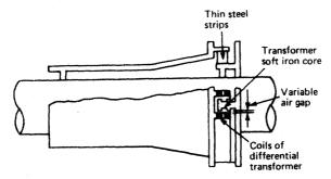
Figure 15.19 Differential transformer torsionmeter
