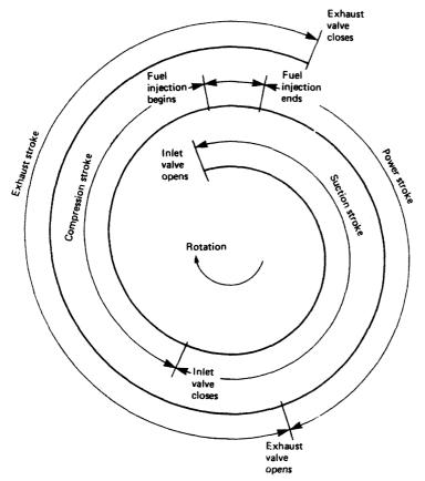
Figure 2.2 Four-stroke timing diagram
