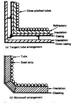
Figure 4.6 Furnace wall construction
