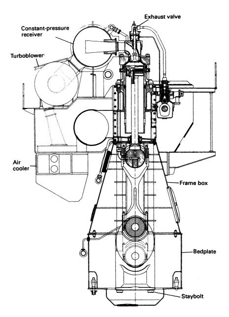
Figure 2.29 MAN B&W L70MC engine
