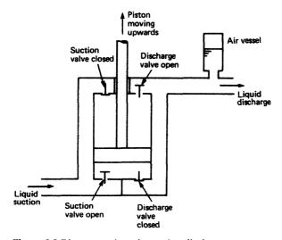
Figure 6.3 Diagrammatic reciprocating displacement pump
