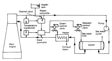
Figure 15.40 Cooling water temperature control
