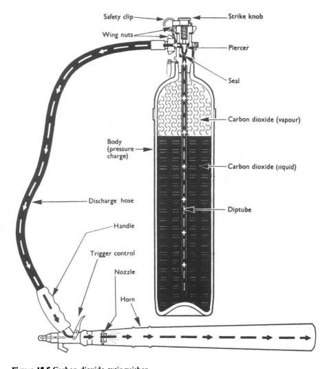
Figure 13.6 Carbon dioxide extinguisher
