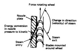
Figure 3.1 Energy conversion in a steam turbine
