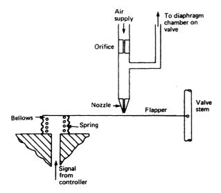
Figure 15.35 Valve positioner
