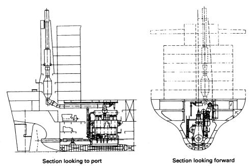
Figure 1.2 Slow-speed diesel machinery arrangement
