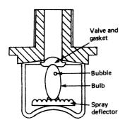
Figure 13.9 Sprinkler head
