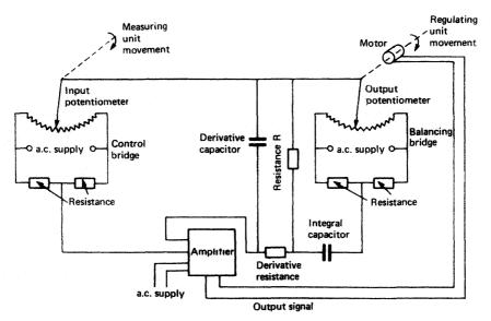
Figure 15.33 Electronic three-term controller
