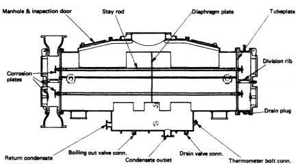
Figure 5.5 Auxiliary condenser
