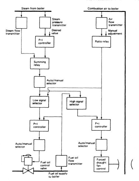
Figure 15.39 Boiler combustion control
