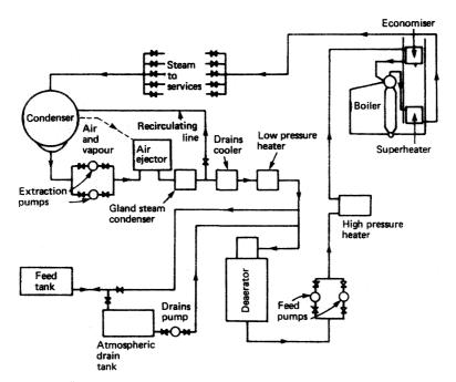
Figure 5.2 Closed feed system
