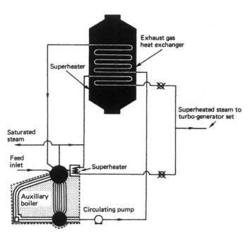
Figure 4.10 Auxiliary steam plant system
