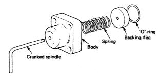
Figure 7.2 Water jacket safety valve
