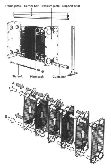
Figure 7.5 Plate-type heat exchanger: (a) construction, (b) operation
