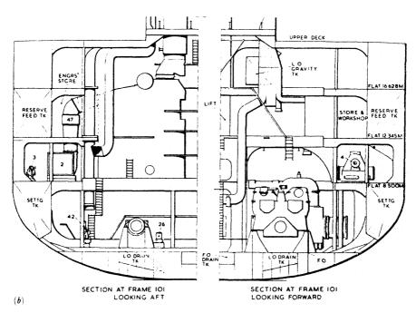
Figure 1.4 Steam turbine machinery arrangement
