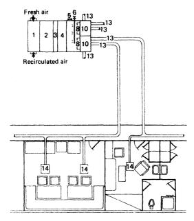
Figure 9.10 Single-duct system
