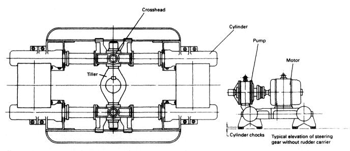
Figure 12.7 Four-ram steering gear—actual arrangement
