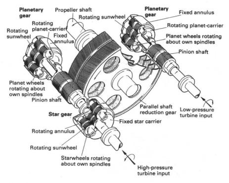
Figure 3.13 Typical marine turbine reduction gear
