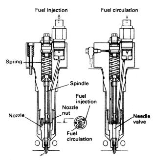
Figure 2.16 Fuel injector
