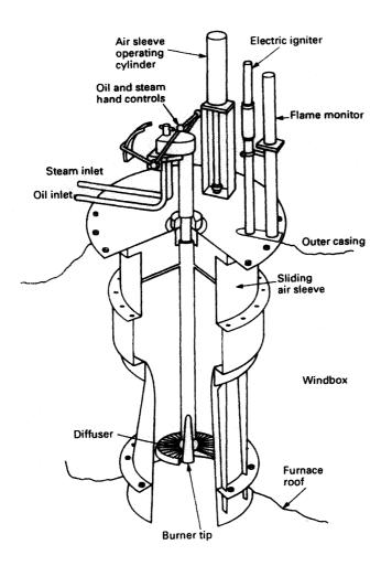
Figure 4.17(b) Air register for roof-fired boiler
