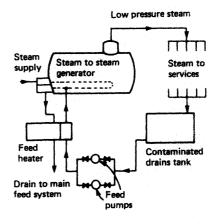
Figure 5.4 Steam-to-steam generator feed system
