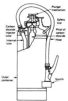
Figure 13.7 Dry powder extinguisher
