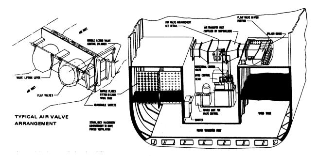
Figure 10.8 Air-controlled tank stabiliser
