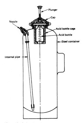
Figure 13.4 Soda-acid extinguisher
