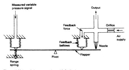
Figure 15.26 Force balance transmitter with feedback
