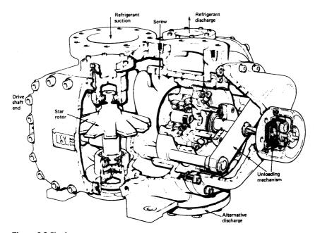
Figure 9.3 Single-screw compressor
