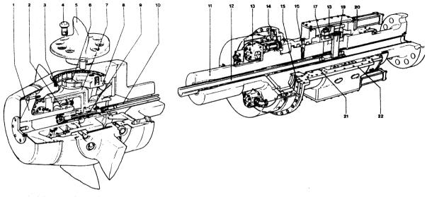
Figure 11.7 Controllable-pitch propeller
