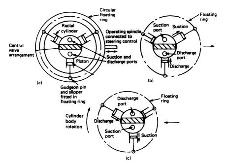
Figure 12.2 Hele-Shaw pump—operating principle
