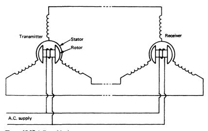
Figure 15.27 A.C. positioning motors
