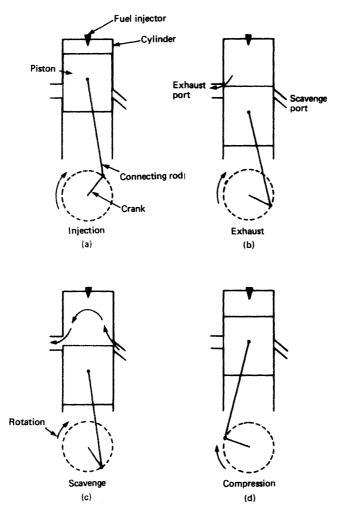
Figure 2.3 Two-stroke cycle
