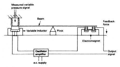
Figure 15.28 Force balance electronic transmitter
