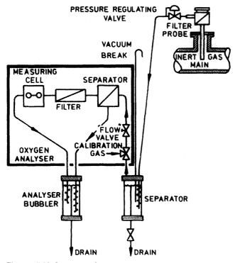
Figure 15.22 Oxygen analyser
