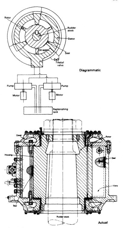
Figure 12.9(a) Rotary vane steering gear
