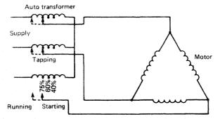
Figure 14.12 Squirrel cage induction motor starting
