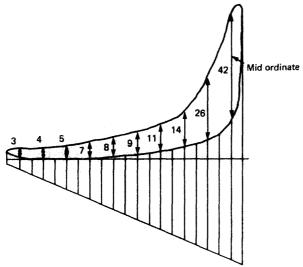
Figure A.2 Indicator diagram
