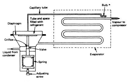
Figure 9.6 Thermostatic expansion valve or regulator
