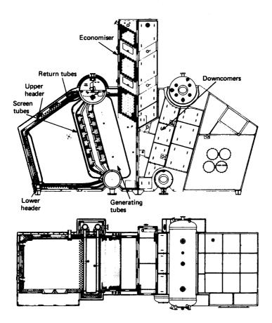
Figure 4.2 Foster Wheeler D-Type boiler
