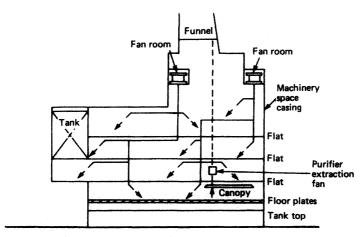
Figure 9.13 Machinery space ventilation—diagrammatic
