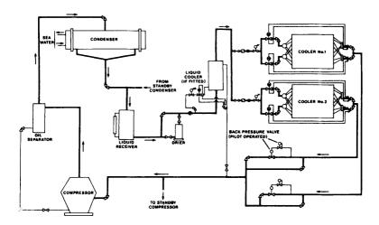
Figure 9.9 Direct expansion system
