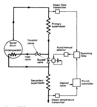
Figure 15.38 Steam temperature control
