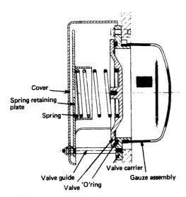
Figure 2.24 Crankcase explosion relief valve
