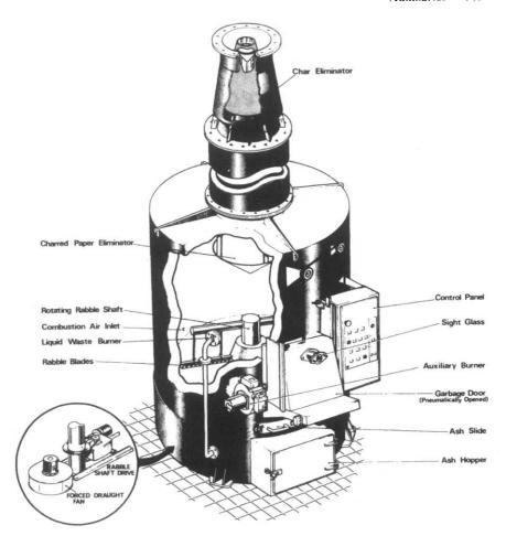
Figure 7.11 Incinerator
