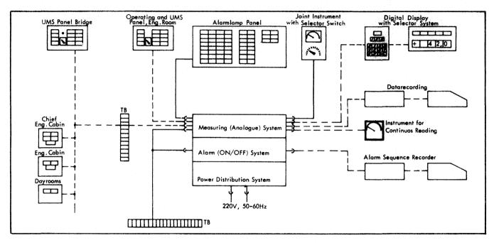
Figure 15.42 Data logging and alarm monitoring system
