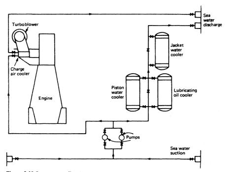
Figure 2.19 Sea water cooling system
