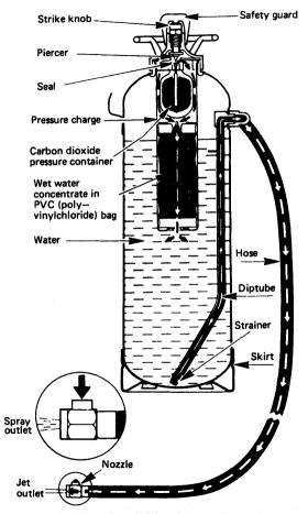
Figure 13.5(b) Foam fire extinguishers—mechanical foam
