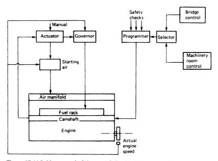
Figure 15.44 Bridge control of slow-speed diesel engine
