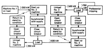
Figure 15.47 Automatic load control of alternators
