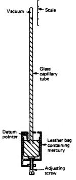
Figure 15.2 Mercury barometer
