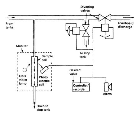
Figure 15.23 Oil-in-water monitoring system
