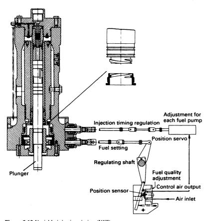
Figure 2.13 Variable injection timing (VIT) pump
