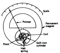
Figure 15.14 Moving coil meter
