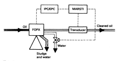
Figure 8.4 Fuel oil separation control
