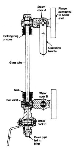
Figure 4.11 Tubular gauge glass
