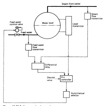
Figure 15.36 Boiler water level control
