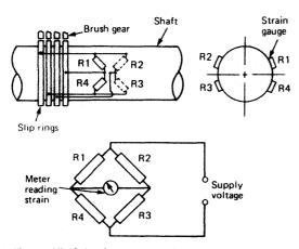
Figure 15.18 Strain gauge torsionmeter
