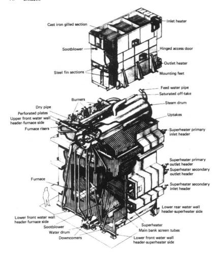
Figure 4.4 Foster Wheeler Type ESD III monowall boiler
