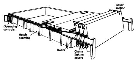
Figure 10.5 Weather-deck hatch cover
