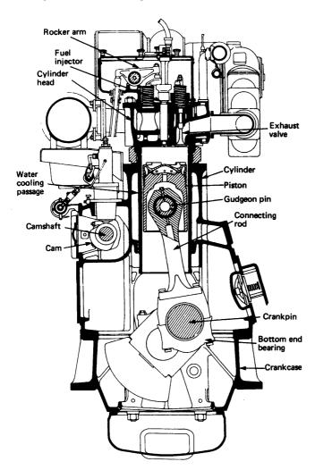
Figure 2.6 Cross-section of a four-stroke diesel engine
