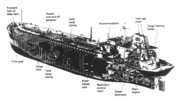
Figure 1.1 Cutaway drawing of a ship
