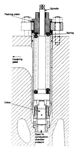
Figure 2.23 Cylinder relief valve
