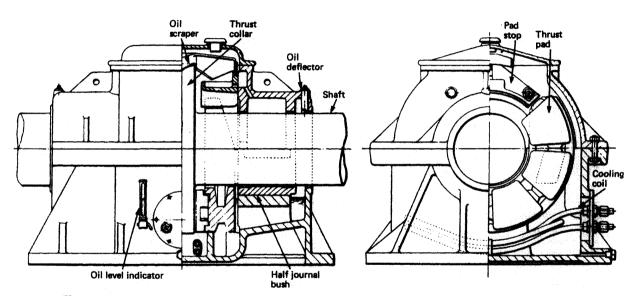
Figure 11.2 Thrust block
