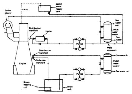
Figure 2.18 Fresh water cooling system
