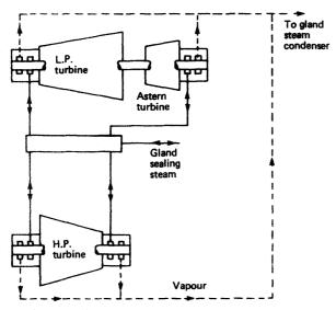
Figure 3.9 Gland steam sealing system
