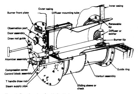
Figure 4.17(a) Air register for side-fired boiler
