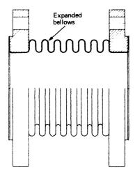
Figure 6.18 Expansion bellows piece
