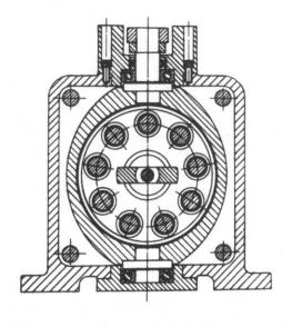
Figure 12.3 Swash plate pump
