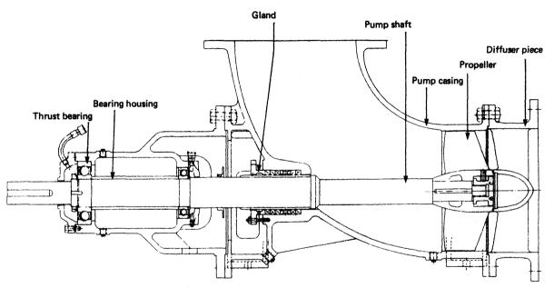
Figure 6.5 Axial-flow pump
