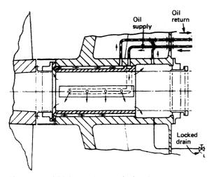
Figure 11.4 Oil lubricated sterntube bearing
