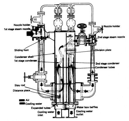
Figure 5.7 Air ejector
