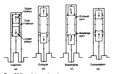
Figure 2.5 Opposed piston engine cycle
