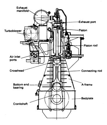
Figure 2.7 Cross-section of a two-stroke diesel engine
