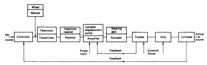
Figure 15.46 Automatic steering system
