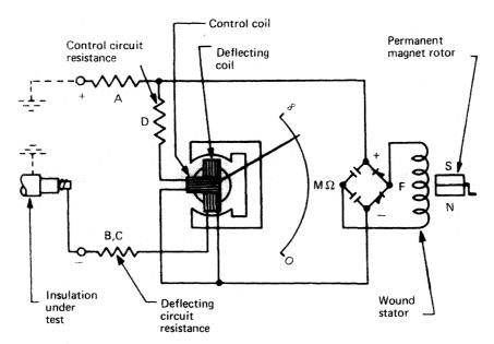
Figure 14.16 Insulation tester
