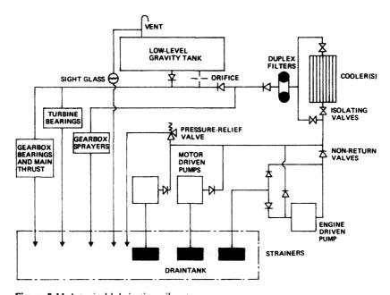
Figure 3.11 A typical lubricating oil system
