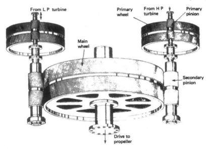
Figure 3.14 Double reduction system of gearing
