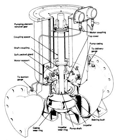
Figure 6.8 Double-entry centrifugal pump
