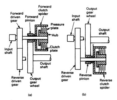
Figure 2.26 Plate-type clutch
