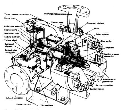
Figure 5.10 Turbo-feed pump
