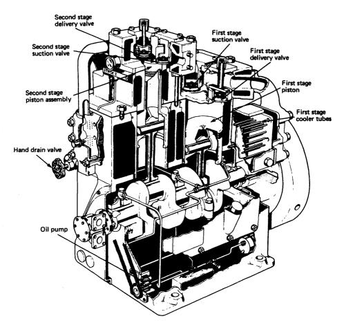
Figure 7.1 Two-stage air compressor
