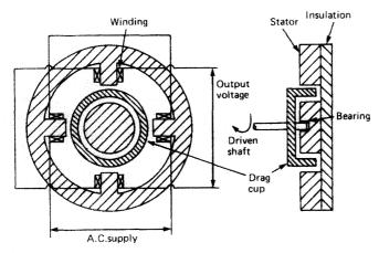
Figure 15.16 Drag cup generator-type tachometer
