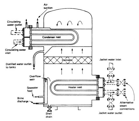
Figure 7.6 Boiling process evaporator
