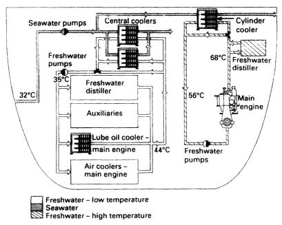
Figure 2.20 Central cooling system
