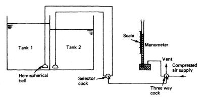
Figure 15.10 Pneumatic gauge
