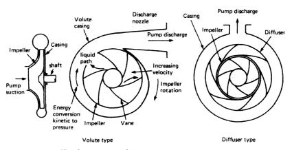
Figure 6.6 Centrifugal pump operation
