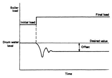
Figure 15.30 System response to proportional controller action
