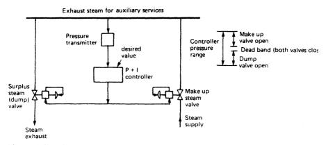
Figure 15.37 Exhaust steam pressure control
