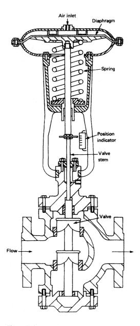
Figure 15.34 Pneumatically controlled valve
