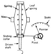
Figure 15.15 Mechanical tachometer
