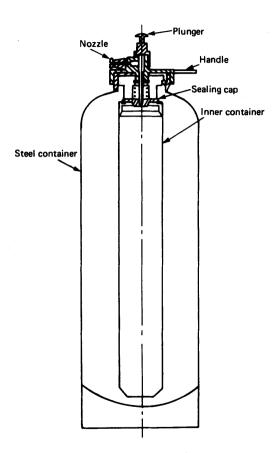
Figure 13.5(a) Foam fire extinguishers—chemical foam
