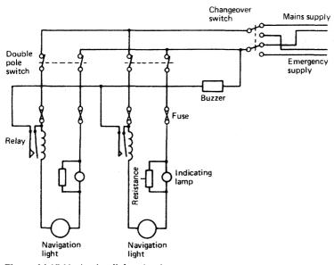
Figure 14.15 Navigation lights circuit
