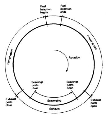
Figure 2.4 Two-stroke timing diagram
