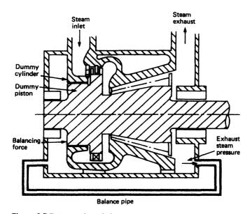
Figure 3.7 Dummy piston balance arrangement
