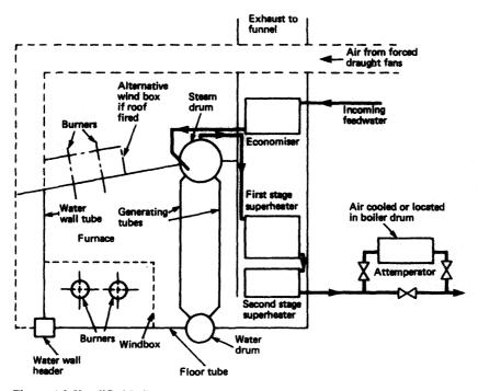
Figure 4.1 Simplified boiler arrangement
