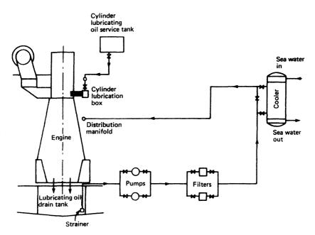
Figure 2.17 Lubricating oil system
