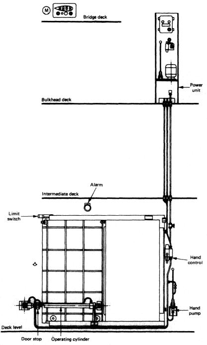
Figure 10.9 Horizontal sliding watertight door
