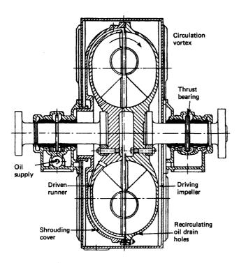
Figure 2.25 Hydraulic coupling
