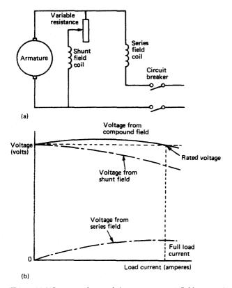
Figure 14.1 Compound wound d.c. generator, (a) field connection; (b) characteristic curves
