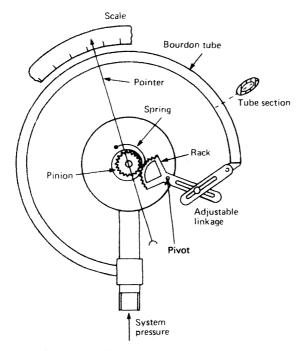
Figure 15.4 Bourdon tube pressure gauge
