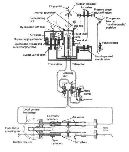
Figure 12.4 Telemotor control system
