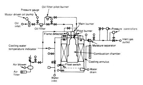
Figure 13.13 Inert gas generator
