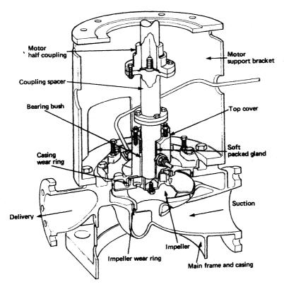
Figure 6.7 Single-entry centrifugal pump
