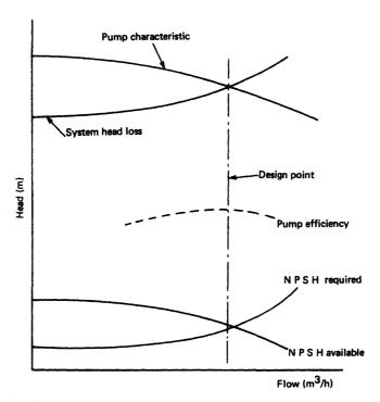
Figure 6.2 Overall pump system characteristics
