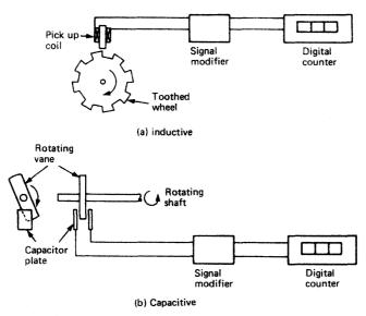
Figure 15.17 Pick-up tachometers, (a) inductive; (b) capacitive
