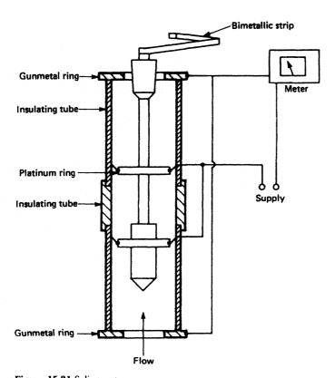
Figure 15.21 Salinometer
