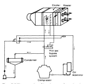
Figure 9.12 Direct-expansion refrigeration system for an air cooler
