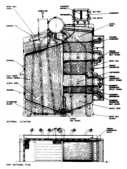
Figure 4.5 Foster Wheeler radiant-type boiler
