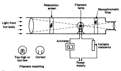
Figure 15.9 Optical pyrometer
