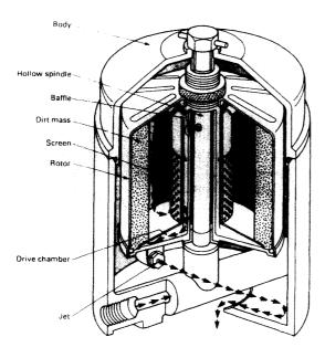
Figure 8.6 Centrifugal filter
