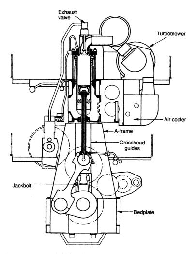
Figure 2.28 Sulzer RTA72U engine
