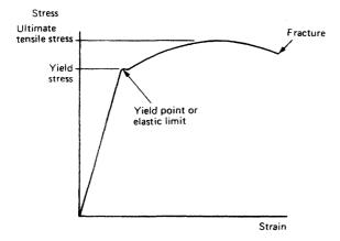
Figure 16.1 Stress strain curve
