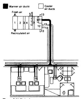
Figure 9.11 Twin-duct system
