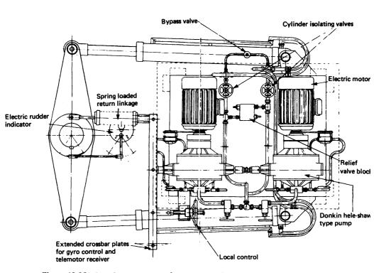
Figure 12.6(b) Actual arrangement of two-ram steering gear
