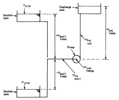
Figure 6.1 Basic pumping system
