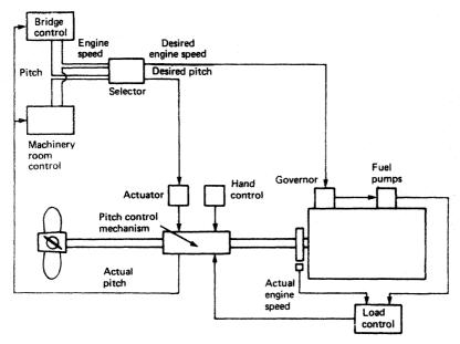
Figure 15.45 Bridge control of controllable-pitch propeller
