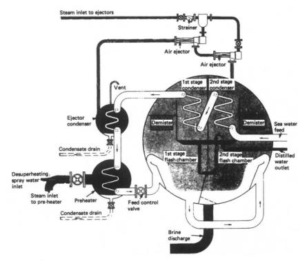
Figure 7.7 Two-stage flash evaporator
