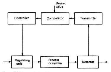
Figure 15.24 Automatic closed loop control
