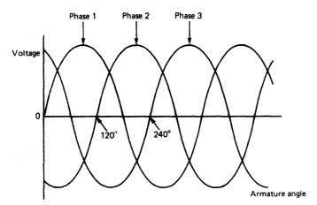
Figure 14.5 Three-phase alternator output
