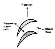
Figure 3.3 Reaction blading
