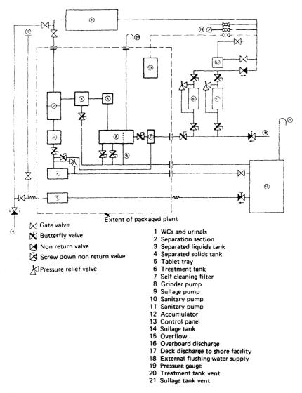
Figure 7.9 Chemical sewage treatment plant
