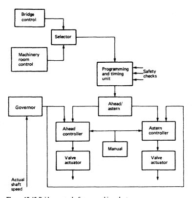
Figure 15.43 Bridge control of steam turbine plant
