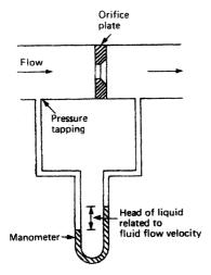
Figure 15.13 Orifice plate
