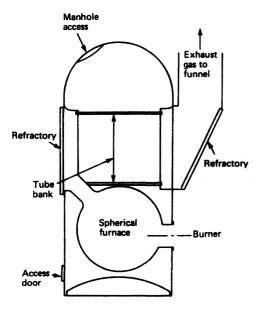
Figure 4.8 Cochran spheroid boiler
