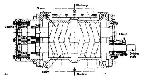
Figure 6.4 Rotary displacement pumps: (a) rotary vane displacement pump, (b) screw displacement pump
