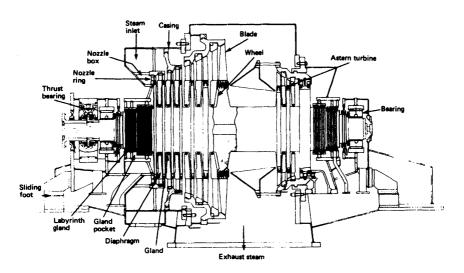
Figure 3.5 Impulse turbine
