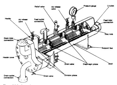
Figure 5.8 Drains cooler
