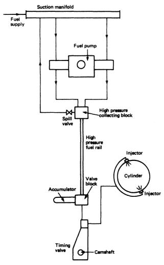
Figure 2.14 Common rail fuel injection system
