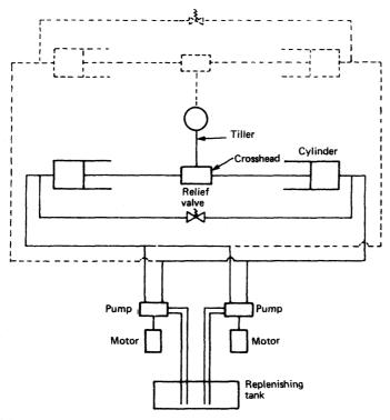
Figure 12.6(a) Diagrammatic arrangement of two-ram steering gear (additional items for four-ram system shown dotted)
