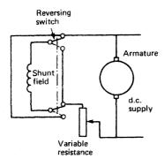
Figure 14.9 Shunt wound d.c. motor
