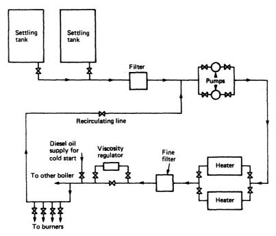
Figure 4.15 Boiler fuel-oil supply system
