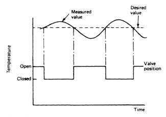
Figure 15.29 Two-step or on-off control
