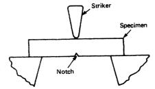
Figure 16.3 Impact test
