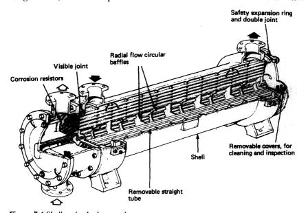
Figure 7.4 Shell and tube heat exchanger
