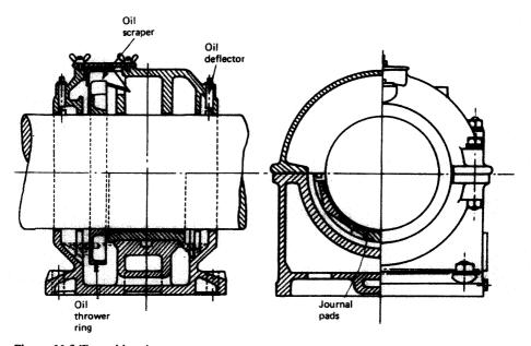
Figure 11.3 Tunnel bearing
