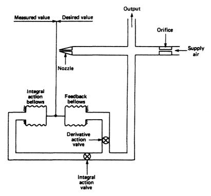
Figure 15.32 Pneumatic three-term controller
