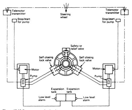
Figure 12.12 Rotary-vane twin circuit system
