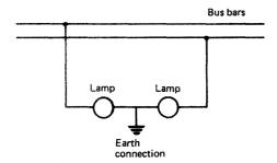
Figure 14.3 Earth lamp circuit
