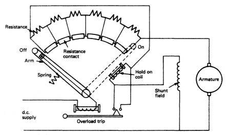
Figure 14.11 D.C. motor starter
