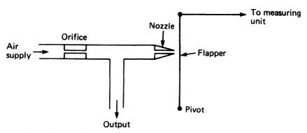
Figure 15.25 Position balance transmitter
