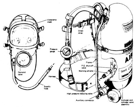
Figure 13.16 Self-contained breathing apparatus
