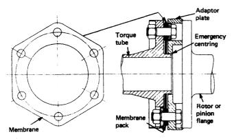
Figure 3.15 Flexible coupling
