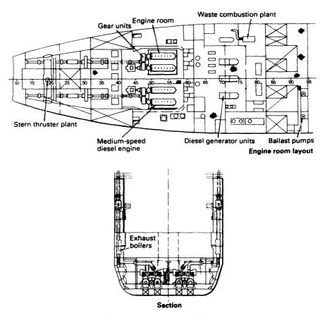
Figure 1.3 Medium-speed diesel machinery arrangement
