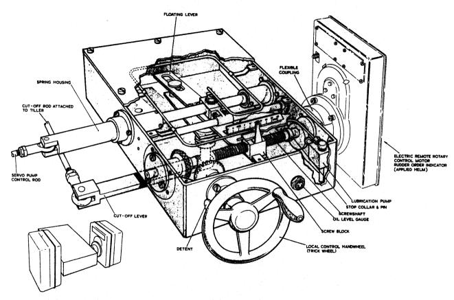
Figure 12.5(b) Arrangement of control box
