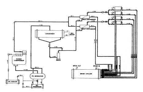
Figure 9.7 Central refrigerating plant
