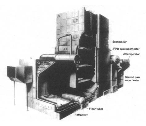
Figure 4.3 Foster Wheeler Type ESD I boiler
