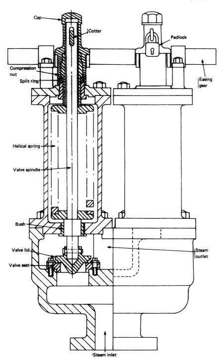
Figure 4.13 Ordinary spring-loaded safety valve
