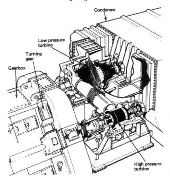
Figure 3.4 Cross compound turbine arrangement
