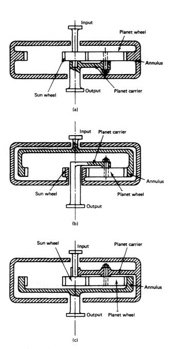
Figure 3.12 Epicyclic gearing; (a) planetary gear, (b) solar gear, (c) star gear
