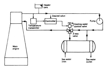
Figure 15.41 Cooling water temperature control
