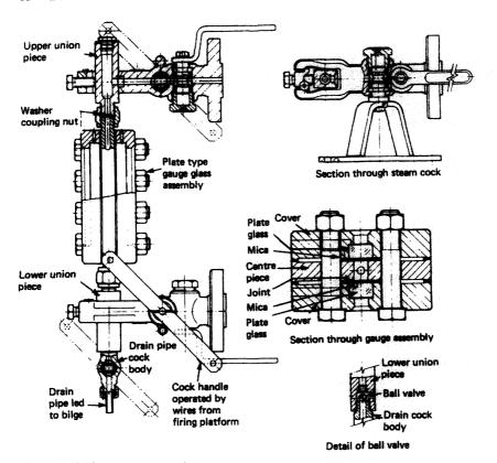
Figure 4.12 Plate-type gauge glass
