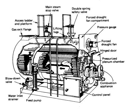
Figure 4.7 Package boiler
