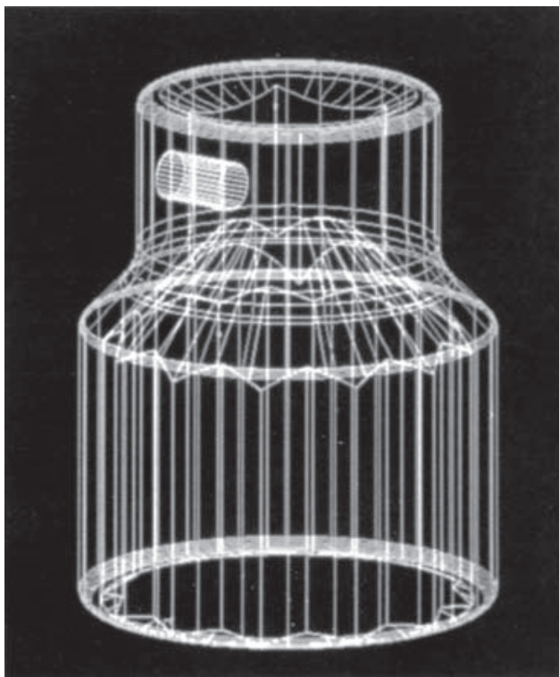
Fig. 3.17 BS4006 gives the dimensions, testing and design requirements for hand-operated square drive socket wrenches and accessories. The tools are manufactured from chrome vanadium steel and these illustrations show typical production drawings and presentations for sales brochures.
