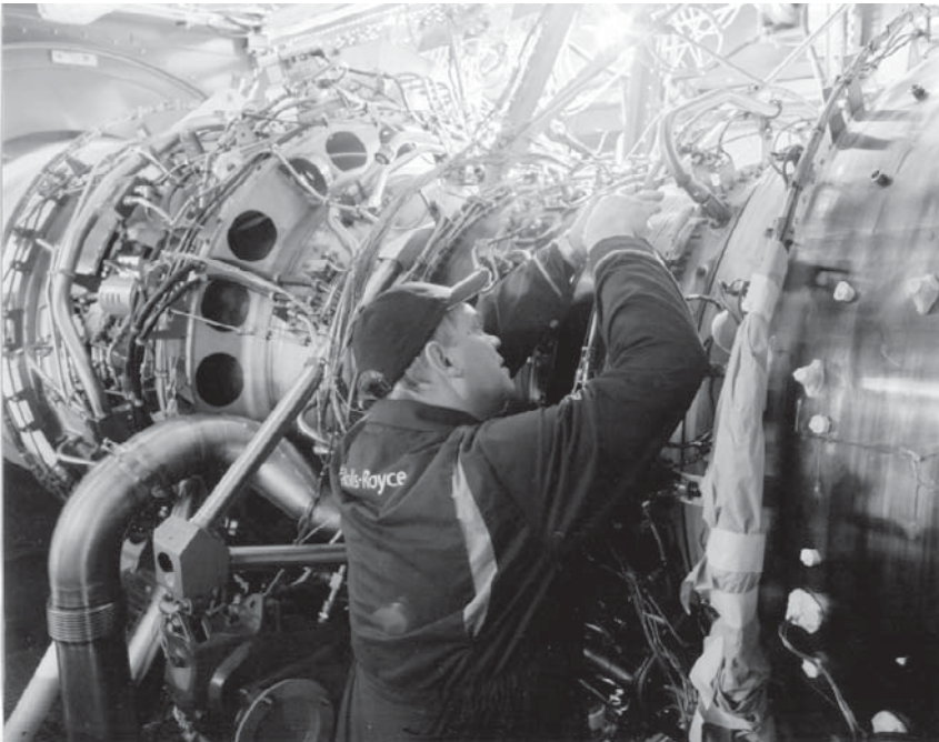
Figure 31.25 Routine maintenance of the Rolls-Royce MT30 gas turbine (shown here on the testbed) is limited to checking fluid levels and visual examinations
