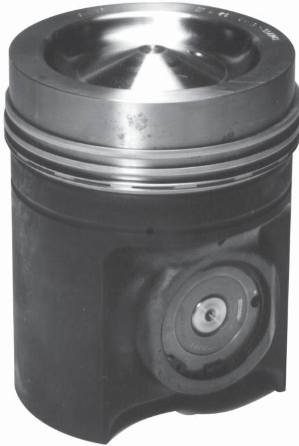
Figure 27.12 Wärtsilä 20 engine composite piston with nodular cast iron pressure-lubricated skirt and steel crown
