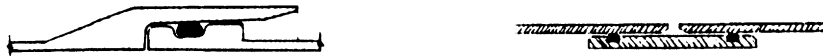
FIGURE 25.2: Bell-and-spigot and coupling joints for fiberglass pipe. (From American Society for Testing and Materials. 1991. D3517. Standard Specification for "Fiberglass" Glass-Fiber-Reinforced Thermosetting-Resin Pressure Pipe . With permission.)
