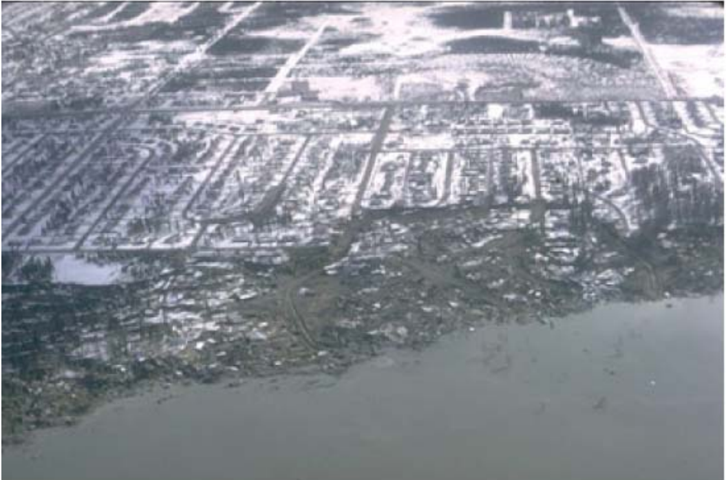
FIGURE 30.17 Aerial view of Turnagain Heights slide. (Courtesy of the Steinbrugge Collection, Earthquake Engineering Research Center, University of California, Berkeley.)
