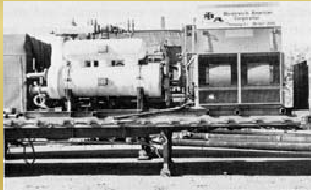
Portable twin 60-ton brine refrigeration unit
