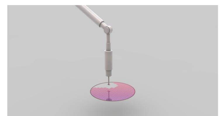
Discarding faulty Dies The dies that responded with the right answer to the test pattern will be put forward for the next step (packaging).
