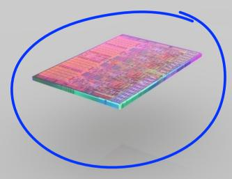
Individual Die This is an individual die which has been cut out in the previous step (slicing).
