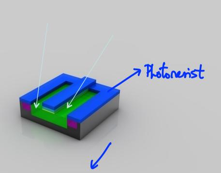
Applying Photo Resist (for Doping or Ion Implantation) There's photo resist (blue color) applied, exposed and exposed photo resist is being washed off before the next step. The photo resist will protect material that should not get ions implanted.
