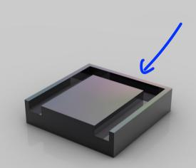
Removing Photo Resist After the etching the photo resist is removed and the desired shape becomes visible.
