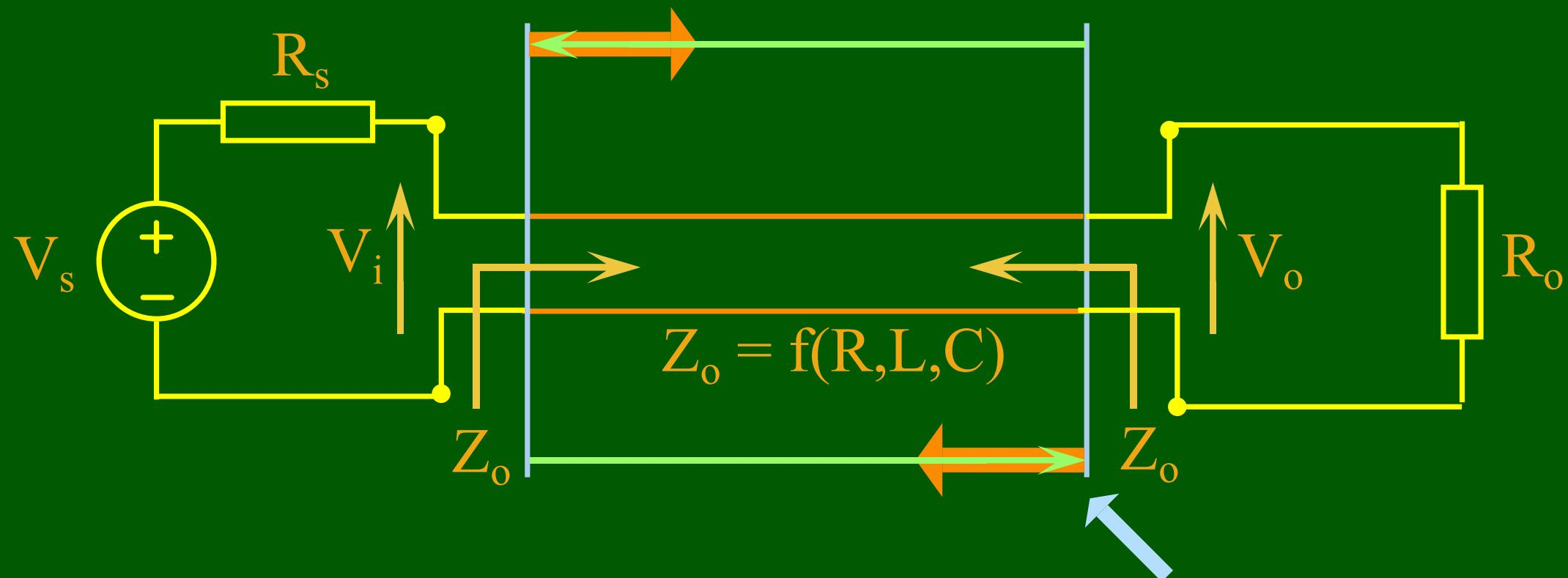
$$\rho_o = \left( \frac{R_o - Z_o}{R_o + Z_o} \right) \text{Coefficient of reflection}$$
