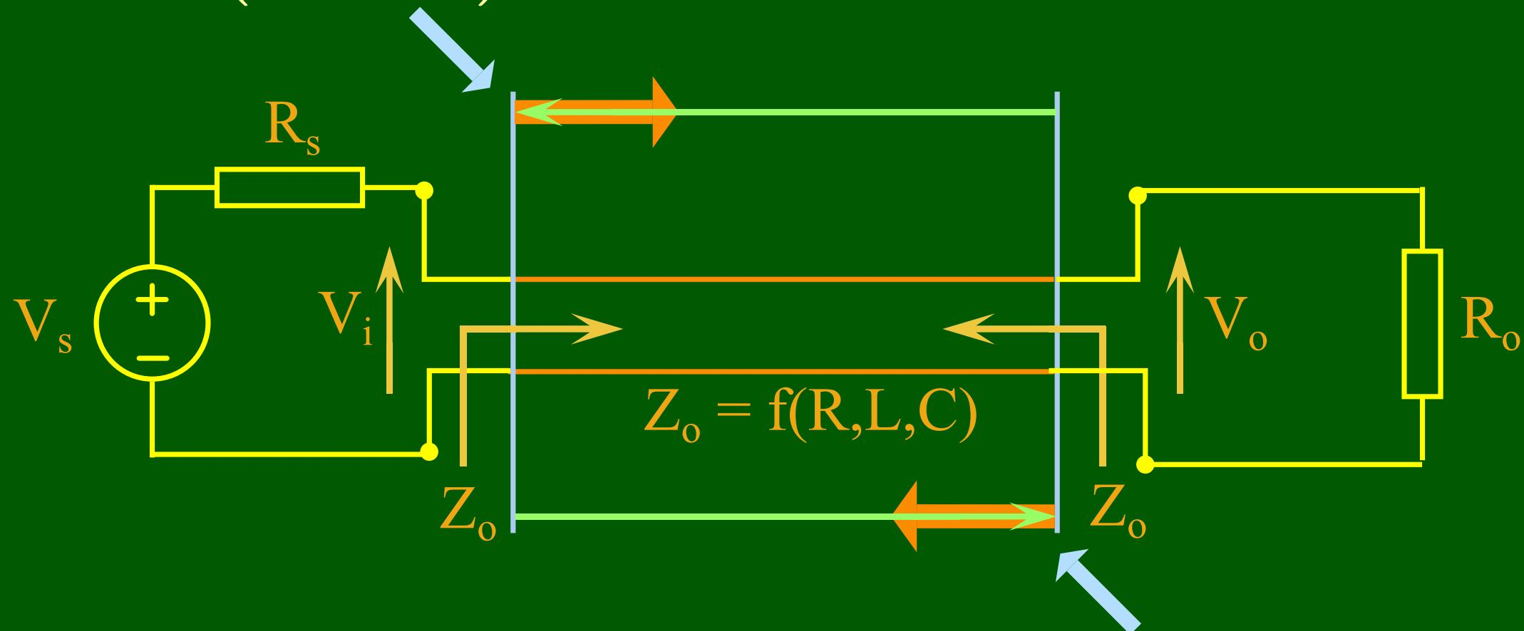
$$\rho_o = \left( \frac{R_o - Z_o}{R_o + Z_o} \right) \text{ Coefficient of reflection}$$
