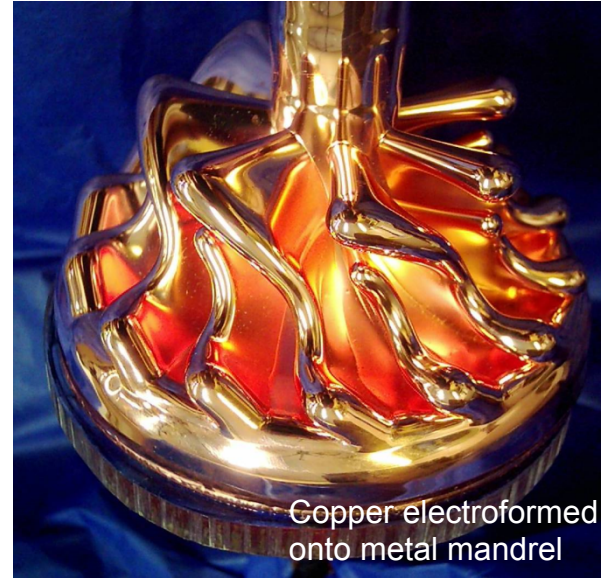
An example of mandrel used in electroforming
