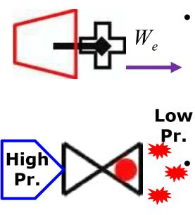
The heat exchangers are used to conserve cold and J – T devices are used to achieve lower temperatures.
