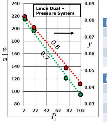
**Liquid yield v/s. i** • The Plot for **y** versus **i** for different pressures is as shown.
