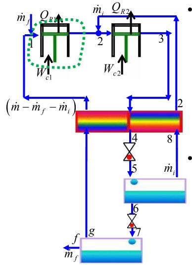
For the work requirement, consider a control volume for the compressor – **1** as shown in the figure.
