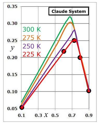
**Liquid yield v/s. x** • However,  $T_3$  is limited by the position of the point **e** on the T – s diagram.
