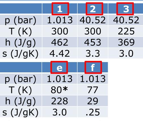
The point e is located on p=1bar isobar by drawing a vertical line from point 3.
