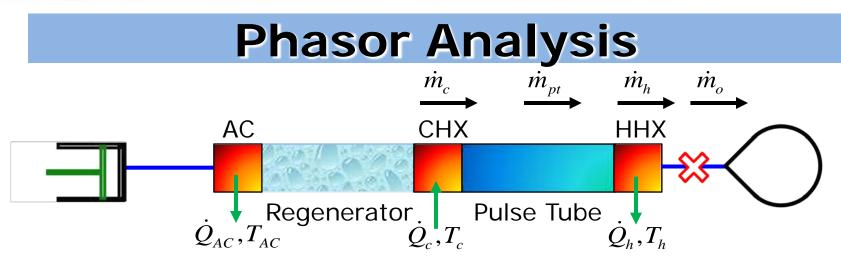
The mass flow rate through the orifice is directly proportional to the pressure drop.
