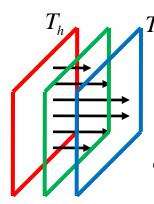
$$k_{A} = \Delta x \left( \sigma \left( T_{h}^{2} + T_{c}^{2} \right) \left( T_{h} + T_{c} \right) \left( \frac{e}{2 - e} \right) + h_{c} \right)$$
