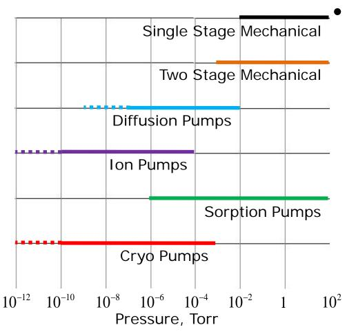
The adjacent figure shows the operating range for different vacuum pumps.
