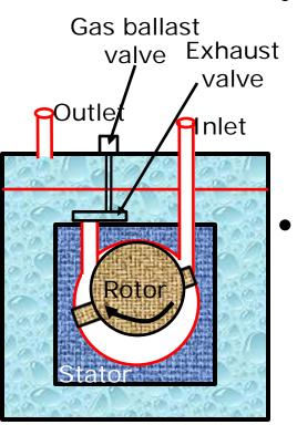
It is important to note that, there is a possibility of condensation of some gases, say water vapor, during the compression process.
