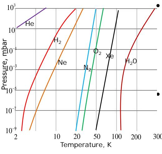
The adjacent figure shows the variation of equilibrium vapor pressure with temperature for different gases.
