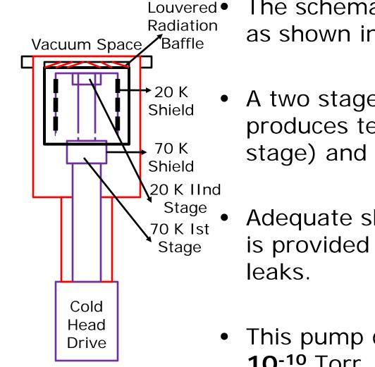
The schematic of a Cryo pump is as shown in the figure.
