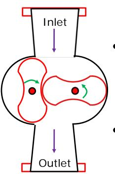
A backing pressure is necessary on the outlet side before the operation of the pump.
