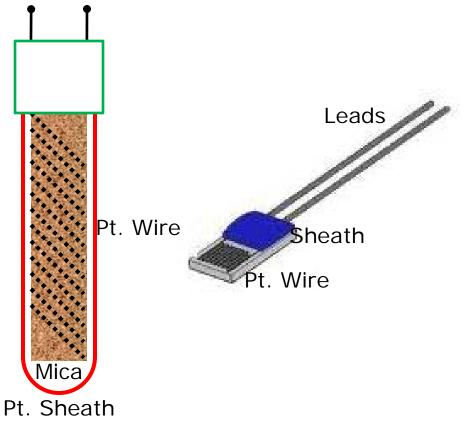
The typical size of a RTD is 3 mm x 1.84 mm x 0.98 mm.
