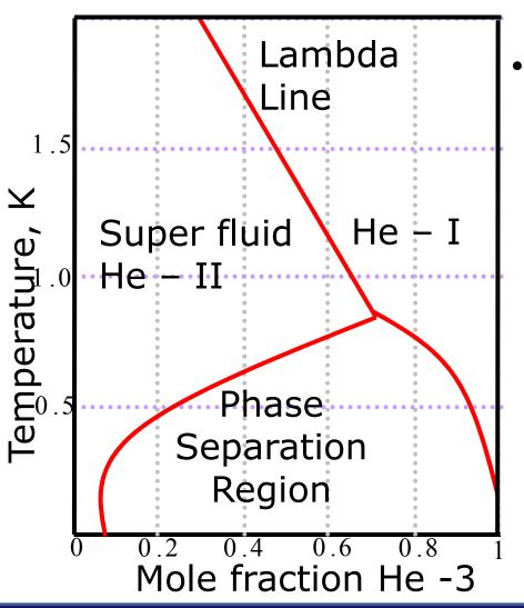
This separation into two liquid phases and difference in vapor pressure forms the basis for Dilution Refrigerator.
