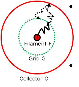
However, a few of the electrons move beyond the grid, due to porosity of the grid and high velocity of electrons.
