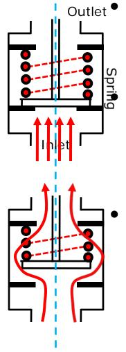
The process of releasing excess pressure is called as Blow Down.
