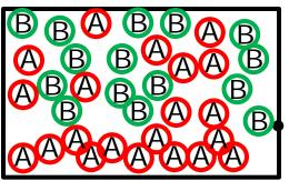
The low temperature heavier gas (**N**<sub>2</sub>, **A**) displaces air, and thereby oxygen, in the nearby spaces.
