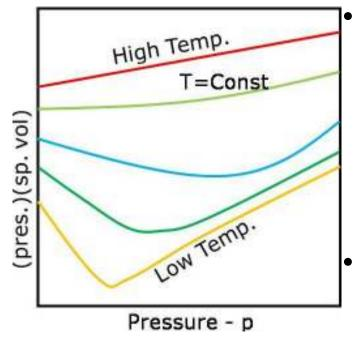
The second term is negative at low pressures and low temperatures, where the gases are more compressible than the Boyle's law.
