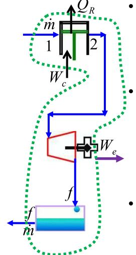
Since in an ideal system, mass of gas compressed is same as mass of gas liquefied,  $m_1 = m_f$ .
