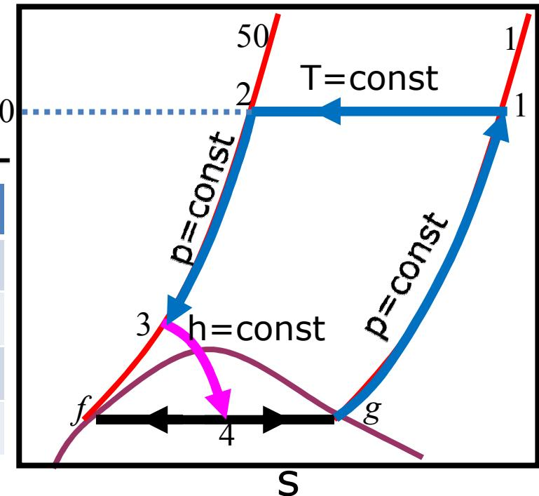
$$y_I = \left( \frac{h_1 - h_2}{h_1 - h_f} \right) = \left( \frac{464 - 454}{464 - 35} \right) = \left( \frac{10}{429} \right) = 0.023$$
