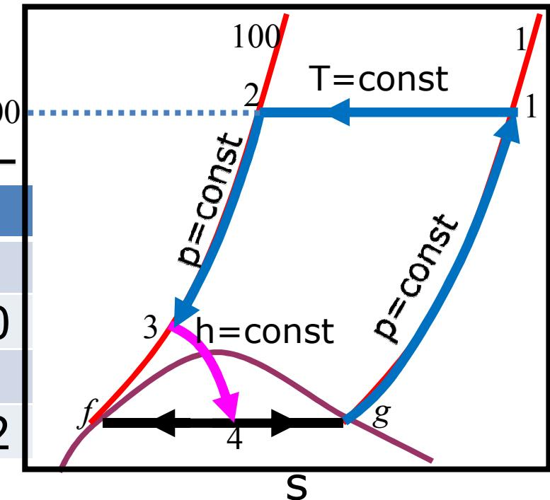
$$y_{III} = \left( \frac{h_1 - h_2}{h_1 - h_f} \right) = \left( \frac{464 - 445}{464 - 35} \right) = \left( \frac{19}{429} \right) = 0.044$$
