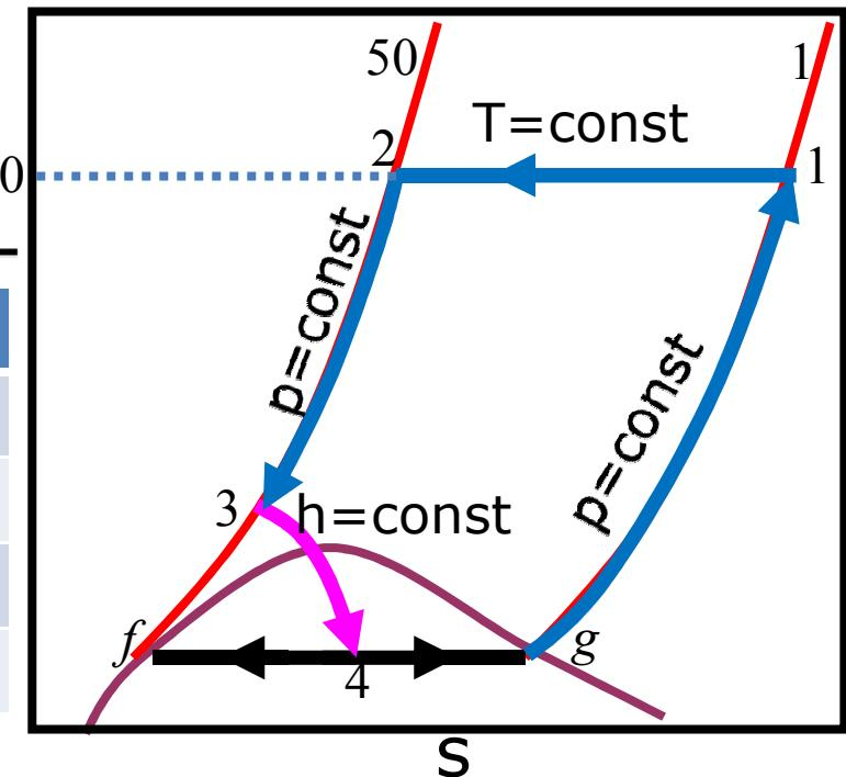
$$y_{II} = \left( \frac{h_1 - h_2}{h_1 - h_f} \right) = \left( \frac{357 - 332}{357 - 35} \right) = \left( \frac{25}{325} \right) = 0.076$$
