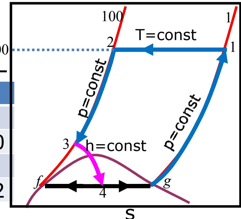
$$y_{IV} = \left( \frac{h_1 - h_2}{h_1 - h_f} \right) = \left( \frac{357 - 312}{357 - 35} \right) = \left( \frac{45}{322} \right) = 0.14$$
