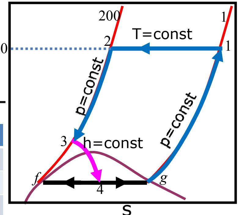
$$y = \left( \frac{h_1 - h_2}{h_1 - h_f} \right) = \left( \frac{28.47 + 8.37}{28.47 + 406} \right) = \left( \frac{36.84}{434.47} \right) = 0.085$$
