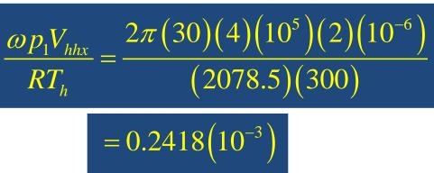
Mass flow rate in Compressor (kg/s).
