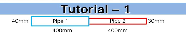
Calculate the overall conductance of the pipe assembly shown above. The pressure on the right end of the 40 mm tube is 150 mPa, while the pressure on the left end of 30mm pipe is 10 mPa. The ambient temperature is 300 K. The molecular weight and viscosity of air are 28.95 g/mol and 18.47 µPa-s.
