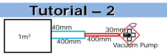
Consider a vacuum vessel of 1m<sup>3</sup> with an initial pressure of 1 atm at 300 K. It is connected to a vacuum pump via a connecting pipe as shown above. The ultimate pressure of the system is 0.1 mPa. Determine the system pumping speed, if the required vacuum in the cavity is 1 kPa in 1 hour.
