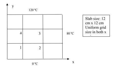
(5) Two dimensional, steady state conduction in a square slab with k = 40 W/mK and an internal heat generation of  $q_v = 6 \times 10^5$  W/m<sup>3</sup> is to be numerically simulated. The details are given in the figure. For simplicity the number of grid points is intentionally kept small for this problem.
