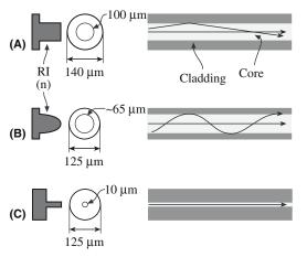
FIGURE 32.15 Total internal reflection (TIR) along an optical fiber. (a) Step index fiber; (b) graded index fiber; (c) single mode fiber. The plot on the left is a variation of RI (= n).
