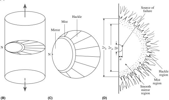
*Mirror*: The region around the crack origin. The crack travels in a single plane accelerating as it goes. The fracture surface is smooth and highly reflective. This can be seen in polycrystalline ceramics, but reflectivity is lower.
