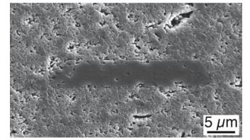
FIGURE 15.9 Templating grain growth. The seed is the elongated grain in the center.
