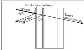
FIGURE 26.13 Illustration of approaches for solar protective double glazing with absorbing and reflecting panes.
