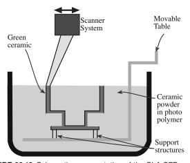
FIGURE 23.13 Schematic representation of the SLA SFF process.
