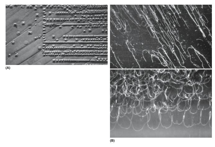
**FIGURE 17.4** (a) Glide bands in LiF revealed by etching. (b) "Glide" bands in spinel: (top) 200°C; (bottom) 950°C.
