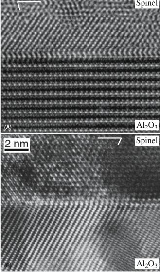
FIGURE 15.2 HRTEM images of crystallographically two different spinel/Al<sub>2</sub>O<sub>3</sub> PBs (a and b). White lines show the {111} planes in the spinel.
