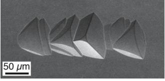
FIGURE 12.9 Etch pits at dislocations emerging at a surface in Si. (a) The cross-sectional view in Si; (b) the plan view in YAG.
