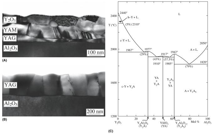
FIGURE 25.21 Forming YAG by a thin-film reaction: (a) intermediate state; (b) final state for the same film; (c) the equilibrium phase diagram.
