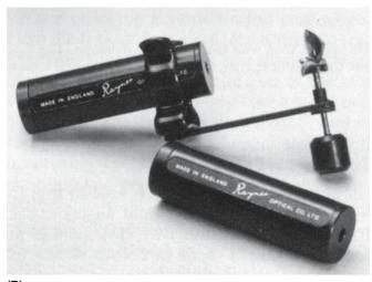
FIGURE 36.12 A dichroscope for estimating the dichroism of a stone and the optics on which it is based.
