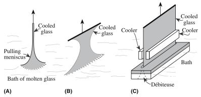
**FIGURE 26.7** Principle of drawing from molten glass: (a) a circular rod; (b) problem of pulling a planar sheet; (c) use of a débiteuse and cooling to allow the formation of a sheet of constant width.
