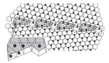
FIGURE 14.17 Schematic of a GB in Al<sub>2</sub>O<sub>3</sub> showing the creation of new polyhedra in the GB. The inset shows a tilted view of the repeating group of polyhedra.
