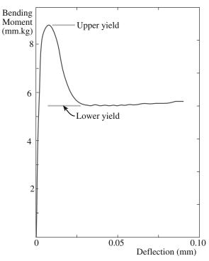
FIGURE 17.2 Stress-strain curve for a LiF single crystal.
