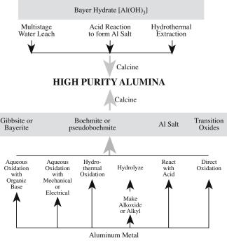
FIGURE 19.6 High-purity alumina production routes.
