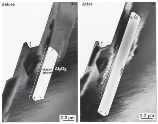
**FIGURE 15.7** Glass "particles" in a thin film of  $\alpha$ -Al<sub>2</sub>O<sub>3</sub> before and after additional heat treatment.
