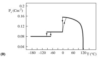
FIGURE 31.14 (a) Dielectric constant and (b) spontaneous polarization of single-crystal BaTiO<sub>3</sub> as a function of T. (Compare to Figure 31.9.)
