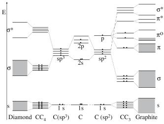
FIGURE 4.17 Energy level diagram for diamond and graphite.
