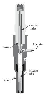
FIGURE 23.16 Schematic of the abrasive waterjet cutting process.
