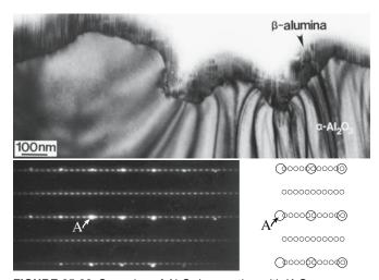
FIGURE 25.22 Corrosion of Al<sub>2</sub>O<sub>3</sub> by reaction with K<sub>2</sub>O vapor showing a TEM image, the DP, and a schematic of the DP.
