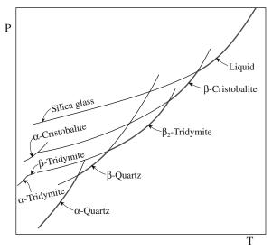
FIGURE 8.8 The SiO<sub>2</sub> phase diagram.
