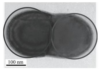
FIGURE 24.7 Two Si spheres partly sintered (TEM image).
