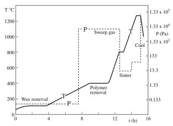
FIGURE 23.15 Pressure-induced binder removal cycle.
