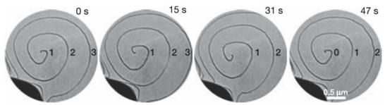
FIGURE 12.24 Dislocation in TiN intersecting the surface causing a spiraling step.
