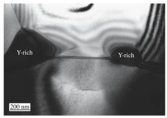
**FIGURE 1.4** TEM image of grain boundaries in AIN showing yttria-rich second-phase particles at the triple junctions.
