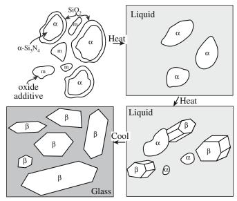
**FIGURE 37.1** Schematic showing processing steps in forming  $Si_3N_4$  by liquid phase sintering (LPS). The metal oxide additive (m) would be something like  $Y_2O_3$  and the liquid an oxynitride/silicate.
