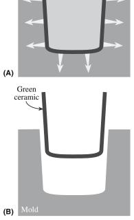
**FIGURE 23.9** Schematic illustrating the drain-casting process. (a) Fill the mold with slip; the mold extracts liquid, forming a compact along the mold walls; (b) after excess slip is drained and after partially dryed, green ceramic is removed.
