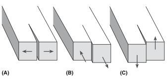
**FIGURE 16.6** The three deformation modes for fracture: (a) Mode I opening. (b) Mode II sliding (in-plane shearing). (c) Mode III tearing (antiplane shearing).
