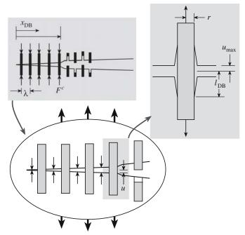
FIGURE 18.19 Illustration of a crack bridging mechanism with debonding and fiber pullout.
