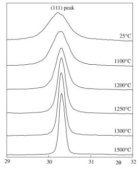
FIGURE 20.14 Illustration of X-ray line broadening for a ZrO<sub>2</sub>/3 mol% Y<sub>2</sub>O<sub>3</sub> powder prepared by hydrothermal synthesis.
