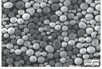
FIGURE 35.8 Lithium calcium borate glass microspheres produced by passing through a flame at 1400°C.
