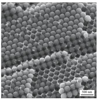
FIGURE 36.23 SEM image of a Gilson opal.
