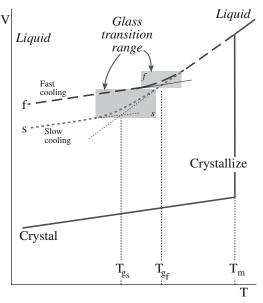
**FIGURE 21.1** Plot of volume versus temperature for a liquid that forms a glass on cooling and one that forms a crystalline solid. The glass transition temperature,  $T_{\rm g}$ , depends on the cooling rate and is not fixed like  $T_{\rm m}$ .
