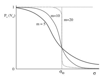
FIGURE 16.21 Illustration of the effect of m on survival probability. When m changes  $P_S$  changes.
