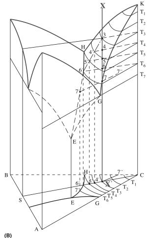
**FIGURE 8.15** (a) A model ternary phase diagram for a system showing three solid solutions. (b) A model ternary phase diagram for a system showing three eutectics.
