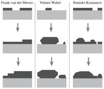
FIGURE 13.14 The three modes of thin-film growth.
