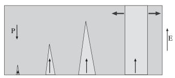
FIGURE 31.11 Illustration of the growth of a ferroelectric domain in a field ξ.
