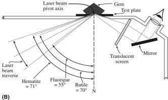
FIGURE 36.6 (a) Portable jeweler's refractometer for measuring the critical angle; (b) the optics of determining the critical angle using the refractometer.
