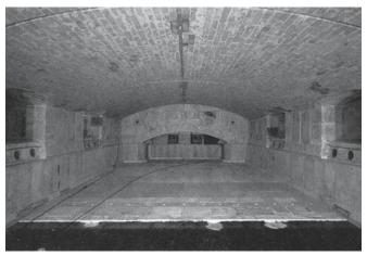
FIGURE 26.2 Inside a typical glass melting tank.
