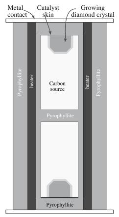
FIGURE 29.16 Chamber for diamond growth.
