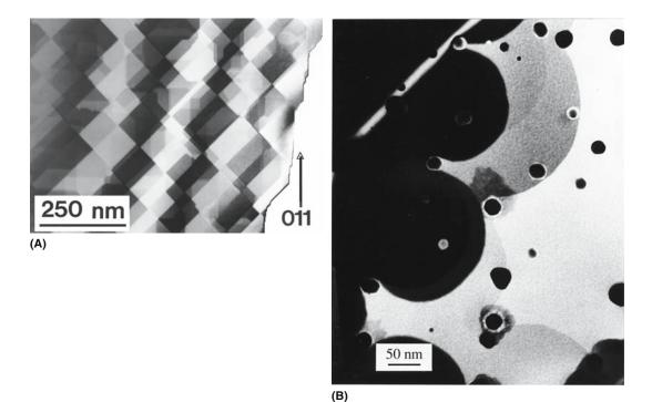
**FIGURE 13.20** Plan view TEM images of steps on  $MgAl_2O_4$  and  $Al_2O_3$ ; the steps occur when the thickness of the TEM sample changes abruptly.
