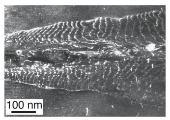
FIGURE 25.6 Movement of interfacial dislocations between hematite and NiFe<sub>2</sub>O<sub>4</sub> spinel during oxidation leading to thickening of the precipitate.
