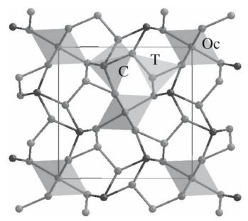
**FIGURE 7.13** The crystal structure of mullite viewed along the short *z*-axis ( $a = 0.76\,\mathrm{nm},\ b = 0.77\,\mathrm{nm},\ c = 0.29\,\mathrm{nm}$ ). The sites Oc and T are never fully occupied so this is an idealized schematic of this orthorhombic orthosilicate. The chains of octahedra at the corners and center lie along *z*.
