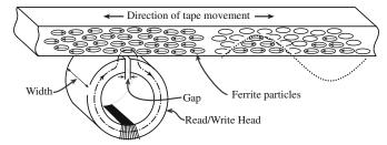
FIGURE 33.25 Illustration of the principal features of longitudinal recording.
