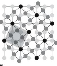
**FIGURE 14.1** Schematics of two low- $\Sigma$  GBs. (a)  $\Sigma = 3$ ; (b)  $\Sigma = 5$ .
