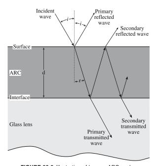
FIGURE 32.8 Illustration of how an ARC works.
