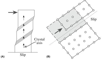
FIGURE 17.3 Illustration of slip bands: (a) macroscopic appearance; (b) showing atomic movements.
