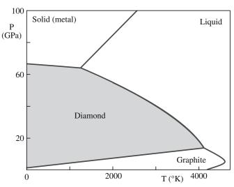
FIGURE 8.7 The C phase diagram.
