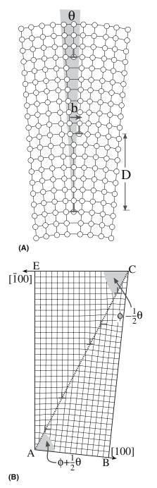
FIGURE 14.6 Schematics of low-angle tilt GBs. (a) Symmetric; (b) asymmetric.
