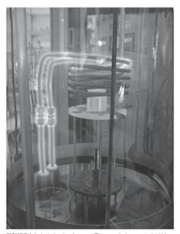
**FIGURE 9.6** An induction furnace. The sample is mounted within the coils, which are usually water-cooled copper.
