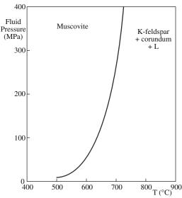
**FIGURE 19.4** Pressure–temperature phase relations for the bulk composition  $K_2O \cdot 3Al_2O_3 \cdot 6SiO_2 - 2H_2O$ .
