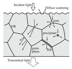
**FIGURE 32.10** Mechanisms for loss of transparency due to scattering. GB, grain boundary; IGF, intergranular film. Details of the individual defects are described in Chapters 12–15.
