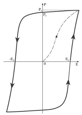
FIGURE 31.3 Hysteresis curve for a typical ferroelectric.
