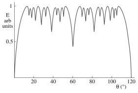
FIGURE 14.4 Cusp in a plot of GB energy versus misorientation angle, θ.
