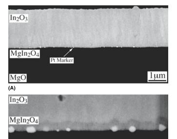
FIGURE 25.14 SEM backscattered electron images of an asdeposited In<sub>2</sub>O<sub>3</sub> film on MgO with Pt markers.
