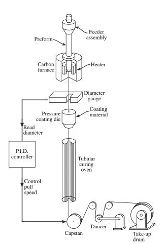
FIGURE 32.17 The fiber drawing tower.
