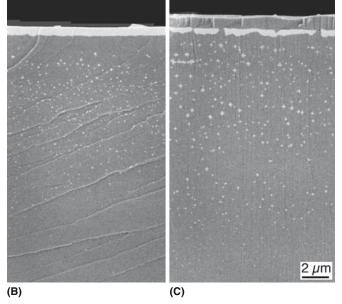
FIGURE 25.23 Reaction between a thin film of Fe<sub>2</sub>O<sub>3</sub> and a layer of MgO in an electric field at 1150°C for 2 hours: (a) schematic of the set up; (b) no applied field; (c) 2kV/cm applied field. The MgO has grown on top of the spinel. The reaction is fastest at GBs in the thin film.
