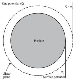
**FIGURE 27.12** Illustration of the  $\zeta$  potential and the effective size of a charged particle.
