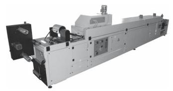
FIGURE 27.4 Example of an industrial tape casting machine.
