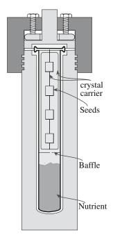
$\begin{tabular}{ll} \textbf{FIGURE 29.11} & A silver-lined laboratory hydrothermal autoclave, \\ about 35\,cm \ long. \ It can be much longer. \\ \end{tabular}$
