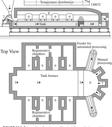
FIGURE 26.3 Schematics of a glass melting tank for producing containers.
