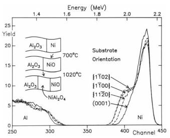
**FIGURE 10.29** RBS data sets obtained using a 2.8-MeV beam of He<sup>2+</sup> ions with the samples tilted 45°. Each sample has been annealed at 700°C for 2 hours followed by 1020°C for 5 hours; the Ni peak shows that the extent of the reaction varies with the surface orientation.
