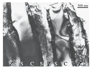
FIGURE 15.18 A CoO/ZrO2 eutectic after solidification and subsequent oxidation. Z, ZrO<sub>2</sub>; C, CoO; S, Co<sub>3</sub>O<sub>4</sub> (spinel).
