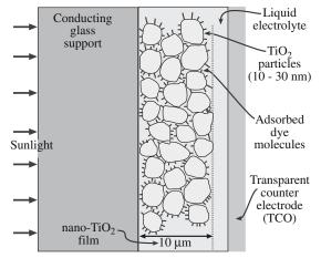
FIGURE 37.11 Schematic of a dye-sensitized nanocrystalline solar cell.
