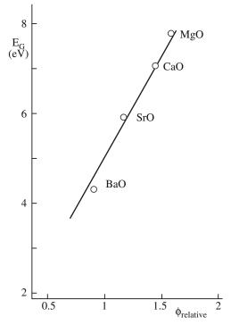
**FIGURE 30.24** Effect of bond ionicity on  $E_{\alpha}$  for metal oxides MO  $(\phi = Z/r)$ .
