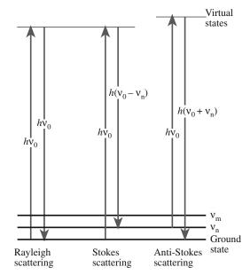
FIGURE 10.19 Schematic of transitions occurring in Raman spectroscopy.
