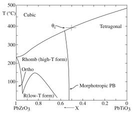
FIGURE 31.20 The PZT phase diagram.
