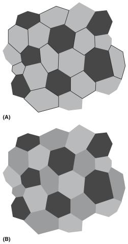
FIGURE 24.26 Schematics of multiphase ceramics; (a) two phases and (b) three phases.
