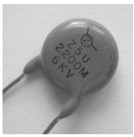
FIGURE 31.17 Ceramic disc capacitor.
