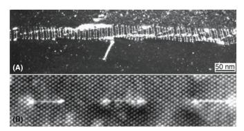
**FIGURE 14.12** A low-angle tilt GB in spinel showing an array of climb-dissociated edge dislocations. (a) The GB viewed at an angle; (b) at higher magnification, the dislocations viewed end-on.
