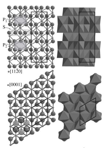
**FIGURE 6.12** The sapphire crystal structure. (Top) [ $11\bar{2}0$ ] view; (bottom) [0001] view; (left) atomic models; (right) stacking octahedra. P<sub>1</sub> and P<sub>2</sub> are two unoccupied octahedra. S is a triangle of more closely spaced O<sup>2-</sup> ions. Open circles in the lower left show the AB stacking of the anions. The unit cell is outlined for both projections.
