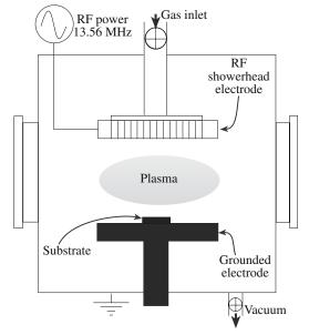
FIGURE 20.9 Schematic of a plasma reactor.
