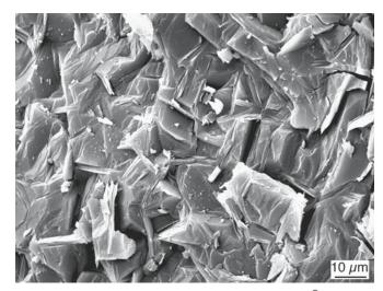
FIGURE 18.23 The fracture surface of Macor®.
