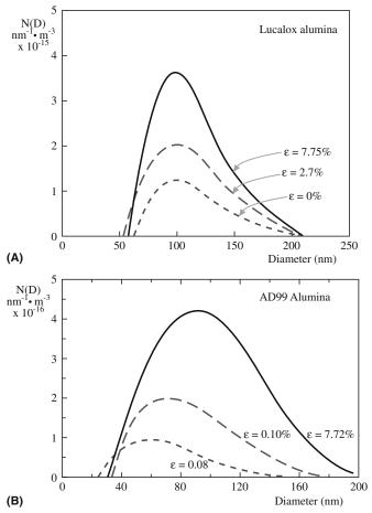
**FIGURE 17.18** (a) Cavity-size distribution as a function of creep strain in alumina without a glassy phase (Lucalox). (b) Cavity-size distribution as a function of creep strain in alumina with a glassy phase (AD99).
