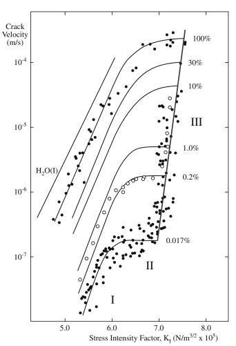
**FIGURE 18.9** Crack velocity in soda-lime glass as a function of  $K_{l}$ , the stress intensity factor. The percentages indicate the relative humidity and the Roman numerals indicate the three regions of crack propagation.
