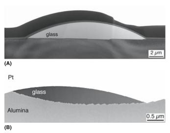
FIGURE 13.11 Experimental observations of glass droplets on the surface of Al<sub>2</sub>O<sub>3</sub>: (a) c plane, (b) m plane.
