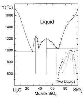
**FIGURE 21.6** Region of liquid–liquid immiscibility for SiO<sub>2</sub>–Li<sub>2</sub>O. Notice that these occur only in the silica-rich end of the phase diagram.
