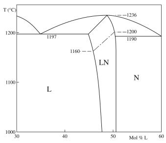
FIGURE 29.10 Part of the Nb<sub>2</sub>O<sub>5</sub>-Li<sub>2</sub>O phase diagram.
