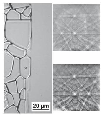
FIGURE 24.20 SEM image and two EBSD patterns from a series of engineered GBs in Al<sub>2</sub>O<sub>3</sub>. The upper DP is from point X and the lower is from the large grain on the left showing the basal-twin relationship.
