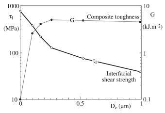
**FIGURE 20.16** Effect of carbon coating thickness ( $D_c$ ) on the mechanical properties of Nicalon<sup>TM</sup> fibers in an SiC matrix. Interfacial shear strength was measured by push-down testing and toughness from the area under the stress–strain curve during loading along the fiber axis.
