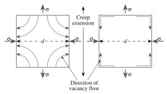
FIGURE 17.16 Illustration of Nabarro-Herring creep.
