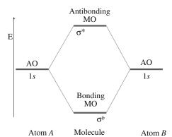
**FIGURE 4.11** Energy level diagram for the  $\rm H_2$  MOs and the corresponding AOs.
