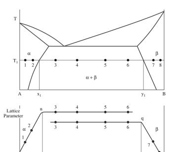
FIGURE 8.2 Parametric method for determination of the solvus lines in a binary phase diagram.
