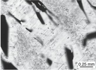
FIGURE 15.6 Particle in a matrix. (a) TEM image of a secondphase β-Al<sub>2</sub>O<sub>3</sub> growing along a GB in α-Al<sub>2</sub>O<sub>3</sub>. The insets show spinel (S) growing up the GBs. (b) VLM of rutile needles growing in a garnet grain.
