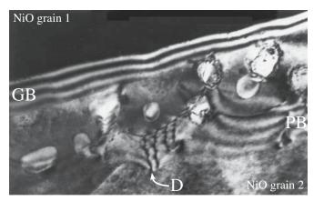
**FIGURE 15.10** Growth of a particle along a GB. The particle is topotactically aligned with one NiO grain (along PB at grain 2) but not the other (grain 1). D shows a dislocation at the coherent interface.
