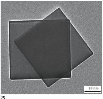
**FIGURE 14.3** Rotated MgO nanoparticles and their relation to  $\Sigma$ . The frequency of measuring a rotation  $\theta$  is  $f(\theta)$ .
