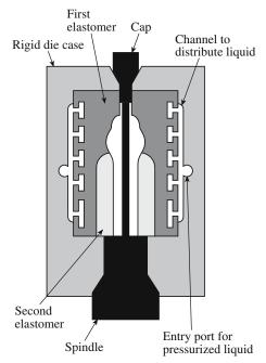
**FIGURE 23.4** Schematic of a die for dry-bag isostatic pressing of a spark plug insulator.
