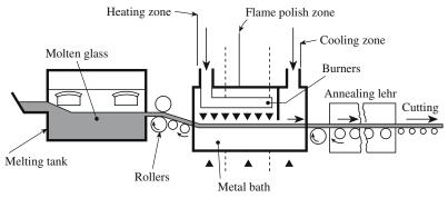
FIGURE 26.9 Schematic diagram of the float glass process.
