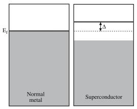
FIGURE 30.30 Band diagram for a superconductor.
