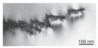
FIGURE 12.8 Diffraction contrast from dislocations in Al<sub>2</sub>O<sub>3</sub>.
