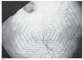
FIGURE 12.22 Schematic and IR image of a single-ended Frank-Read source in Si.
