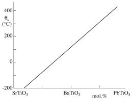
**FIGURE 31.16** Effect of substitution on  $\theta_c$  for BaTiO<sub>3</sub> solid solutions with SrTiO<sub>3</sub> and PbTiO<sub>3</sub>.
