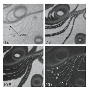
FIGURE 13.24 Studies of changes occurring at the surface of TiO2 using LEEM. A total of 20 seconds separates the four images. The different contrast occurs because of the surface reconstruction.
