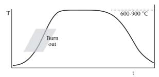
FIGURE 27.16 Typical thick film circuit firing profile.
