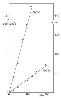
FIGURE 25.13 Kinetics of the reaction between bulk NiO and bulk Al<sub>2</sub>O<sub>3</sub> to form spinel.
