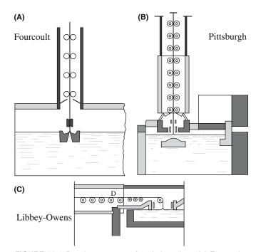
**FIGURE 26.8** Drawing processes for window glass. (a) Fourcault, (b) Pittsburgh, and (c) Libbey-Ownes.
