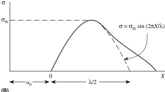
**FIGURE 18.2** (a) Model of a crack tip. The interplanar spacing is  $a_0$ . (b) Stress versus distance plot.
