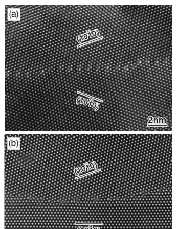
**FIGURE 14.16** HRTEM images of two high-angle GBs in ZnO: (a) near-symmetric; (b) asymmetric.
