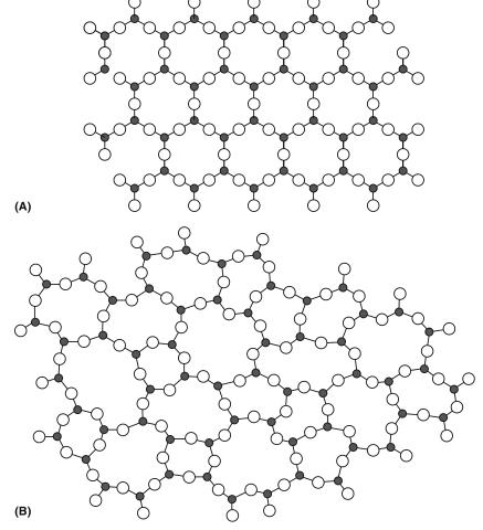
FIGURE 7.19 Comparing the structure of (a) crystalline silica and (b) glass.
