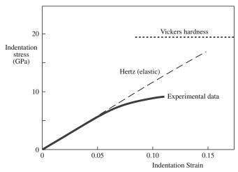
FIGURE 16.14 Indentation stress versus indentation strain.
