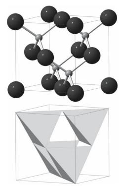
**FIGURE 6.4** The zinc-blende crystal structure. (Top) Ion positions; (bottom) corner-sharing tetrahedra.
