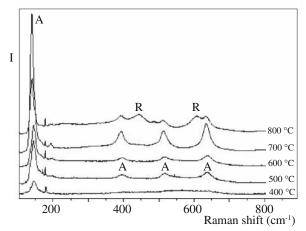
FIGURE 10.20 Example of Raman spectra from TiO2 films heated to different temperatures. R, rutile; A, anatase.
