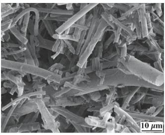
FIGURE 15.16 The porous material used to make insulating tiles for the space shuttle. The silica fibers are 2-4 µm in diameter.
