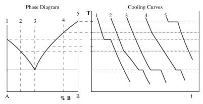
FIGURE 8.1 Illustration of the use of cooling curves to determine the liquidus and eutectic in a binary phase diagram.
