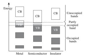
FIGURE 30.2 Schematic of electron energy bands in solids. The valence band (VB) and conduction band (CB) are indicated.
