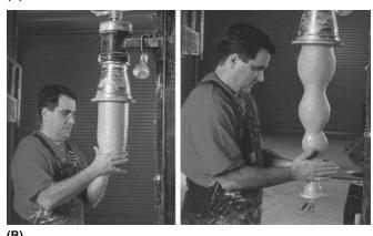
FIGURE 23.11 Extruding clay. Manual and electric extruders.
