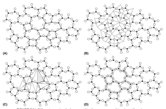
FIGURE 7.21 Different ways (a-d) of representing the same array of ions in a silica glass.
