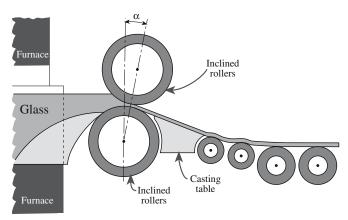
FIGURE 26.6 Continuous casting of flat glass.
