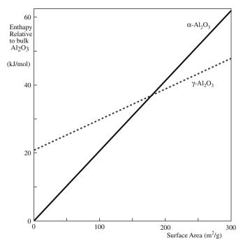
**FIGURE 5.11** Calculated enthalpy of alumina ( $\gamma$ - and  $\alpha$ -) polymorphs as it varies with the surface area. The calculation is an MD simulation using data for small surface areas. A large surface area per gm implies small particles.
