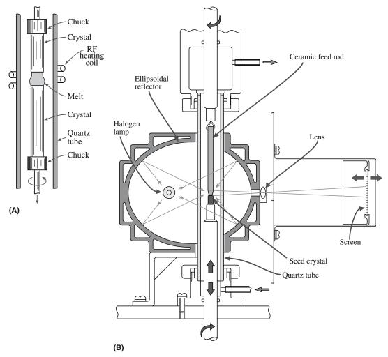
FIGURE 29.2 (a) Vertical float zone. (b) Arc image furnace.
