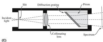
**FIGURE 36.8** (a) Photograph of a spectrometer. (b) The prism spectrometer and (c) the absorption spectrometer.
