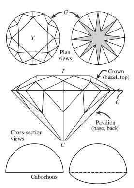
**FIGURE 36.4** Different regions of polished (cut, faceted) stones and two cross sections of cabochons. T, table; C, culet; G, girdle.
