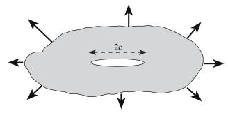
FIGURE 18.5 The "Griffith" crack of length 2c.
