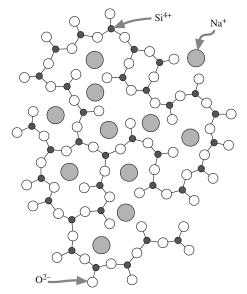
**FIGURE 7.20** Schematic of how network modifiers in glass cause nonbridging O ions.
