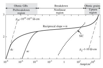
**FIGURE 30.17** Typical *I–V* characteristic for a ZnO varistor.
