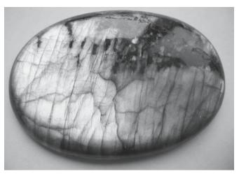
FIGURE 36.17 Laboradite causes an iridescence due to scattering by twin planes in the feldspar crystal.
