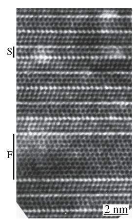
**FIGURE 14.26** The structure of β-alumina as a repetition of chemical twin boundaries. S and F are a block of spinel and an SF, respectively.
