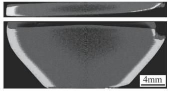
FIGURE 10.4 High-resolution X-ray CT images from the top and side of the same sample.
