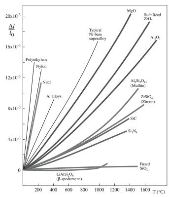
FIGURE 34.15 Thermal expansion characteristics of several polycrystalline ceramics.
