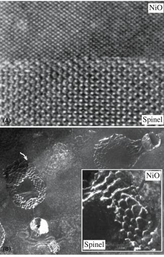
FIGURE 15.3 The spinel/NiO PB. (a) HRTEM image of latticematched PB; (b) dislocations are present at the interface after relaxation to accommodate lattice misfit. The inset is from the arrowed region.
