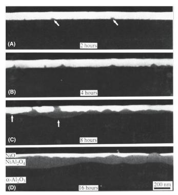
**FIGURE 25.18** SEM images of reactions at GBs in thin films of NiO deposited on (0001)  $Al_2O_3$ .
