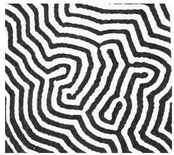
FIGURE 33.19 Domain pattern in a YIG thin film revealed by the Faraday effect. The stripes are 12 µm wide.
