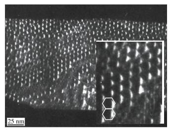
**FIGURE 15.1** Image of an Fe<sub>2</sub>O<sub>3</sub> film on an Al<sub>2</sub>O<sub>3</sub> substrate showing both  $\Sigma=1$  and  $\Sigma=3$  PBs. The inset shows the hexagonal dislocation network.
