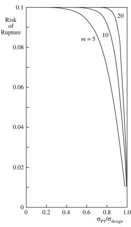
**FIGURE 16.26** Plot showing the risk of rupture after proof testing to the ratio of proof-test stress to design stress.
