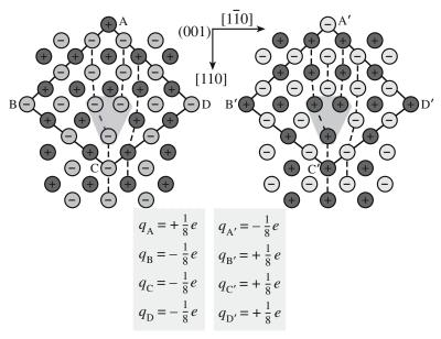
FIGURE 12.10 The core of a dislocation in NaCl.
