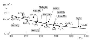
FIGURE 34.11 Plot of the average coefficient of thermal expansion versus melting temperature for many ceramics.
