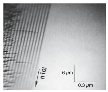
**FIGURE 13.22** REM image from a GaAs substrate with a Al<sub>x</sub>Ga<sub>1-x</sub>As/GaAs superlattice; the substrate has cleaved perfectly.
