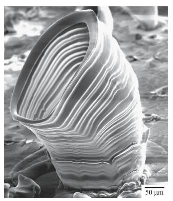
FIGURE 17.22 Microblown silica shape formed on oxidized SiC.
