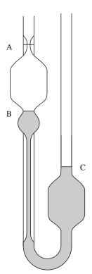
FIGURE 22.8 An Ostwald viscometer. The liquid is initially at B and C, then is drawn up to A.
