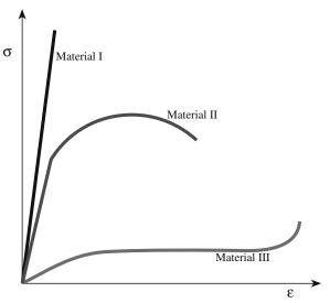
FIGURE 16.2 Idealized stress-strain curves for different materials classes.
