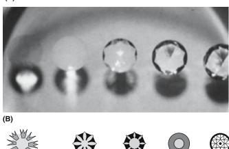
FIGURE 36.11 Determining the shadow patterns when stones are immersed in methyl iodide or liquid of other n. Different liquids are given in Table 36.4.
