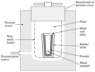
FIGURE 23.3 Schematic of a wet-bag isostatic pressing system.
