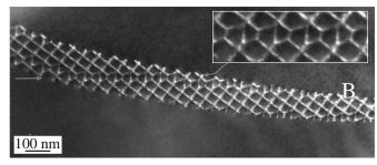
**FIGURE 14.13** An extrinsic dislocation interacting with a low-angle {001} twist GB in spinel. Note how all the dislocations are changed by the interaction as seen in the enlarged inset.
