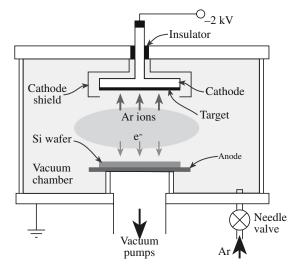
FIGURE 28.4 Schematic of a sputtering system.
