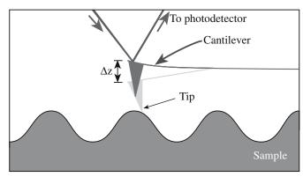
FIGURE 10.15 Schematic of the tip/sample interaction in AFM using a cantilever system.
