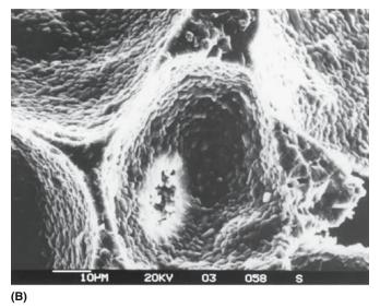
FIGURE 13.12 The surface of foam.
