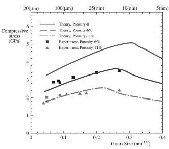
**FIGURE 17.11** Compressive yield stress as a function of grain size for nanocrystalline  $TiO_2$  at three levels of porosity.
