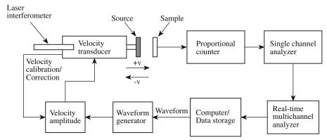
FIGURE 10.23 Schematic of the set-up for Mössbauer spectroscopy.
