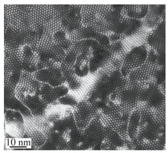
**FIGURE 14.22** Curved twin boundaries in a thin film of NiO on an Al<sub>2</sub>O<sub>3</sub> substrate. (The hexagonal pattern is a moiré interference effect.)
