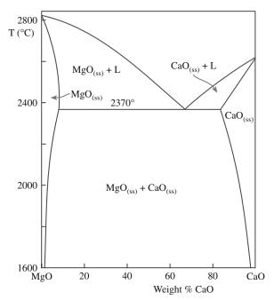
FIGURE 8.11 The MgO-CaO phase diagram.
