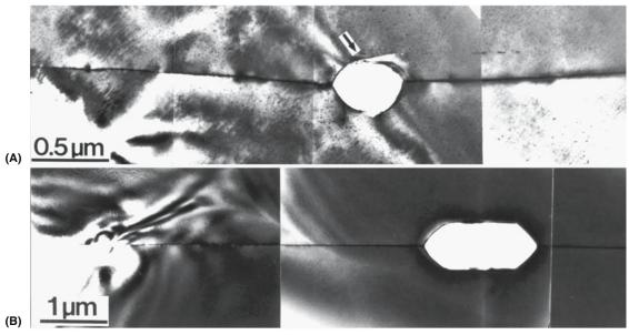
FIGURE 14.28 The same GB in Al<sub>2</sub>O<sub>3</sub> processed with and without glass.
