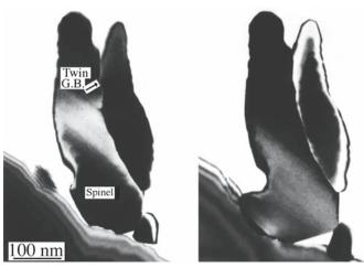
FIGURE 25.9 Particle of Ni-Al spinel growing on an Al<sub>2</sub>O<sub>3</sub> thin film.
