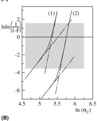
**FIGURE 16.24** (a) Different flaws lead to different values of *m*. (b) Weibull plot for a sample having both surface and volume flaws.
