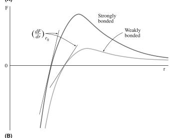
**FIGURE 4.1** (a) Bond-energy curve for KCI. At infinite separation, the energy is that required to form K<sup>+</sup> and Cl<sup>-</sup> from the corresponding atoms. (b) Force-distance curves for two materials: one where the bonding is strong and one where it is weak.
