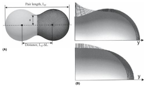
FIGURE 24.28 (a, b) Modeling sintering using Surface Evolver.
