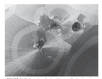
FIGURE 21.15 Illustration of spherulitic crystallization in a glass.
