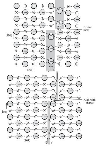
FIGURE 12.17 Schematic of kinks on a screw dislocation showing they may or may not be charged.
