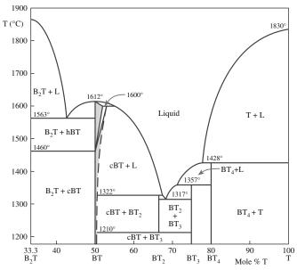
FIGURE 8.23 The BaTiO<sub>3</sub> phase diagram.
