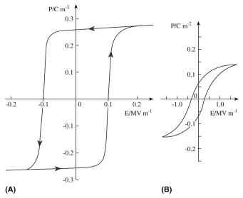
FIGURE 31.10 Hysteresis loops for BaTiO<sub>3</sub>. (a) Single-domain single crystal. (b) Polycrystalline ceramic.
