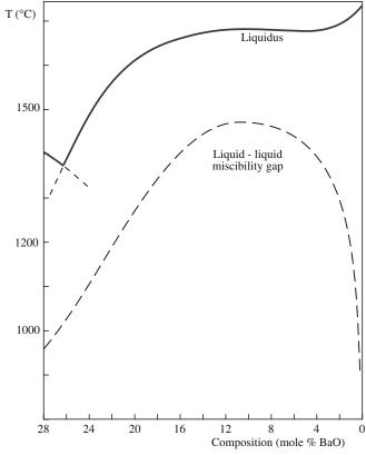
FIGURE 8.25 The silica-rich end of the BaO-SiO<sub>2</sub> phase diagram.
