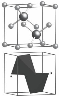
**FIGURE 6.10** The Cu<sub>2</sub>O crystal structure. (Top) Ion positions; (bottom) two "occupied" tetrahedra. The Cu ions sit at the fcc sites; two O ions "occupy" tetrahedral sites.
