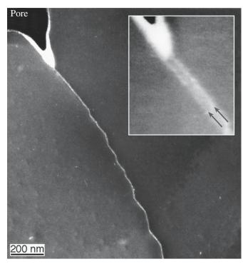
**FIGURE 14.35** A cautionary tale: the "glass" in the faceted GB is actually material deposited in surface grooves during sample preparation.
