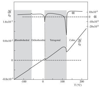
FIGURE 34.13 The coefficient of thermal expansion of BaTiO<sub>3</sub> as a function of temperature.
