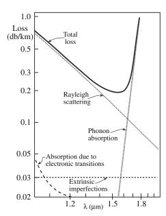
FIGURE 32.18 Loss spectrum for fibers.
