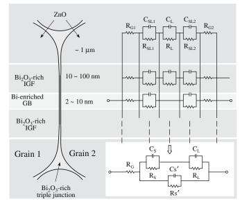
FIGURE 14.38 Modeling IGFs in ZnO varistor materials.
