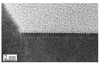
FIGURE 13.21 Cross section HRTEM image of a surface of Fe<sub>2</sub>O<sub>3</sub>.
