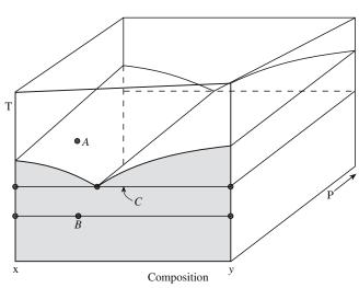
**FIGURE 8.9** A model binary phase diagram showing T, P, and composition as variables.
