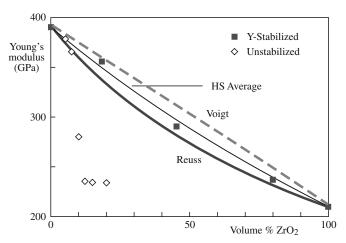
**FIGURE 16.7** Comparison of predicted values of Young's modulus for an  $Al_2O_3$  tetragonally stabilized  $ZrO_2$  composite with experimental data.
