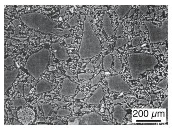
**FIGURE 2.7** Microstructure of a "Masters of Tabriz" tile showing many large grains of crystalline SiO<sub>2</sub>.
