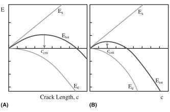
**FIGURE 18.4** Plots of energy versus crack length.  $E_{\rm tot}$  is the sum of  $E_{\rm s}$  and  $E_{\rm e}$ . The right plot corresponds to a greater applied stress (on this scale the stress is greater by  $\sqrt{2}$  and  $c_{\rm crit}$  is correspondingly reduced by a factor of 2).
