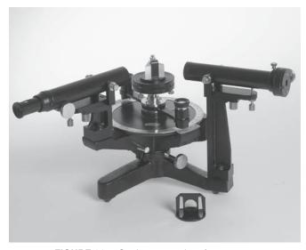
FIGURE 36.7 Goniometer-style refractometer.
