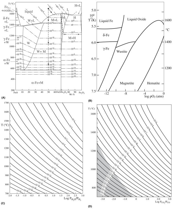
FIGURE 8.20 (a, b) The FeO-Fe<sub>2</sub>O<sub>3</sub> phase diagram; (c) the H-O system; (d) the C-O system.
