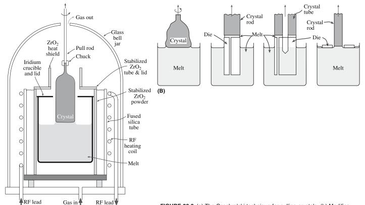
$\label{eq:Figure 29.3} \textbf{(a) The Czochralski technique for pulling crystals. (b) Modifications to Czochralski. Compared with the conventional geometry (left).}$
