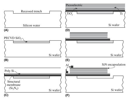
FIGURE 31.23 Steps in the production of a MEMS cantilever. (a) Create trench by etching; (b) deposit SiO<sub>2</sub> layer by pressure-enhanced chemical vapor deposition (PECVD); (c) deposit Si<sub>3</sub>N<sub>4</sub> followed by polysilicon; (d) deposit the piezoelectric film on an electrode/diffusion barrier system; (e) pattern and etch; (f) apply metal contacts and sacrificial etch.
