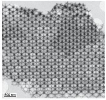
FIGURE 15.14 An ordered mesoporous material.
