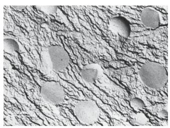
**FIGURE 21.12** SEM image of crystallized glass. The glass is a binary Li–Be fluoride opal glass 40 mol% LiF, 60 mol% BeF $_2$  containing small amounts of Ag and Ce (0.001 and 0.01 mol%, respectively). The glassy droplets (BeF $_2$  rich) are surrounded by a crystallized matrix.
