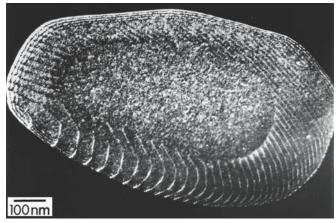
FIGURE 25.7 Growing particle of spinel in a matrix of Fe-doped Al<sub>2</sub>O<sub>3</sub> during internal reduction.
