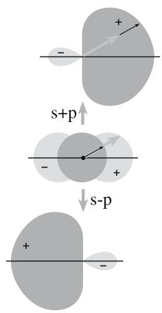
**FIGURE 4.15** Two sp hybrid orbitals formed by adding and subtracting the corresponding wave functions.
