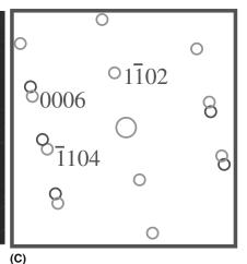
FIGURE 14.20 Rhombohedral twin boundary in Al<sub>2</sub>O<sub>3</sub> and its diffraction pattern.
