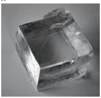
FIGURE 5.2 Crystals with faceted surfaces illustrating macroscopic symmetry elements; (a) MgO, (b) calcite.
