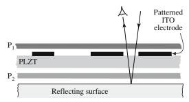
FIGURE 32.24 Basic layout of a PLZT reflective display.
