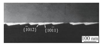
**FIGURE 14.30** An IGF in  $Al_2O_3$  that was initially uniformly thick varying in thickness after heat treatment.
