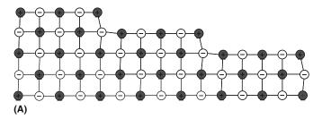
**FIGURE 13.23** Different representations of surface steps: (a) (100) cross section of MgO; b) wurtzite; (c) (110)  $TiO_2$ .
