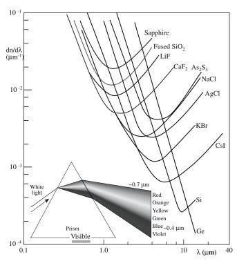
FIGURE 32.6 Dispersion as a function of wavelength for a number of ceramics. The inset is the classic illustration of dispersion, a prism separating white light into its spectral components.
