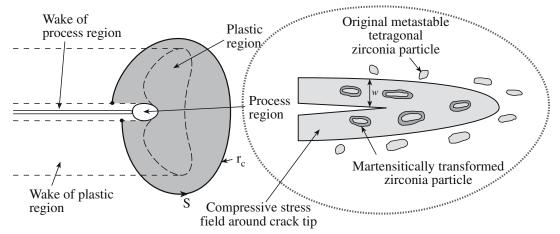
FIGURE 18.22 Illustration of transformation toughening in a ceramic matrix containing ZrO<sub>2</sub> particles.
