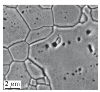
FIGURE 24.24 Pores trapped in grains.
