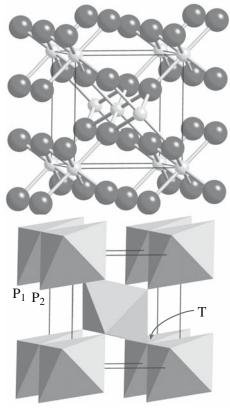
**FIGURE 6.11** Rutile crystal structure viewed nearly parallel to the *z*-axis. Each of the pairs of overlapping octahedra (e.g.,  $P_1/P_2$ ) shares an edge. The two octahedra in the lower right thus have point T in common. The central octahedron touches each of the eight at the corners.
