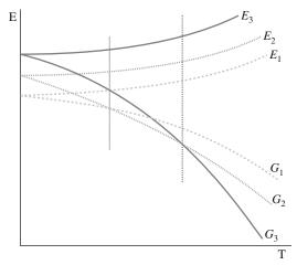
**FIGURE 5.10** Schematic showing the relationship between internal energy E and free energy G of three polymorphic forms:  $E_3 > E_2 > E_1$  and  $S_3 > S_2 > S_1$ . The form with the lowest G will be the one usually found at a specific temperature.
