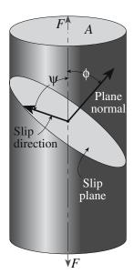
FIGURE 17.6 Geometry used to determine the critical resolved shear stress.
