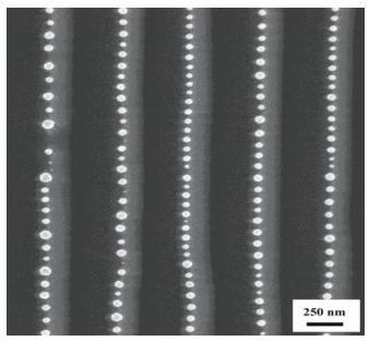
**FIGURE 13.28** Self-assembly of Pt nanoparticles due to charging along a surface ridge in  $Al_2O_3$ : the particles sit on the ridge not the valley!
