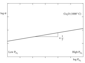
FIGURE 30.16 Conductivity of Cu<sub>2</sub>O as a function of pO<sub>2</sub>.
