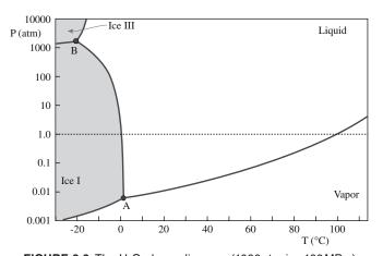
FIGURE 8.6 The  $H_2O$  phase diagram. (1000 atm is ~100 MPa.)
