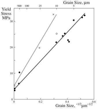
**FIGURE 17.10** Grain size dependence of yield strength for KCI. The solid circles are for pure material with a <100> texture; the open circles are for pure material with a <111> texture. The crosses are for Sr-doped KCI.
