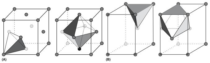
FIGURE 5.9 (a) Interstitial sites in the fcc structure; (b) interstitial sites in the hcp structure.
