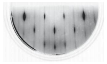
**FIGURE 13.19** RHEED pattern from anatase film grown on  $LaAlO_3$ .
