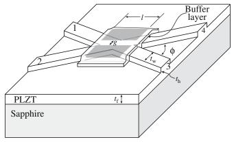
FIGURE 32.26 An example of a PLZT thin film optical switch on sapphire.
