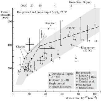
**FIGURE 16.5** Compilation of strength data as a function of grain size for polycrystalline  $Al_2O_3$ .
