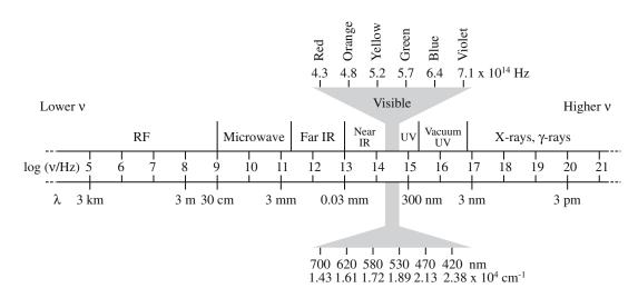
FIGURE 32.1 The electromagnetic spectrum. The visible region has been expanded for clarity. It is actually a very small part of the spectrum.
