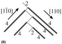
**FIGURE 13.4** A faceted shallow thermal etch pit on the (001) surface of spinel. 2 and 4 refer to the height of the steps (0.2 nm and 0.4 nm).
