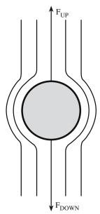
**FIGURE 20.10** Illustration of the force balance during settling of a particle in a Newtonian fluid with laminar flow.
