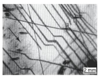
FIGURE 10.3 X-ray topography image showing dislocations in KDP imaged using a 022 reflection.
