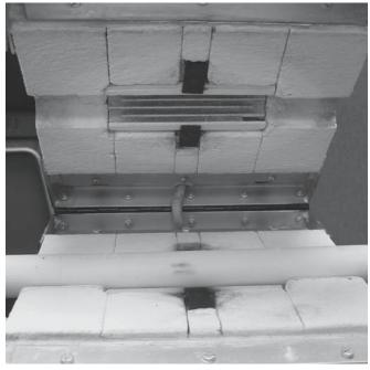
FIGURE 9.3 An electrically heated tube furnace.
