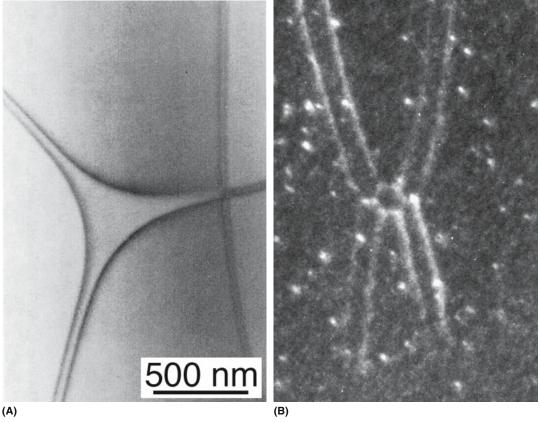
FIGURE 12.23 Dislocation nodes in (a) AIN; (b) spinel.
