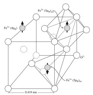
**FIGURE 33.12** Subcell of magnetite showing the location of Fe ions and their spin moments.
