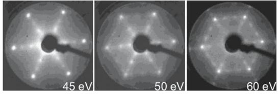
FIGURE 13.18 LEED patterns from GaN on  $Al_2O_3$  as the accelerating voltage is changed.
