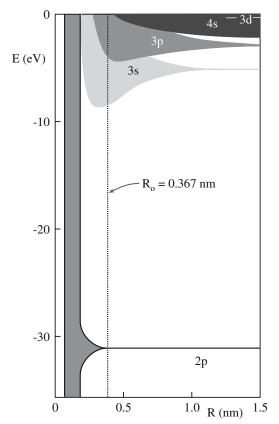
**FIGURE 4.21** Formation of electron "bands" as the interatomic spacing is reduced.
