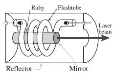
FIGURE 32.19 Schematic of the components of a ruby laser.
