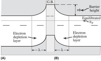
**FIGURE 30.18** Proposed band diagram for two semiconducting ZnO grains separated by an IGF: (a) showing the location of acceptor sites in the IGF; (b) at equilibrium. Application of a potential decreases the barrier height.
