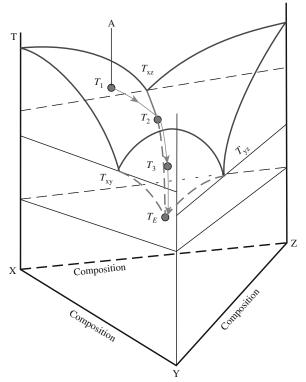
FIGURE 8.19 Illustration of a cooling path in a ternary system.
