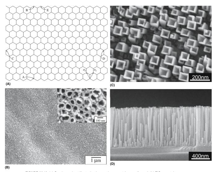
FIGURE 29.19 (a) Graphene sheet illustrating how carbon nanotubes are formed. (b) TiO<sub>2</sub> nanotubes. (c) and (d) IrO2 nanotubes.
