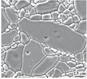
FIGURE 24.21 Elongated exaggerated grain in Al<sub>2</sub>O<sub>3</sub>.
