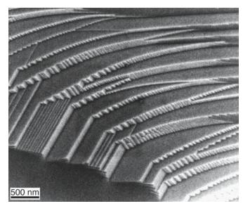
FIGURE 10.6 SE image showing steps on an alumina surface.
