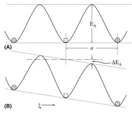
FIGURE 30.20 Potential energy barrier to ion movement. (a) In the absence of an applied field and (b) with an applied field.  $E_A$  is the activation energy and a the jump distance between ion sites.
