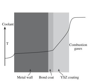
FIGURE 27.10 Schematic representation of a thermal barrier coating. The relative temperatures in the different parts of the coating are indicated.
