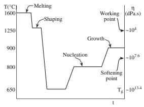
FIGURE 26.14 Processing cycle for a glass-ceramic.
