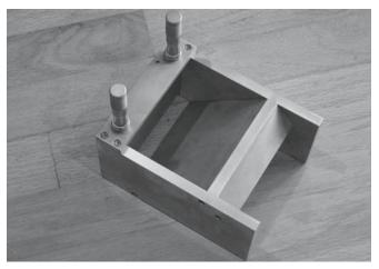
FIGURE 27.3 Typical doctor blade assembly.
