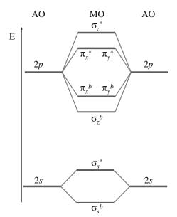
**FIGURE 4.13** Energy level diagram for homonuclear diatomic molecule where there is negligible s-p hybridization.
