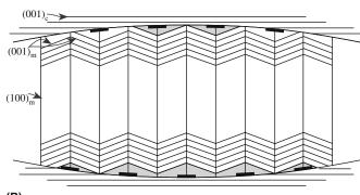
FIGURE 25.5 Twins in transformed particles: (a) experimental observation and (b) a possible mechanism.
