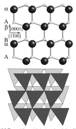
FIGURE 6.6 The wurtzite crystal structure viewed along [1120]. (Top) Ion positions showing the  $A\alpha B\beta$  stacking; (bottom) two interpenetrating arrays of corner-sharing tetrahedra. (Only one set is needed to construct the crystal.)
