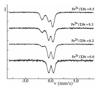
**FIGURE 10.25** Mössbauer spectra from glasses containing different concentrations of  $Fe^{2+}$ .
