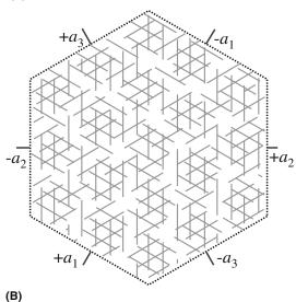
FIGURE 36.15 Asterism: the effect of precipitates oriented along several different directions giving rise to the star in star sapphire.
