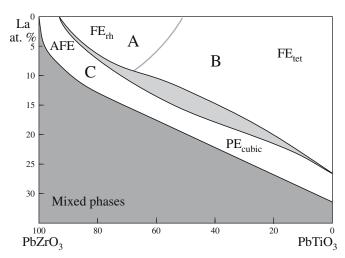
FIGURE 32.21 The PLZT phase diagram. A, memory; B, linear; C, quadratic.
