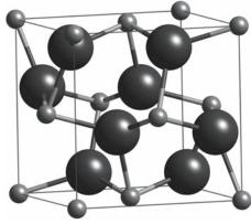
**FIGURE 6.8** The  $FeS_2$  crystal structure. The Fe ions occupy the fcc positions; the cubic cell also contains four S-S dumbells.
