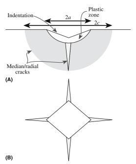
**FIGURE 16.17** Cracks at an indent allow determination of  $K_{lc}$ .
