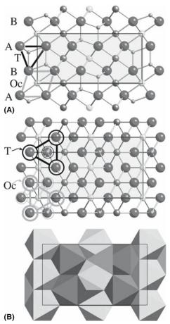
FIGURE 7.6 The crystal structure of olivine, an orthosilicate. (a) View along [001]; (b) view along [100]. Examples of octahedra and tetrahedra are outlined in both figures. Typified by forsterite, Mg<sub>2</sub>SiO<sub>4</sub>.
