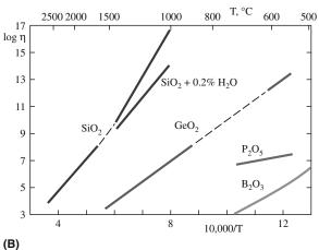
**FIGURE 21.4** (a) Viscosity as a function of temperature (T) for several silicate glasses: units of  $\eta$  are dPa·s. (b) Viscosity as a function of temperature (1/T) for the main glass-forming oxides. Notice the effect that a small amount of water has on the viscosity of silica glass.
