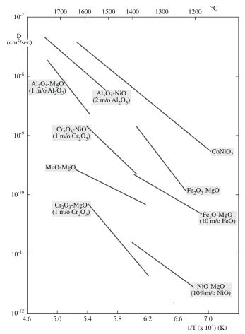
FIGURE 25.16 Dependence of diffusion coefficients on T for different oxides
