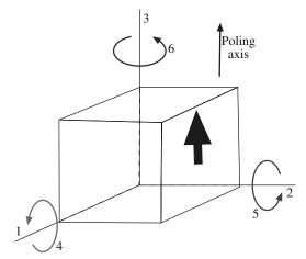
FIGURE 31.19 Notation of axes for a piezoelectric ceramic.
