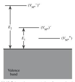
FIGURE 30.15 Schematic representation of energy levels in a deficit semiconductor such as Cu2-xO.
