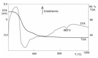
**FIGURE 10.37** DTA and TGA measurements showing the reaction as CA<sub>2</sub> crystallizes.
