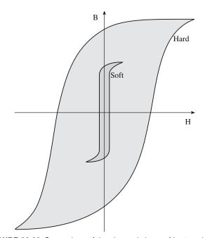
FIGURE 33.23 Comparison of the size and shape of hysteresis loops for hard and soft magnets.
