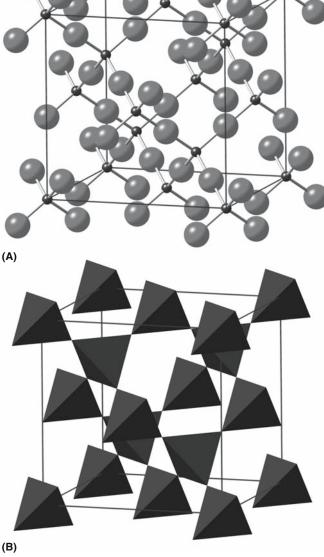
FIGURE 7.5 The crystal structure of cristobalite. The most symmetric of SiO<sub>2</sub> having cubic symmetry (m3m) and a lattice parameter of 0.72 nm.
