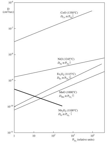
FIGURE 11.14 Diffusion coefficients varying with pO<sub>2</sub>.
