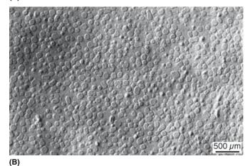
**FIGURE 21.13** SEM images of (a) Na–Be and (b) K–Be fluoride glass 15 mol% KF (or NaF), 85 mol% BeF<sub>2</sub>. This glass is cloudy: if the droplets were smaller the glass would be clear. Replacing K by Rb actually reduced the droplet size to 10–20 nm.
