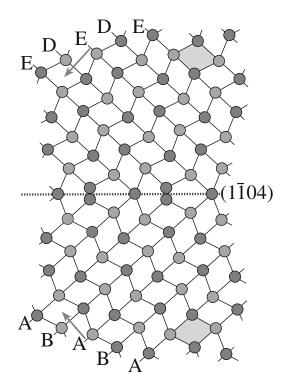
**FIGURE 14.19** Schematic of a  $(1\bar{1}04)$  twin boundary in  $Al_2O_3$ . The arrows show the <0001> directions; the letters show the hcp stacking of the anions. The cations are omitted but sit in the octahedral—shown by the shaded rhombi.
