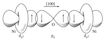
FIGURE 33.9 Overlap between Ni dze orbitals and O pz orbitals in Ni.
