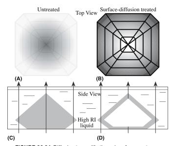
FIGURE 36.34 Diffusion to modify the color of a gemstone.
