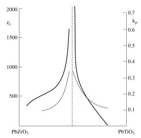
**FIGURE 31.21** Dielectric constants and coupling coefficients for PZT compositions near the MPB.
