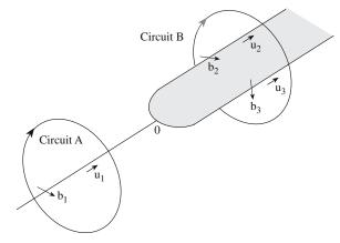
FIGURE 12.3 Diagram used for proving Frank's rule for conservation of b.
