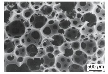
FIGURE 15.15 Sintered alumina foam made using a soap-nut slurry with a 40 volume % ceramic.
