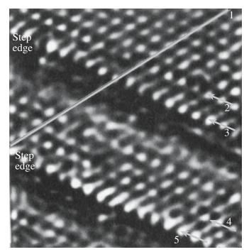
FIGURE 13.15 STM of a surface of Fe<sub>2</sub>O<sub>3</sub>. 1-5 indicate different rows of atoms.
