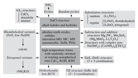
**FIGURE 6.9** Schematic showing how two simple structures (NaCl and FeS<sub>2</sub>) can be related to more complicated crystal structures.
