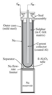
FIGURE 30.21 Schematic of a "central sulfur" cell. Typically, the electrolyte tube is some 300 mm long and 30 mm in diameter.
