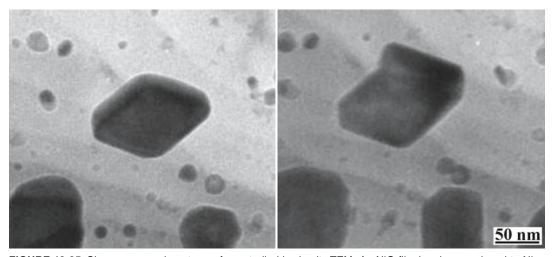
FIGURE 13.25 Changes occurring at a surface studied by in situ TEM. An NiO film has been reduced to Ni, which then dewets the sample and grows on the sapphire substrate.
