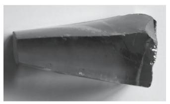
FIGURE 36.28 As grown crystal of RE-doped CZ.
