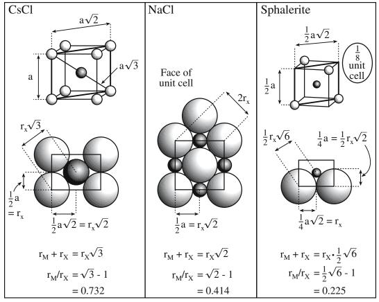
FIGURE 5.7 Geometric method for calculating limiting radius ratios.
