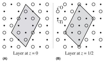
FIGURE 30.5 The structure of TiO. (a) The (100) plane. (b) The (200) plane. Both show the absence of alternate ions along <110> directions. The resultant superlattice has a monoclinic unit cell as indicated by the shaded region.
