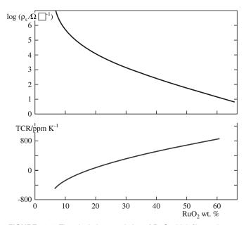
FIGURE 30.9 Electrical characteristics of RuO<sub>2</sub> thick-film resistors.
