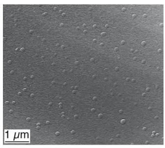
FIGURE 8.24 Image of small droplets of glass in a glass matrix. The composition of the glass is 16wt% CaO, 10wt% MgO, 14wt%  $Al_2O_3$ , and 60 wt%  $SiO_2$ .
