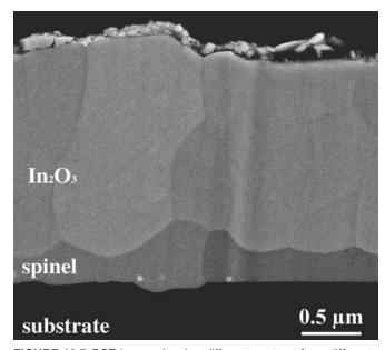
**FIGURE 10.7** BSE image showing different contrast from different materials in an  $MgO/In_2O_3$  reaction couple.
