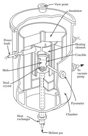
FIGURE 29.9 Illustration of the heat-exchange (Schmid-Viechnicki) method.
