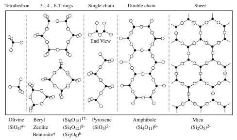
FIGURE 7.4 Arranging SiO<sub>4</sub> tetrahedra in different silicates. The exception is the sheet that extends indefinitely in all directions in the plane. These are the best known ways of combining (or not) the  $SiO_4$  tetrahedra.
