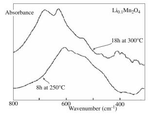
FIGURE 10.18 FTIR absorption spectra from Li<sub>x</sub>Mn<sub>2</sub>O<sub>4</sub> insertion electrodes after different heat treatments.
