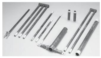
FIGURE 9.7 Examples of SiC furnace elements.
