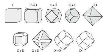
FIGURE 36.20 Different diamond shapes produced by diamonds faceting on three different crystallographic planes while keeping the same symmetry.
