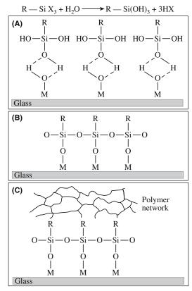
**FIGURE 20.17** Illustration of the processes involved in joining a polymer and glass using silane coupling agents. (a) Hydrolysis of the silane to the corresponding silanol; (b) hydrogen bonding between hydroxyls on the silanol and those attached to the glass; (c) polysiloxane bonded to the glass following condensation during drying; and (d) bonding between the functional group R and the polymer.
