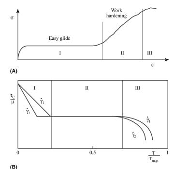
**FIGURE 17.7** (a) Stress–strain curve for a crystal suitably oriented for plastic flow. (b) Temperature dependence of the normalized critical resolved shear stress for two strain rates, where  $\gamma_1 > \gamma_2$ .
