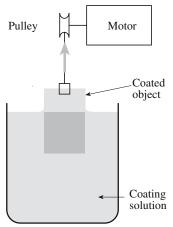
FIGURE 27.6 Schematic of a simple dip coating process.
