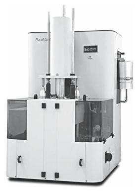
FIGURE 15.13 A commercial porosimeter.
