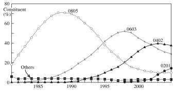
FIGURE 37.3 Multilayer ceramic capacitor-sized trends.
