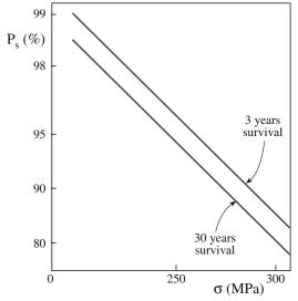
**FIGURE 16.27** SPT diagram for medical grade Al<sub>2</sub>O<sub>3</sub>. The survival probability decreases with increasing stress and longer times.
