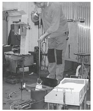
**FIGURE 26.10** Demonstration of blowing glass into a mold. Note the worker's bench, the annealing burners, and the box of frit.
