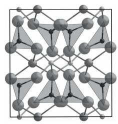
FIGURE 7.11 The crystal structure of a pyroxene (spodumene) shows layers of Li<sup>+</sup> (larger) and Al<sup>3+</sup> (smaller) ions in octahedra alternating with layers of Si<sup>4+</sup> in tetrahedra giving a nominal formula of LiAlSi<sub>2</sub>O<sub>6</sub>.
