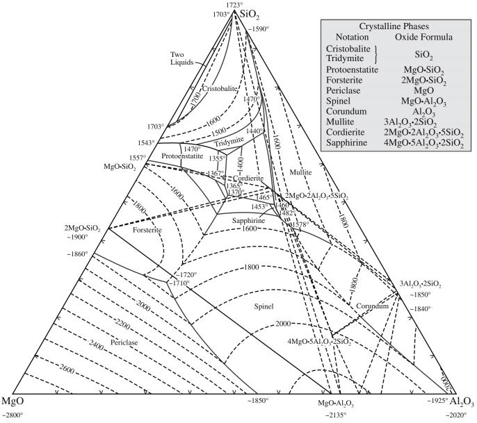
FIGURE 8.16 The MgO-Al<sub>2</sub>O<sub>3</sub>-SiO<sub>2</sub> phase diagram.
