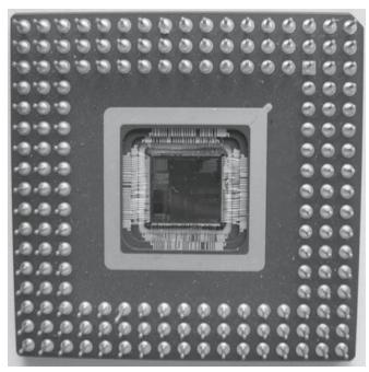
FIGURE 34.9 A ceramic pin-grid-array package (96% pure Al<sub>2</sub>O<sub>3</sub>) with multilayer Au metallization.
