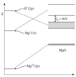
FIGURE 30.23 Energy band diagram for MgO.
