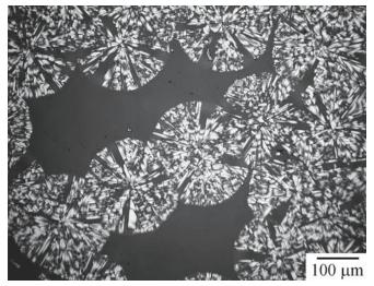
**FIGURE 21.10** Spherulitic crystallization of an amorphous  $SiO_2$  film on SiC. The spherulites are crystobalite.
