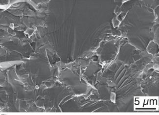
FIGURE 18.13 (a) The fracture surface of polycrystalline AIN. (b) The fracture surface of polycrystalline SiC.
