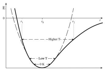
FIGURE 34.10 A typical bond-energy curve.
