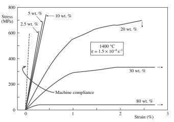
FIGURE 16.9 Stress-strain curve for Si<sub>3</sub>N<sub>4</sub> at 1400°C for various amounts of silica. The machine compliance is the inherent displacement within the instrument.
