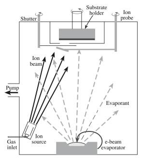
FIGURE 28.7 Ion-beam-assisted deposition system.
