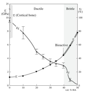
**FIGURE 35.7** Effect of volume fraction of HA on  $\mathcal{E}$  and strain to failure of HA-reinforced PE composites, in comparison to cortical
