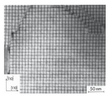
FIGURE 14.7 Two sets of orthogonal screw dislocations in a lowangle (001) twist GB in Si.
