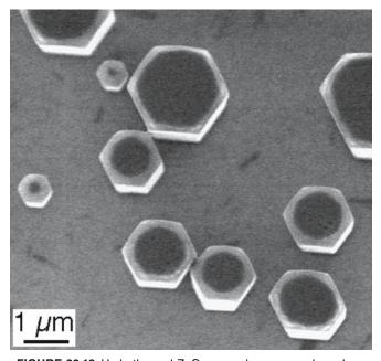
FIGURE 29.13 Hydrothermal ZnO nanorods seen nearly end on.
