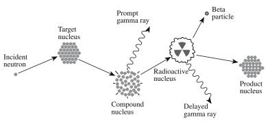
FIGURE 10.36 Schematic of the NAA process.
