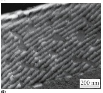
**FIGURE 14.31** Dewetting of IGFs in Si GBs: (a)  $\Sigma = 1$  {111}; (b)  $\Sigma = 5$  {001}.
