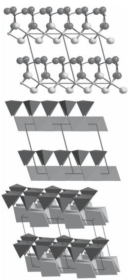
**FIGURE 7.10** In the crystal structure of kaolinite, the  $SiO_4$  tetrahedra form one side of the sheet while the octahedra contain  $OH^-$  on the outer layer attached to the  $Al^{3+}$  ions. The sheets are held together only by van der Waals bonds.
