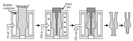
FIGURE 23.5 Making spark plugs. Hydrostatic pressure is applied by pumping oil around the rubber container, which is part of the press and thus easily removed.
