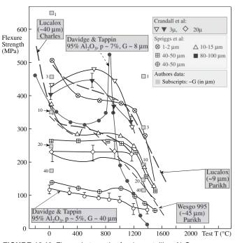
FIGURE 16.12 Flexural strength of polycrystalline Al<sub>2</sub>O<sub>3</sub> as a function of test temperature.
