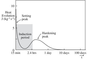
**FIGURE 2.10** Heat evolution during the setting and hardening of Portland cement.
