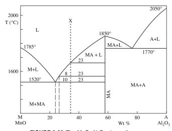
FIGURE 8.22 The MnO-Al<sub>2</sub>O<sub>3</sub> phase diagram.
