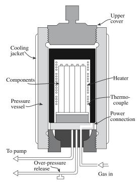
FIGURE 23.6 Schematic of a hot isostatic pressing apparatus.
