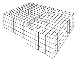
FIGURE 12.2 Schematic of a screw dislocation.
