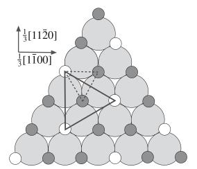
**FIGURE 12.12** Schematic used to show  ${\bf b}$  of perfect dislocations in  ${\rm Al_2O_3}.$
