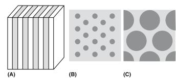
FIGURE 34.8 Three models for the distribution of two phases in a material. (a) Parallel slabs, (b) continuous matrix phase, discontinuous particulate dispersion, and (c) large isolated grains separated by a continuous minor phase.
