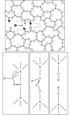
FIGURE 18.10 Environmental effects at the crack tip. A water molecule diffuses to the crack tip, chemisorbs, and rotates such that the lone pairs on the oxygen are aligned with the unoccupied electron orbitals of the Si atom.
