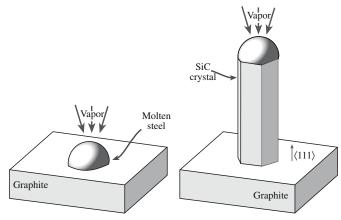
FIGURE 29.17 VLS process for growing SiC whiskers.
