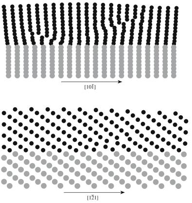
FIGURE 15.20 Schematic of stand-off dislocations accommodating lattice misfit between Nb and Al<sub>2</sub>O<sub>3</sub>.
