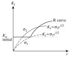
**FIGURE 18.7** A material showing R curve behavior (bold curve) exhibits a region of stable crack growth and flaw tolerant behavior. The lighter curves  $\sigma_1$  and  $\sigma_2$  represent typical Griffith behavior.
