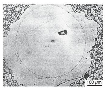
**FIGURE 24.22** Using a single-crystal sphere to model exaggerated grain growth in Al<sub>2</sub>O<sub>3</sub> doped with 1 wt% MgO; at 1800°C for 60 minutes.
