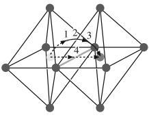
FIGURE 11.15 A probable diffusion mechanism in NaCl.
