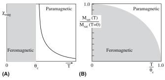
**FIGURE 33.7** Schematic showing how (a)  $\chi$  varies with T; (b) M varies with T for a ferromagnet.
