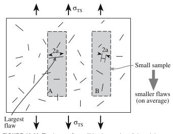
FIGURE 16.22 The largest flaw will be the weakest link and the source of failure. Smaller samples have smaller flaws.
