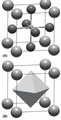
**FIGURE 7.2** The perovskite crystal structure. The lattice is simple cubic with several cations able to occupy the central octahedron. (a) Atomic model; (b) the polyhedron.
