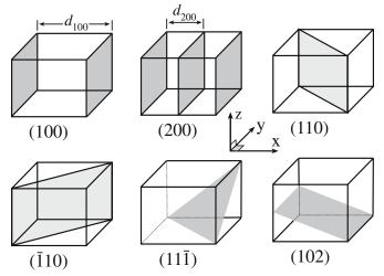
**FIGURE 5.4** Miller indices of some lattice planes. The lattice-plane spacing is given by  $d_{nkl}$ .
