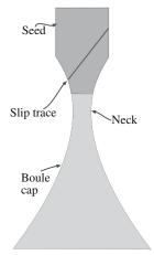
FIGURE 29.6 Schematic illustration of neck-down and flare-out geometries for growing dislocation-free crystals.
