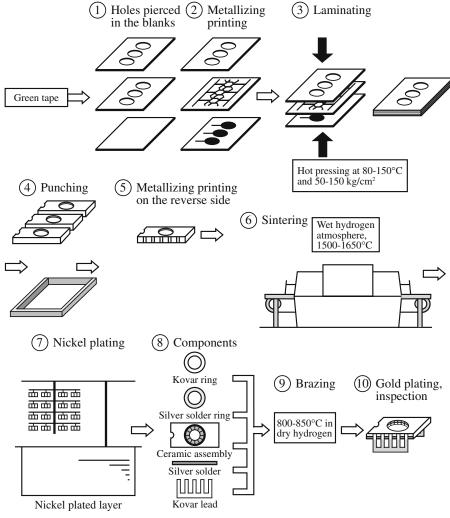
FIGURE 27.5 The steps in the production of an integrated-circuit package.
