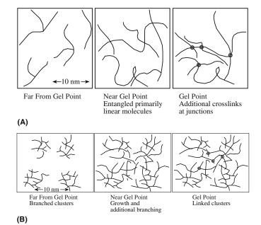
FIGURE 22.7 Illustration of (a) acid- and (b) base-catalyzed polymerization and gelation.
