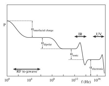
FIGURE 31.2 Frequency dependence of polarization.
