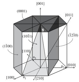
FIGURE 5.6 Indices of planes (using Miller–Bravais notation) and directions (using three-index Miller notation) in the hexagonal unit cell
