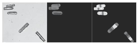
**FIGURE 35.10** Microbar codes from Corning. The cyllindrical bars are typically 100  $\mu$ m long and 20  $\mu$ m in diameter.
