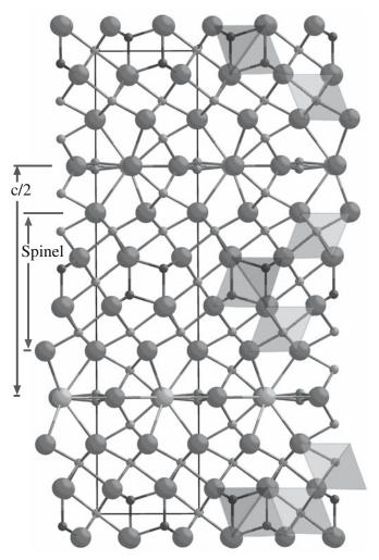
**FIGURE 7.12** The crystal structure of  $\beta$ -alumina. The main features are the large value of c, the twinned spinel blocks, and the mirror plane containing the Na<sup>+</sup> (or K<sup>+</sup> or Ca<sup>+</sup>) ion.
