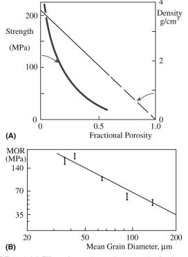
**FIGURE 16.4** (a) Effect of porosity on the strength of polycrystal-line  $Al_2O_3$ . (b) Effect of grain size on the strength of BeO.
