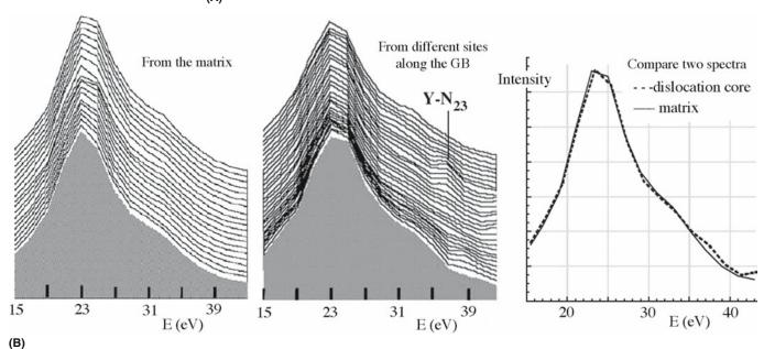
**FIGURE 14.2** Solute distribution at GBs. (a) Profiles using XEDS; (b) EELS spectra used to analyze a GB in sapphire. In (a) the integrated X-ray solute/Zn peak ratios are plotted against *d*, the distance from the GB.
