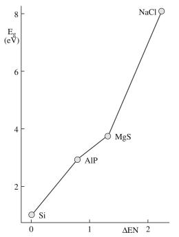
**FIGURE 30.25** Correlation of  $E_{\alpha}$  and electronegativity difference  $(\Delta EN)$ .
