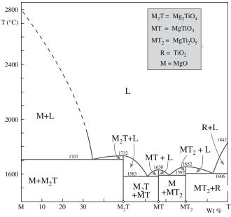
FIGURE 8.14 The MgO-TiO<sub>2</sub> phase diagram.
