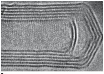
**FIGURE 7.16** The structure of (a)  $C_{60}$  and (b) carbon nanotubes. (c) Image of the end of a six-layer carbon nanotube.
