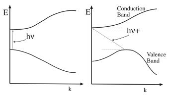
FIGURE 4.25 Illustration of direct and indirect band gap transitions. Energy is plotted versus wave vector.
