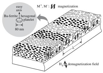
FIGURE 33.26 The principle of perpendicular recording.
