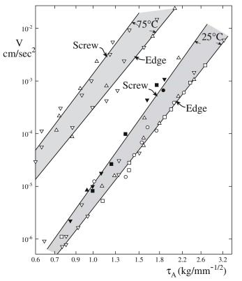
FIGURE 17.12 The stress dependence of dislocation velocity.
