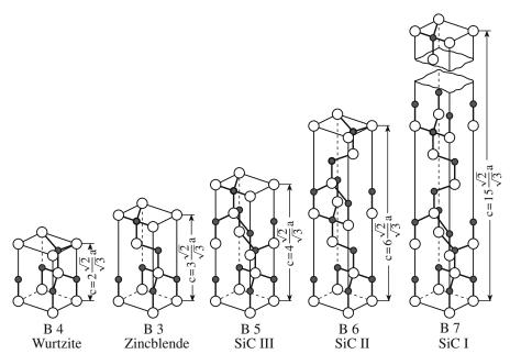
FIGURE 6.17 The stacking sequence for five SiC polytypes.
