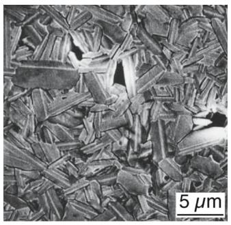
FIGURE 24.3 SiC processed with addition of Al<sub>2</sub>O<sub>3</sub> at 2050°C; etched polished surface.
