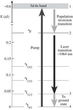
FIGURE 32.20 The four-level system for lasers.
