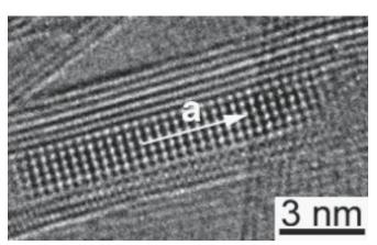
FIGURE 10.12 HRTEM image of a C nanotube partly loaded with a crystal of KCI.
