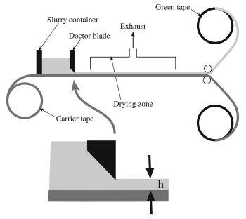
FIGURE 27.1 Schematic diagram of the tape casting process.
