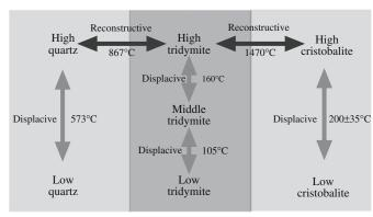
**FIGURE 6.16** Schematic of how the polymeric forms of silica can be converted into one another by displacive or reconstructive structural transformations.
