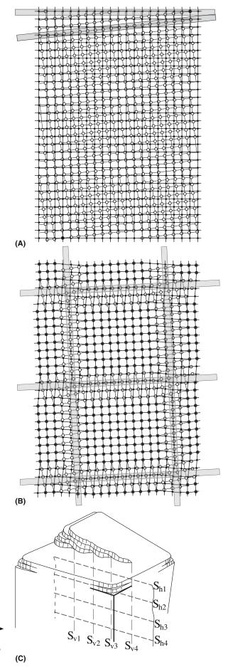
**FIGURE 14.5** Schematics of a low-angle twist GB. (a) Before and (b) after local atomic relaxations. (c) The twist when the GB emerges at the surface.
