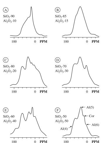
FIGURE 10.22 NMR signals from an Al-Si glass.
