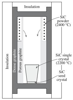
**FIGURE 29.18** Modified sublimation process for SiC single crystals.
