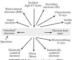
FIGURE 10.9 Signals produced in a TEM.
