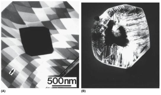
FIGURE 10.10 (a) BF and (b) DF image (using a spinel reflection) of a particle of NiO on a film of Al<sub>2</sub>O<sub>3</sub> before and after reaction.
