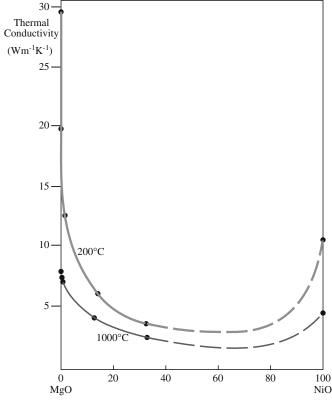
FIGURE 34.6 The thermal conductivities of solid solutions in the MgO-NiO system.
