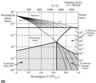
**FIGURE 17.19** (a) Schematic of creep deformation map for a polycrystalline ceramic. (b) Creep deformation map for  $Al_2O_3$ .
