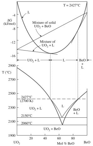
$\textbf{FIGURE 8.3} \ \ \text{The UO}_2\text{--BeO} \ phase diagram determined using free energy calculations.}$
