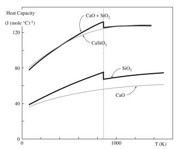
FIGURE 34.2 Heat capacity of SiO<sub>2</sub> as a function of temperature.
