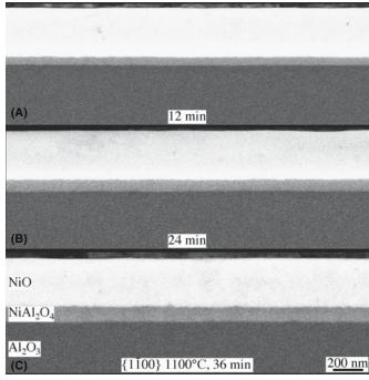
FIGURE 25.19 SEM images of growth of spinel between thin films of NiO and (0001) Al<sub>2</sub>O<sub>3</sub> when an initial buffer layer of spinel is present.
