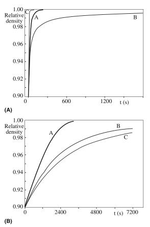
**FIGURE 24.10** Calculated densification curves at final stage of sintering at 1727°C for alumina powder compacts for grain size of (a)  $0.8\,\mu m$  and (b)  $4.0\,\mu m$  at 90% density. The curves are calculated using different equations but show the same trends.
