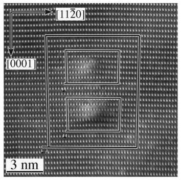
FIGURE 12.7 HRTEM of the core of a dislocation in Al<sub>2</sub>O<sub>3</sub>.
