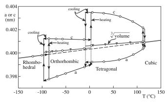
FIGURE 31.9 Experimental measurements of lattice parameters of BaTiO<sub>3</sub> as a function of T. Note the change in volume at each transition and the hysteresis in the lattice parameters.
