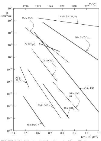
FIGURE 11.12 Arrhenius plots for different oxides: diffusion coefficients varying with  $T^{-1}$ .
