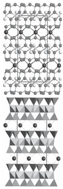
FIGURE 7.9 The crystal structure of mica showing the large K<sup>+</sup> ions forming a sheet of octahedral sites. The c lattice parameter normal to this sheet is 2.0 nm with a and b being much smaller, 0.52 and 0.90, respectively. The polyhedron model emphasizes the layer nature of the structure.
