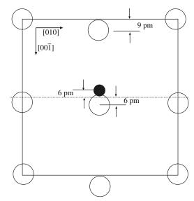
FIGURE 31.7 [100] projection of BaTiO<sub>3</sub> showing ion displacements below  $\theta_c$  (not to scale).
