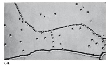
FIGURE 14.9 Seeing low-angle GBs by (a) decoration (silver particles on a GB in KCI) and (b) etch pits (LiF).
