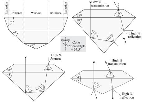
FIGURE 36.10 The origin of the sparkle in gemstones: total internal reflection (TIR).
