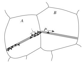
FIGURE 17.9 Illustration of slip propagation from grain A to grain B.
