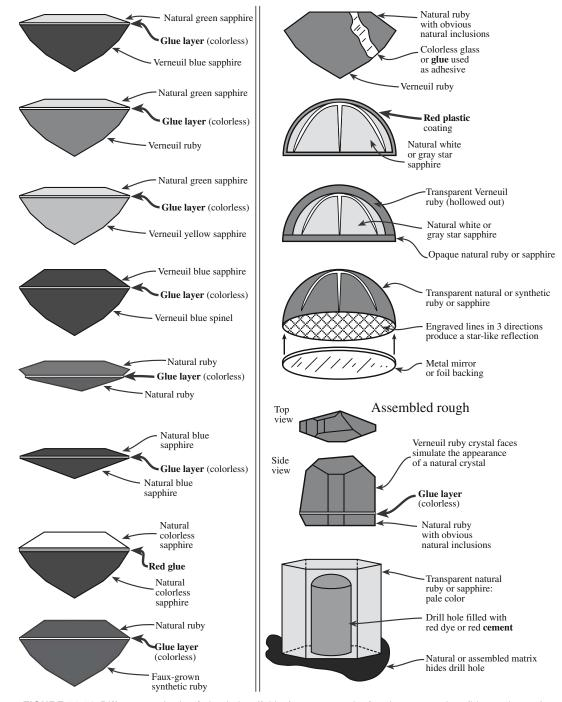
FIGURE 36.31 Different methods of simulating (faking) gemstones by forming composites (bicrystals, etc.).
