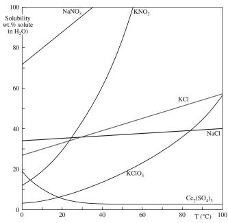
FIGURE 20.5 Solubility (grams of solute in 100 g H<sub>2</sub>O) versus temperature for several ionic compounds.
