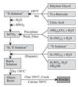
FIGURE 20.7 Flow chart for preparing SrTiO<sub>3</sub> powders by the Pechini method.
