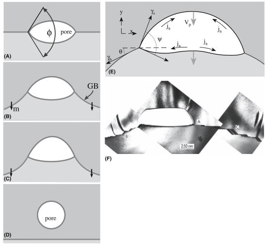
FIGURE 24.14 (a-e) GB/pore interaction: the break-away process.
