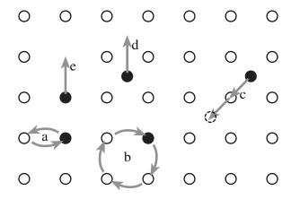
FIGURE 11.10 Possible mechanisms occurring during diffusion. (a) Exchange, (b) ring, (c) vacancy, (d) interstitial, (e) knock-on.
