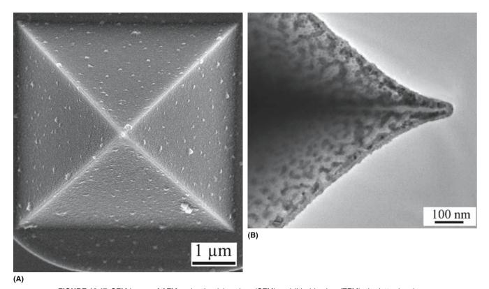
FIGURE 13.17 SEM image of AFM probe tips (a) end-on (SEM) and (b) side view (TEM); the latter has been coated to test the interaction with the sample.
