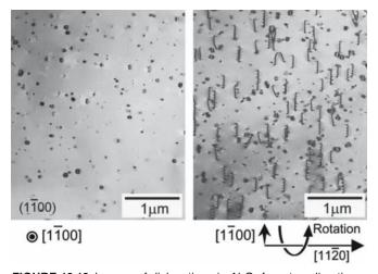
FIGURE 12.13 Images of dislocations in Al<sub>2</sub>O<sub>3</sub> from two directions.
