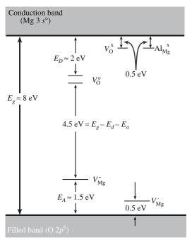
FIGURE 30.26 Defect levels in MgO.
