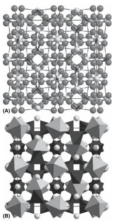
**FIGURE 7.7** The crystal structure of garnet. The general formula is  $A_3B_3(CO_4)_3$  where C is Si for the silicates. The B cation sits in an octahedral site while the largest cation A is located in a dodecahedron. The bcc unit cell has a lattice parameter of ~1.1 nm. With 20 atoms in the chemical formula there are 160 atoms in the unit cell.
