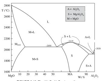
FIGURE 8.12 The MgO-Al<sub>2</sub>O<sub>3</sub> phase diagram.
