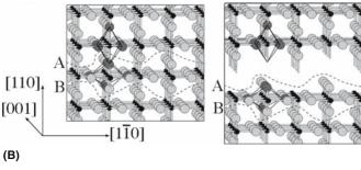
FIGURE 10.14 STM image of the (110) surface of TiO<sub>2</sub>. The features labeled 'A' have been assigned as oxygen vacancies; the features labeled 'B' have not been identified. The schematics show the TiO<sub>2</sub> structure (compare to Fig. 6.11) and a model showing the proposed surface reconstructon.
