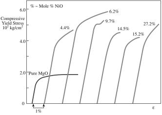
FIGURE 17.14 Illustration of solute hardening in MgO.
