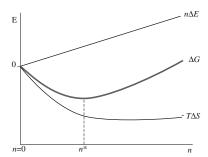
FIGURE 11.3 Schematic showing how the free energy decreases to a minimum as the number of vacancies increases.
