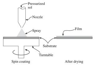
FIGURE 27.7 Schematic of the spin coating process.
