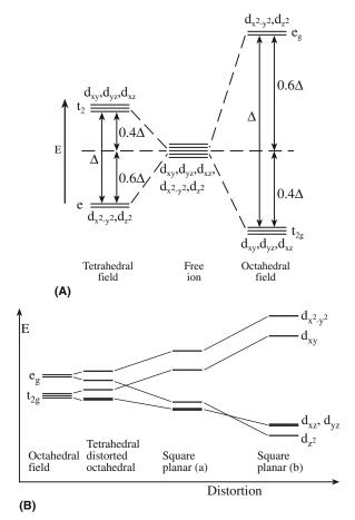
FIGURE 32.9 (a) Splitting of the d orbitals in a ligand field. (b) Splitting of d orbitals in a distorted octahedral ligand field in corundum.
