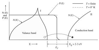
FIGURE 4.23 Plot of the density of states function and Fermi function versus energy.
