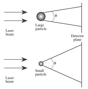
FIGURE 20.13 Scattering of light by large and small particles.
