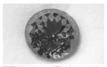
FIGURE 36.29 A single-crystal of RE-doped as-grown synthetic CZ. (Diameter =  $2.5 \, \text{cm}$ ).
