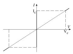
**FIGURE 30.31** *I–V* characteristics of a Josephson junction.
