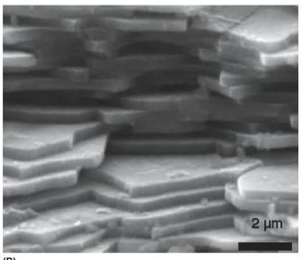
FIGURE 35.12 (a) Schematic of the abalone shell. (b) Abalone slabs
