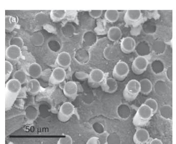
FIGURE 18.18 SEM image showing fiber pullout on the fracture surface of AIPO<sub>4</sub>-coated alumina/mullite fiber/Al<sub>2</sub>O<sub>3</sub> CMC, hot pressed at 1250°C for 1 h.
