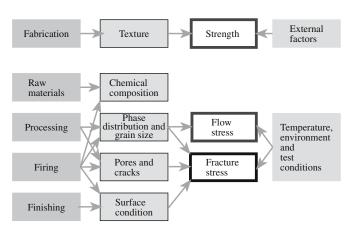
**FIGURE 16.3** Factors affecting the mechanical properties of ceramics.
