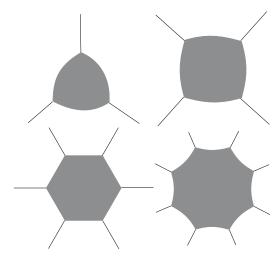
FIGURE 24.9 Angles and grains. In 2D the grains shrink if there are fewer than six sides and expand if there are more than six
