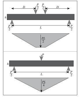
FIGURE 16.11 The geometries for three- and four-point bending.
