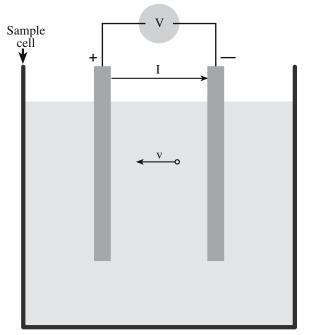
FIGURE 27.11 Schematic diagram of a particle electrophoresis cell.
