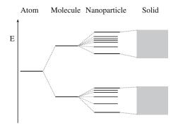
**FIGURE 4.26** Illustration of how the energy band gap arises in a nanoparticle.
