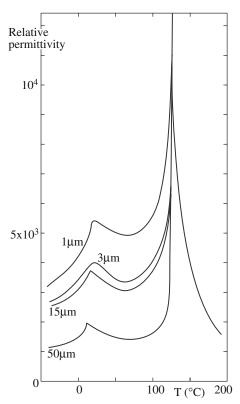
FIGURE 31.15 Effect of grain size on the dielectric constant of BaTiO<sub>3</sub>.
