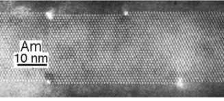
FIGURE 25.17 Chemical reactions by movement of steps on in interface. a) β-Al<sub>2</sub>O<sub>3</sub> growing in spinel; (b,c) amphibote growing in orthodyroxene.
