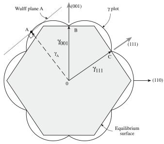
**FIGURE 13.1** Wulff plot looking along the  $[1\overline{1}0]$  direction for an fcc crystal.
