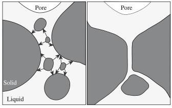
FIGURE 24.23 Schematic of Ostwald ripening.
