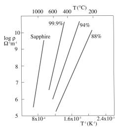
**FIGURE 1.6** Dependence of resistivity on temperature for different compositions of alumina.
