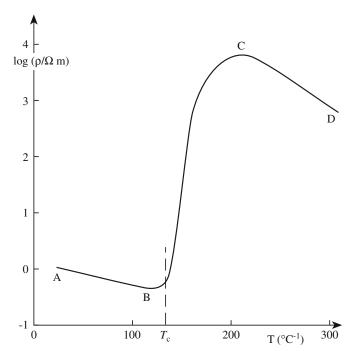
FIGURE 30.19 Typical characteristics of a PTC thermistor
