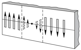
**FIGURE 31.5** Illustration of a  $180^{\circ}$  domain wall. The width is  $\sim 0.2-0.3$  nm.
