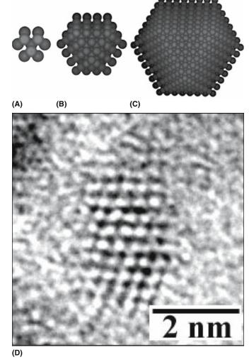
**FIGURE 13.6** Illustrating the fraction of atoms sitting at the surface of a nanoparticle. (a) Ten atoms, all on the surface; (b) 92 atoms with 74 on surfaces (80%); (c) 792 atoms with 394 on surfaces (50%). (d) An HRTEM image of a faceted nanoparticle of CdSe.
