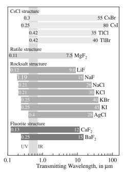
**FIGURE 6.2** Range of transmittance for halide samples grouped by structure. (Each sample is 2 mm thick; 10% cut off.) The vertical band shows the visible range.
