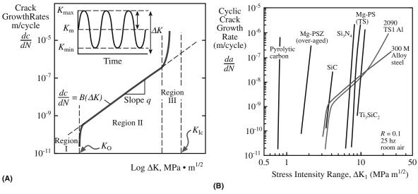
**FIGURE 18.11** (a) Log-log plot of crack growth rate versus K, which is defined in the inset. (b) Cyclic-fatigue crack growth rates for several ceramics and metal alloys as a function of applied stress intensity range,  $\Delta K$ .
