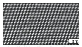
**FIGURE 6.5** HRTEM image of GaAs showing the Ga-As 0.14-nm dumbbell.
