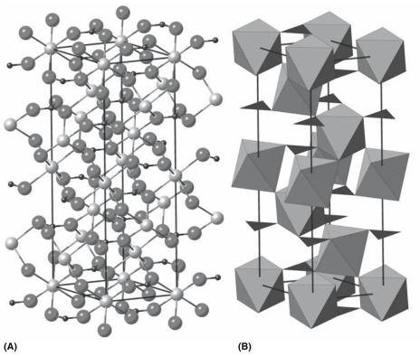
**FIGURE 7.3** The crystal structure of calcite. The  $Ca^{2+}$  cations sit in an octahedral site; the  $CO^{2-}$  ions are represented as a triangle that each links six octahedra. The octahedra have one of two orientations each and "stack" in an ApBqCr sequence giving the 3 symmetry producing the c lattice parameter of 1.71 nm (a is 0.50 nm).
