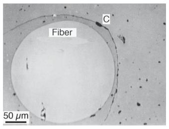
**FIGURE 18.21** SEM image showing crack propagation around a sapphikon ( $Al_2O_3$ ) fiber in a calcium aluminosilicate (CAS) glass-ceramic.
