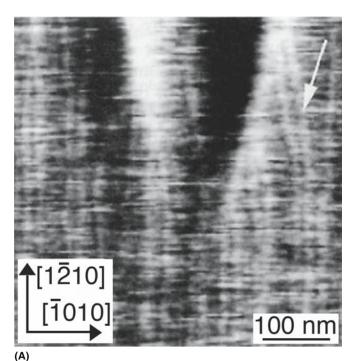
FIGURE 13.16 Sub-unit-cell surface steps on (a) sapphire and (b) spinel. The steps are 0.2nm high in each case.
