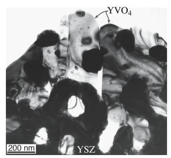
FIGURE 25.4 Corrosion of YSZ by V2O5 vapor.
