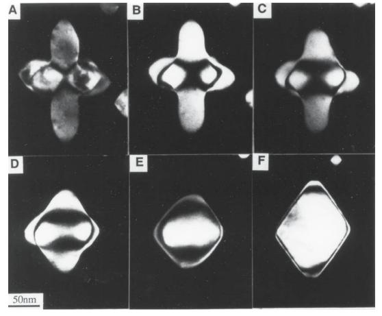
**FIGURE 15.5** Spinel particles changing shape in NiO due to heat treatment. (The image is formed as for Figure 15.4.) (A) Looking along [011]: 30-minute heat treatment between images: (B) 800°C, (C) 825°C, (D) 850°C, (E) 875°C, (F) 900°C. The shape change is summarized in the schematics (G–I). The 3D figures shows the original shape.
