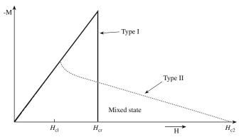
FIGURE 33.4 Magnetization behavior of Type I and Type II superconductors as a function of the applied field.
