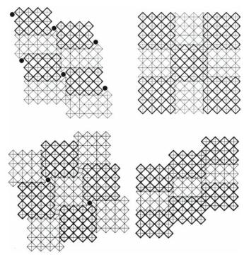
**FIGURE 14.24** Shear planes in  $WO_3$ . Dark and light lines are at heights 0 and 0.5.
