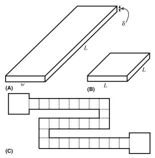
FIGURE 27.17 (a-c) Illustration of sheet resistance.
