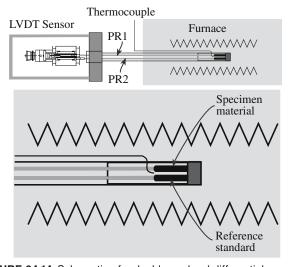
FIGURE 34.14 Schematic of a double pushrod differential dilatometer.
