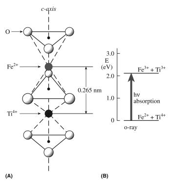
**FIGURE 36.13** (a) Illustration of the combined effect of incorporation of Ti and Fe in sapphire. The distance between the dopant cations is 0.265 nm. (b) The corresponding energy band diagram for the excitation showing how a gemstone with blue coloration is obtained by absorption.
