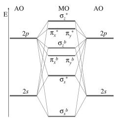
**FIGURE 4.14** Energy level diagram for homonuclear diatomic molecule where s-p hybridization has occurred.
