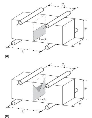
FIGURE 16.13 Geometries for (a) SENB and (b) CN specimens used to determine  $K_{lc}$ .
