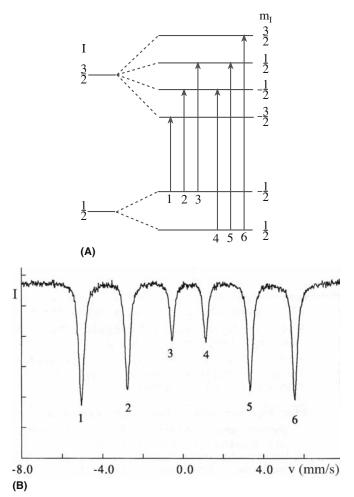
**FIGURE 10.24** Transitions in Fe and the resulting Mössbauer spectrum.
