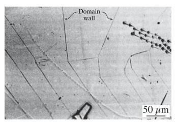
FIGURE 33.18 Magnetic domains on the basal surface of a hexagonal ferrite, Co<sub>2</sub>Ba<sub>2</sub>Fe<sub>28</sub>O<sub>46</sub>, revealed by the Bitter technique.
