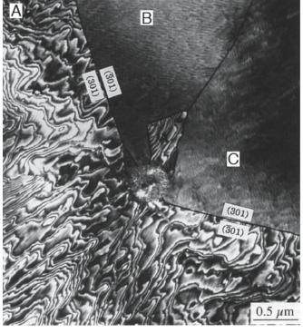
**FIGURE 14.36** Example of GBs in thin films of anorthite on  $Al_2O_3$ ; the three grains correspond to three epitactic orientations, but only one shows the misfit dislocations in this TEM image.
