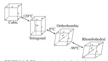
FIGURE 31.8 BaTiO<sub>3</sub> polymorphs showing direction of polarization.
