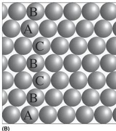
FIGURE 12.6 The intrinsic stacking fault in an fcc crystal.
