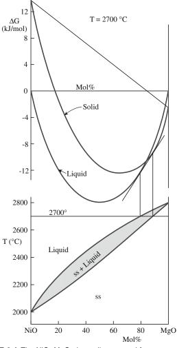
**FIGURE 8.4** The NiO–MgO phase diagram and free energy curves at T = 2700 °C.
