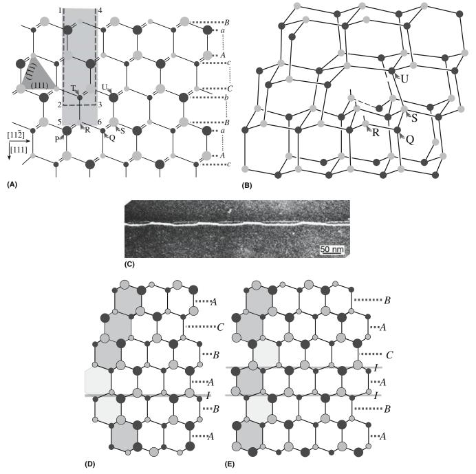
**FIGURE 12.11** Models for forming dislocations and stacking faults in sphalerite. (a) Two cuts in which to make an edge dislocation; (b) dislocation made by removing 1234; (c) two structures for a dislocation with Burgers vector **b** in Si; (d and e) intrinsic and extrnsic in Si.
