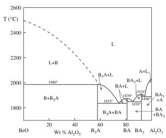
FIGURE 8.13 The BeO-Al<sub>2</sub>O<sub>3</sub> phase diagram.
