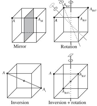
FIGURE 5.3 Symmetry elements for a simple cube.
