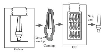
**FIGURE 23.7** Individual steps of cold preforming, canning, HIPing, and stripping in the standard HIPing process.
