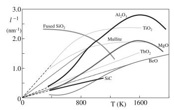
FIGURE 34.4 Inverse phonon mean free paths for several crystalline oxides and for vitreous silica.
