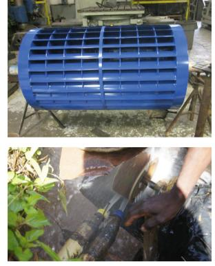
Fig. 6.27 An improvised hydroturbine in Malawi. Notice the use of plastic beverage bottles for nozzles (courtesy P. Dauenhauer)
