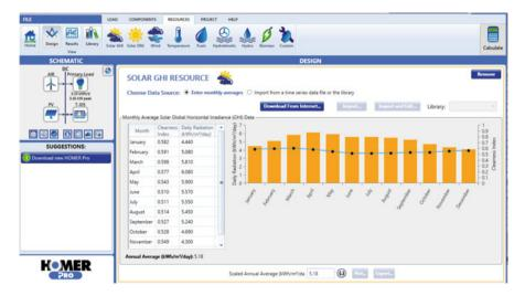
Fig. 12.7 The solar resource input screen from HOMER (courtesy of HOMER Energy)
