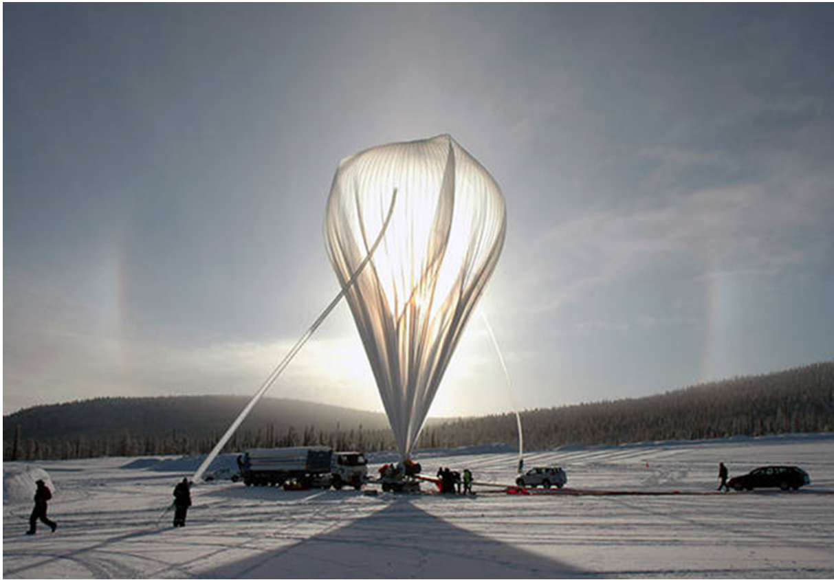
Figure 7.7 Start of a helium-filled research balloon for the investigation of the higher stratosphere. The balloon is filled only with a low He-pressure. With increasing height the external pressure decreases and the balloon inflates, increasing its volume and the buoyancy (SSC/DLR) ( http://www.eskp.de/turmhohe-forschungsballoons-messen-ozonschicht/ )
