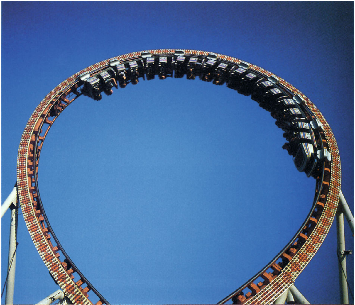
Figure 2.11 Rollercoaster, where the superposition of centripetal acceleration and gravity changes along the path and influences the feelings of the passenger (with kind permission of Foto dpa)
