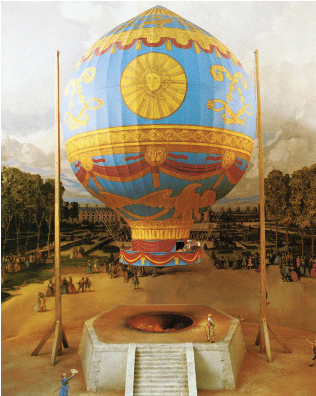
Figure 7.6 Lift of the first manned Montgolfiere. At the 21st of November 1783 the hot-air-balloon, named after its inventor Montgolfiere, started in the garden of the castle Mulette near Paris with two ballonists and landed safely after 25 min at a distance of 10 km from the starting point. The balloon was constructed with thin branches of a willow tree, that stabilized the envelope of thin fabric, covered with colorfully painted paper. The air inside the ballon was heated by a coal fire in the center of the lower opening. With kind permission of Deutsches Museum München
