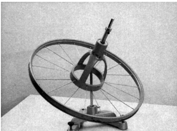
Figure 5.32 Bicycle wheel as symmetric top
