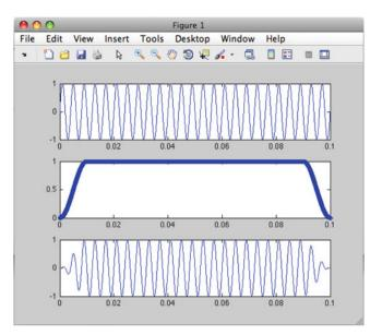
Fig. 5.2 At the *top* part of the figure you can see the original sound. At the *center* is shown the envelope that was used to modulate the sound's onset and offset. At the *bottom* of the figure is displayed the resulting modulated sound. Note that the onset and offset are not abrupt as in the *top left* graph
