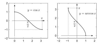
Fig. 3.12 The principal branch of the cosine (left); the arccosine function (right)
