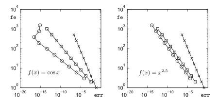
**Fig. 13.3** Accuracy-cost-diagram of the Gaussian quadrature formulas. The crosses are the results of the one-stage Gaussian method of order 2, the squares the ones of the two-stage method of order 4 and the circles the ones of the three-stage method of order 6
