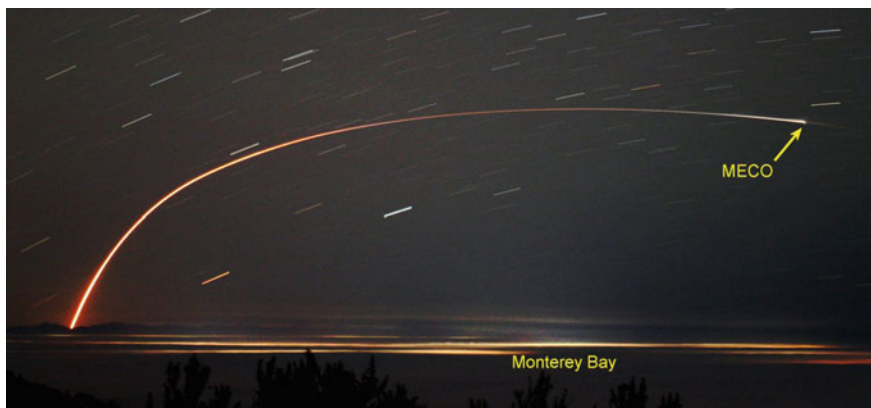
Fig. 6.11 Ascent trajectory with gravity turn until main engines cut-off (MECO) of an ascending Delta II rocket from Vandenberg Air Force Base on July 2, 2014. Credit Rick Baldrige
