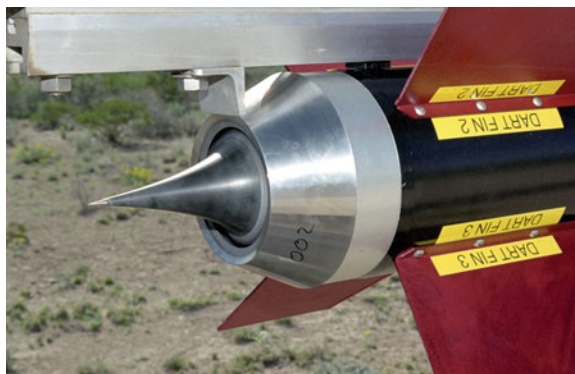
Fig. 4.12 A spike nozzle having a plug at the center as used in NASA's Dryden Aerospike Rocket Test in March 2004. Credit NASA
