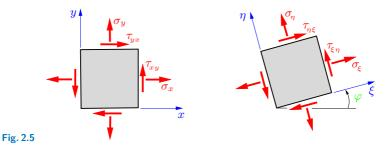
A quantity whose components have *two* coordinate subscripts and which are transformed by a certain rule from one coordinate system to a rotated coordinate system is called a *second rank ten*-
