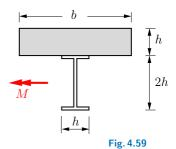
Given: M = 2000 kNm,  $E_{\text{Con}} = 3.5 \cdot 10^4 \text{ MPa},$   $E_{\text{St}} = 2.1 \cdot 10^5 \text{ MPa},$  h = 500 mm, $A_{\text{St}} = h^2/6, I_{\text{St}} = h^4/18.$
