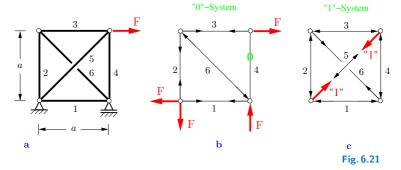
**Solution** The truss consists of m=6 members and j=4 joints; it has r=3 supports. According to Volume 1, Section 6.1, it is statically indeterminate to the first degree: m+r-2j=1. We obtain a statically determinate truss if we remove one of the bars.
