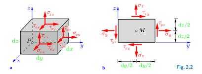
The notation can be simplified for the normal stresses. In this case the directions of the normal to the section and of the stress component coincide. Thus, both subscripts are always equal and one of them can be omitted without losing information:
