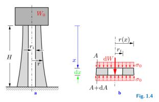
**Solution** We consider the tower to be a slender bar. The relationship between stress, normal force and cross-sectional area is given by (1.4). In this example the constant compressive stress  $\sigma = \sigma_0$  is given; the normal force (here counted positive as compressive force) and the area A are unknown.
