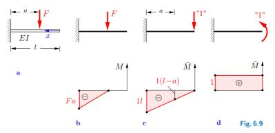
To illustrate the method we consider the cantilever beam subjected to a force F as depicted in Fig. 6.9a. We will calculate the deflection and the angle of slope at the free end. If we use the coordinate x shown in Fig. 6.9a, the bending moment caused by the given force F is (Fig. 6.9b)
