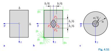
As a second example consider a circular cross section with radius a (Fig. 4.51c). With  $r_{gy}^2 = a^2/4$ ,  $z_0 = a$  and with symmetry considerations the core is obtained to be an inner circle of radius a/4.
