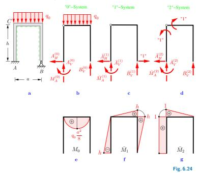
**Solution** The frame has five support reactions (clamping and hinged support). Therefore it is statically indeterminate to the second degree. In order to obtain a statically determinate "0"-system, we replace the hinged support B with a roller support (which can move in the horizontal direction) and we introduce a hinge at the corner C.
