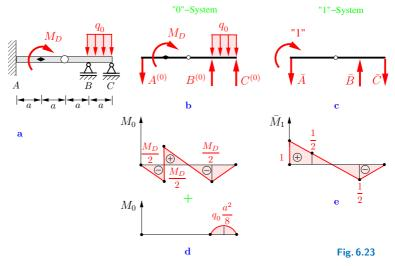
**Solution** The beam is statically indeterminate to the first degree (see Volume 1, Section 5.3.3). To obtain a statically determinate "0"-system, we remove the clamping and replace it with a hinged support. The equilibrium conditions yield the support reactions (Fig. 6.23b)
