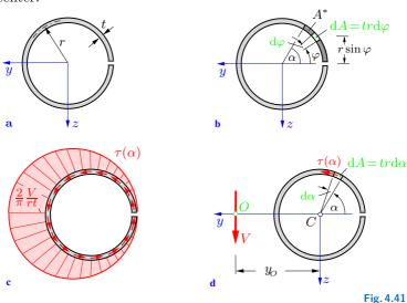
**Solution** The shear stresses follow from (4.39). The first moment of the area  $A^*$  is obtained as (see Fig. 4.41b)
