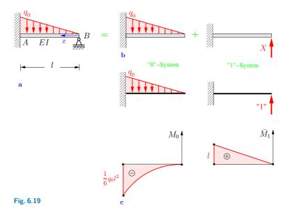
to (6.44) the redundant support reaction X is obtained from
