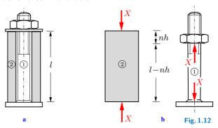
**Solution** After the nut has been turned it exerts a compressive force X on the tube which causes a shortening of the tube. According to Newton's third axiom (action = reaction) a force of equal magnitude and opposite direction acts via the nut on the bolt which elongates. The free-body diagrams of bolt and tube are shown in Fig. 1.12b.
