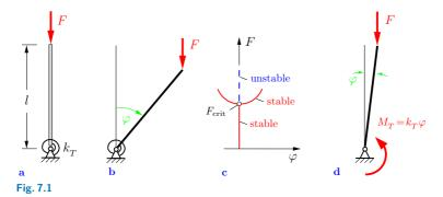
In order to determine the equilibrium positions and to analyse their stability we use the total potential of the system. Choosing the zero-level of the potential of F at the height of the pin support, the potential of the system, rotated about  $\varphi$  (Fig. 7.1b), is given by
