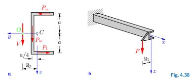
force are in equilibrium with the applied loads and a torque is not caused by the loads.
