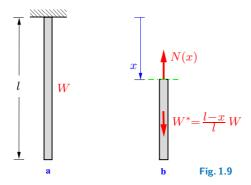
As an illustrative example of a statically determinate system let us consider a slender bar (weight W, cross-sectional area A) that is suspended from the ceiling (Fig. 1.9a). First we determine the normal force caused by the weight of the bar. We cut the bar at an arbitrary position x (Fig. 1.9b). The normal force N is equal to the weight  $W^*$  of the portion of the bar below the imaginary cut. Thus, it is given by  $N(x) = W^*(x) = W(l-x)/l$ . Equation (1.4) now yields the normal stress
