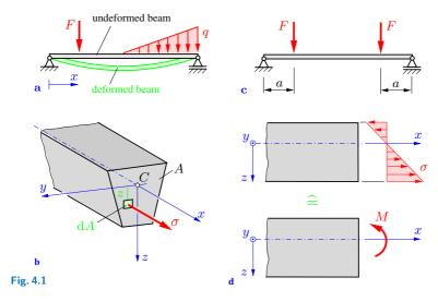
Let us consider the beam in Fig. 4.1b where the z-axis is an axis of symmetry. In accordance with Volume 1, the x-axis coincides with the axis of the beam and passes through the centroid C of the cross-sectional area A. The reason for this particular choice of the location of the x-axis will become apparent in Section 4.3. The z-axis points downward and the orientation of the y-axis is chosen in such a way that the axes x, y and z represent a right-hand system.
