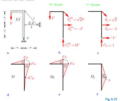
**Solution** The structure is statically indeterminate to the first degree. To obtain a "0"-system we replace the hinged support at C with a roller support which can move in the horizontal direction. The equilibrium conditions in the "0"-system (Fig. 6.22b) yield
