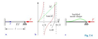
The four constants of integration can be determined from the boundary conditions: two conditions at each boundary. In order to illustrate the procedure, let us consider a statically indeterminate bar as depicted in Fig. 7.4a. From (7.14) we obtain
