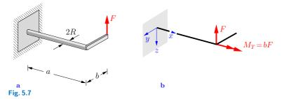
**Solution** The force F at the free end of the lever is statically equivalent to a force F and a moment  $M_T = b F$  at the end of the straight circular shaft (Fig. 5.7b). The shaft is subjected to
