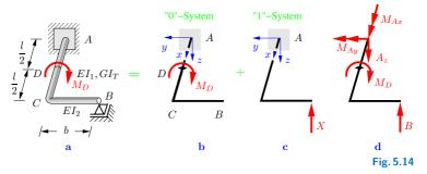
**Solution** The frame has one degree of static indeterminacy. We first determine one support reaction with the method of superposition. If we remove the support at B, we obtain the "0"-system depicted in Fig. 5.14b. As a result of the loading  $M_D$  the cross section at C exhibits the same rotation as the cross section at D. Using equation (5.7), we obtain
