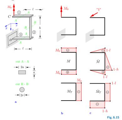
**Solution** The parts 1 and 3 are subjected to bending; part 2 is subjected to torsion. One can see by inspection that point C undergoes a displacement v in the y-direction.
