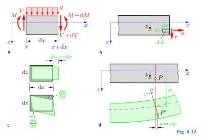
i.e., we assume that the axes y and z are the principal axes of the cross sectional area ( $I_{yz}=0$ ). In addition, the applied loads are assumed to cause only a shear force V in the z-direction and a bending moment M about the y-axis. These assumptions are satisfied, for example, if the z-axis is an axis of symmetry of the cross section and the applied forces act in the x, z-plane.
