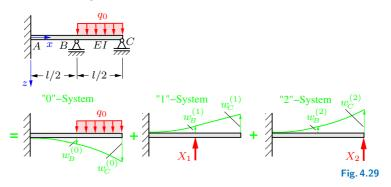
at B and C in the original system, the compatibility conditions are
