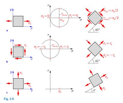
circle in this case coincides with the origin of the coordinate system (Fig. 2.9b). The principal stresses are  $\sigma_1 = \tau_0$  and  $\sigma_2 = -\tau_0$ ; they act in sections at 45° with respect to the x-axis.
