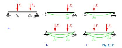
If we first apply  $F_i$  and subsequently  $F_k$  (Fig. 6.17c), the total work is
