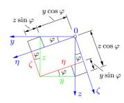
$\cos^2\varphi=\frac{1}{2}(1+\cos2\varphi)$  and  $2\sin\varphi\cos\varphi=\sin2\varphi$  we obtain the transformation equations
