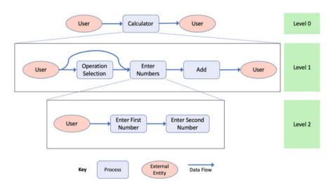
In this diagram the hierarchy of DFDs is indicated by the levels which expand on how the function in the previous level is implemented by the functions at the next level. This DFD also only presents the data flow for the situation where the user selects the add function as the numerical operation to apply.
