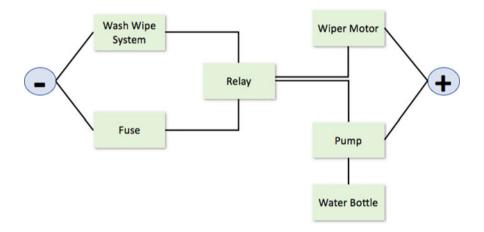
This system aims to provide a diagnosis tutor for the equipment illustrated above. Rather than use the wash-wipe system from a real car, students on a car mechanics diagnosis course use this software simulation. The software system mimics the actual system, so the behaviour of the pump depends on information provided by the relay and the water bottle.
